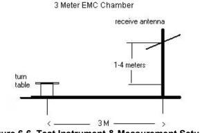
Figure 6-6. Test Instrument & Measurement Setup
