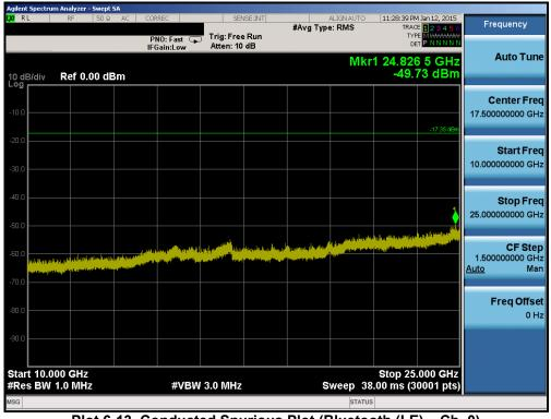
Plot 6-13. Conducted Spurious Plot (Bluetooth (LE) – Ch. 0)
