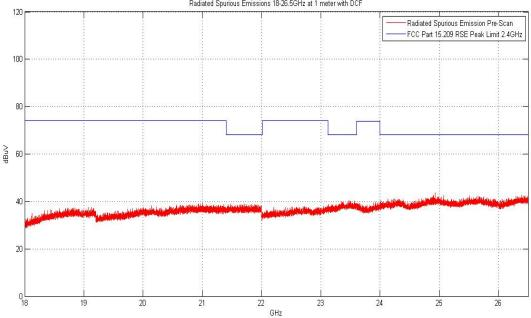
Radiated Spurious Emissions 18-26.5GHz at 1 meter with DCF
