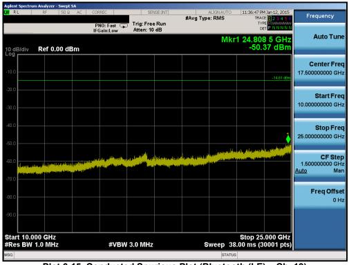
Plot 6-15. Conducted Spurious Plot (Bluetooth (LE) – Ch. 19)
