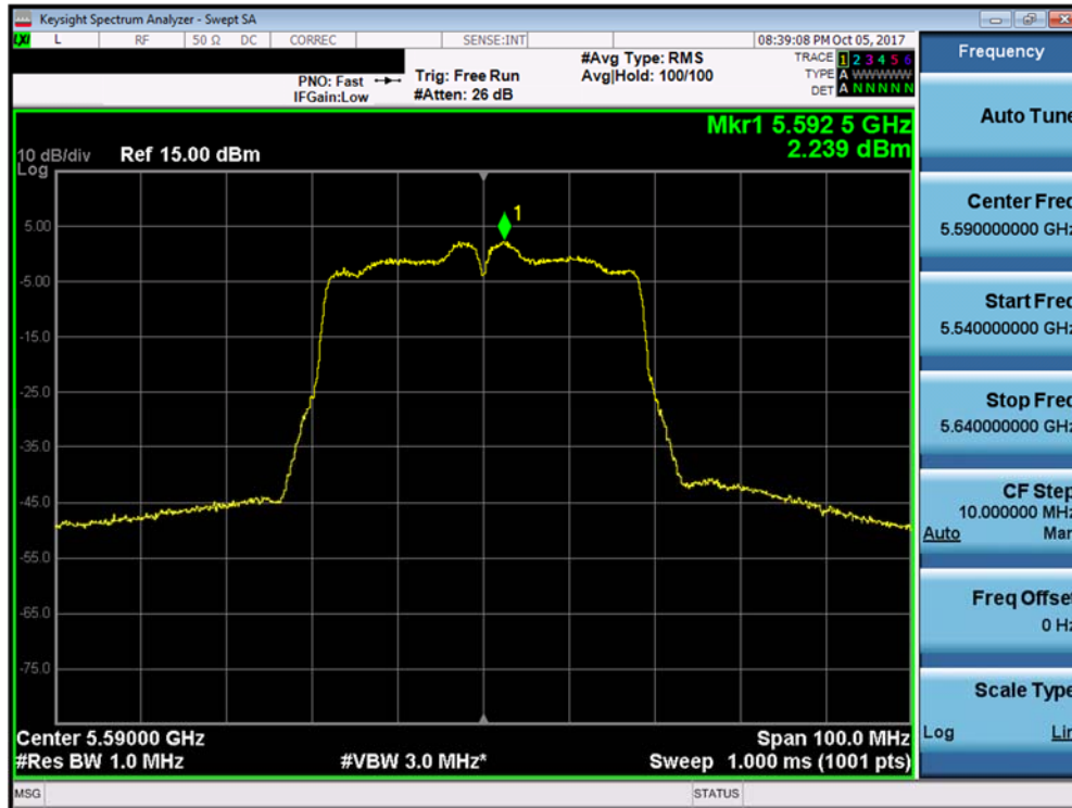
Plot 7-11. Power Spectral Density Plot (40MHz BW 802.11n (UNII Band 2C) – Ch. 118)
