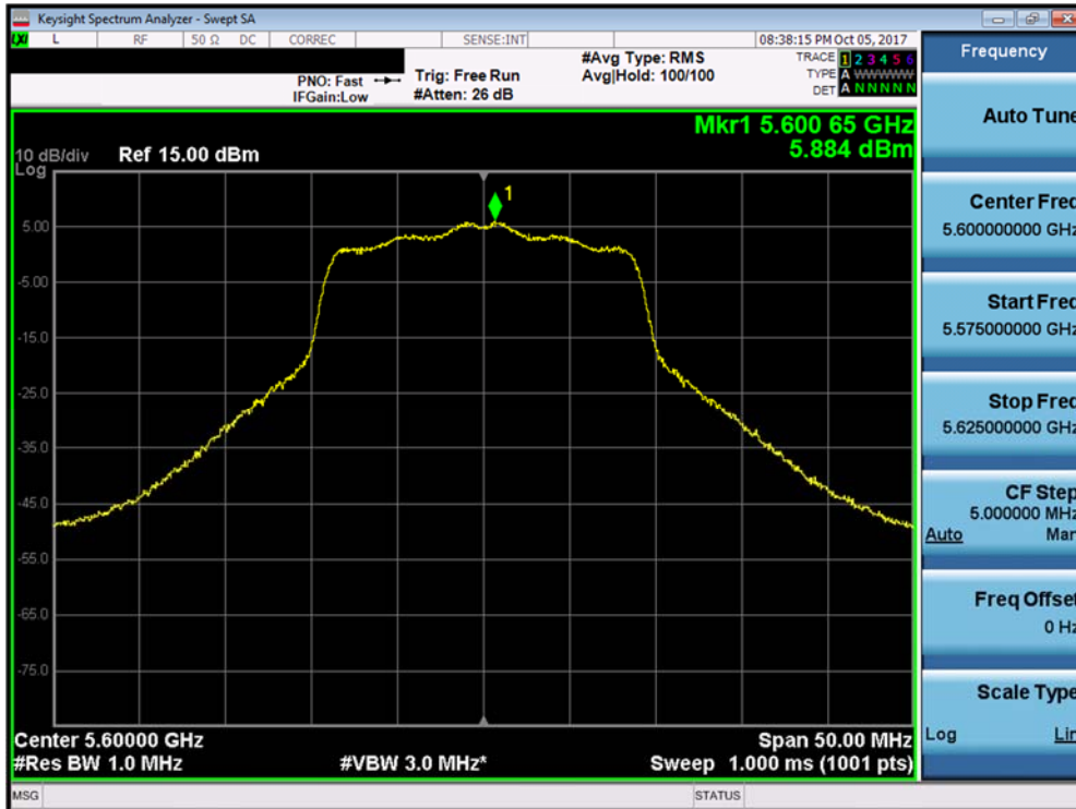
Plot 7-10. Power Spectral Density Plot (20MHz BW 802.11n (UNII Band 2C) – Ch. 120)
