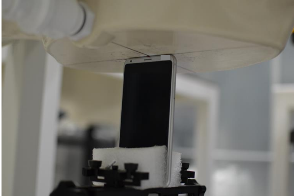
SAR Test Setup Photo 11: Top at 0.0 cm
