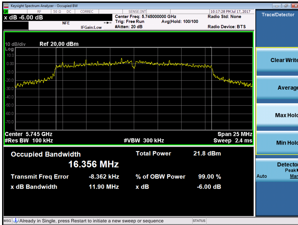
Plot 7-68. 6dB Bandwidth Plot (802.11a (UNII Band 3) – Ch. 149)
