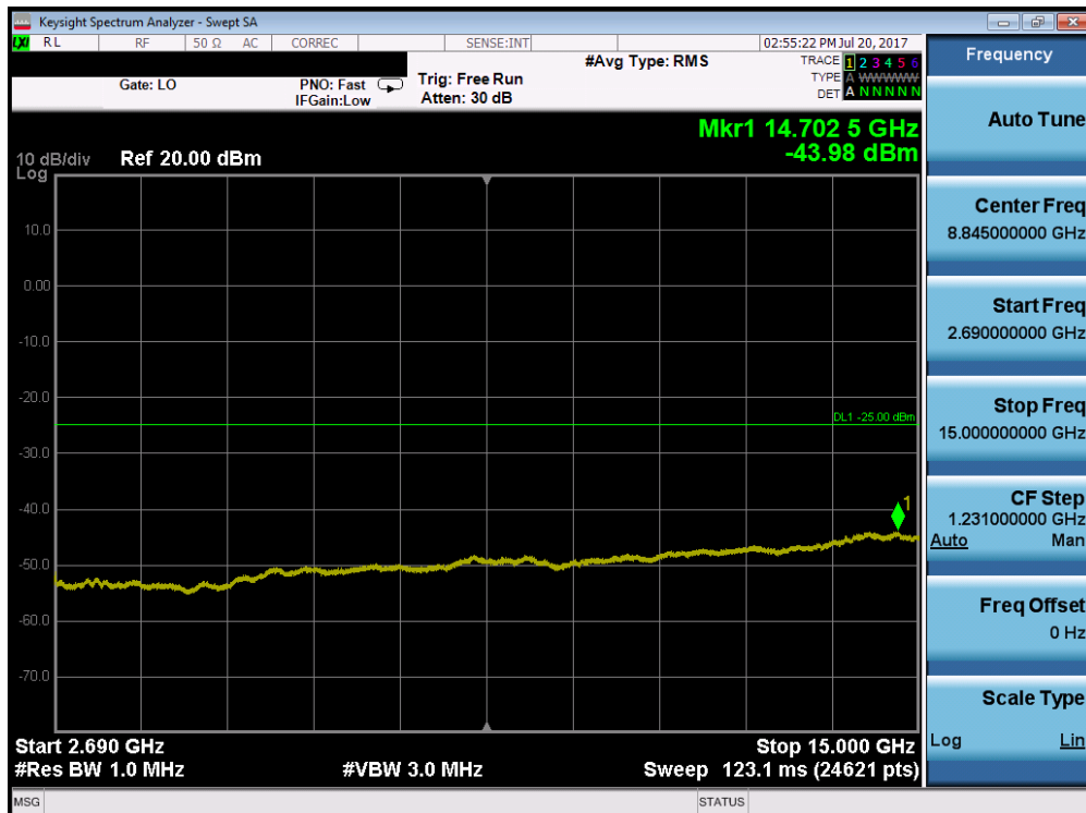
Plot 7-134. Conducted Spurious Plot (Band 41 – 20.0MHz QPSK – RB Size 1, RB Offset 0 – Mid Channel)
