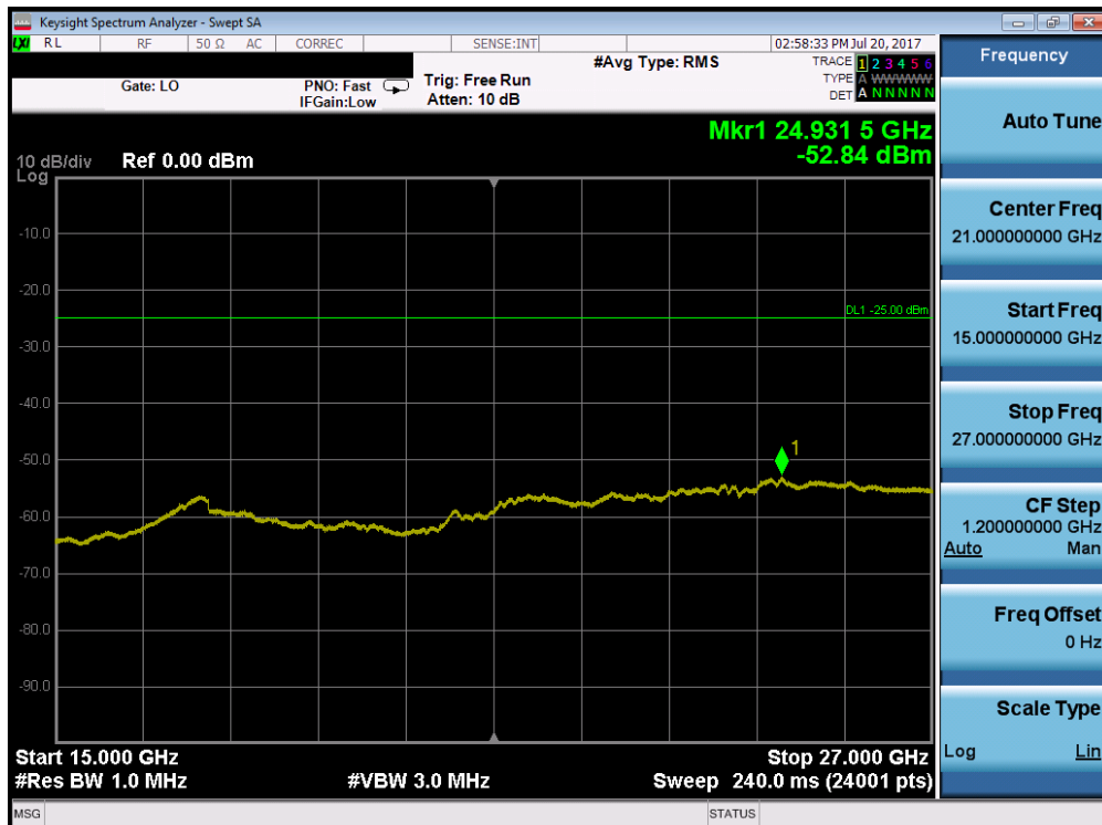
Plot 7-132. Conducted Spurious Plot (Band 41 – 20.0MHz QPSK – RB Size 1, RB Offset 0 – Low Channel)
