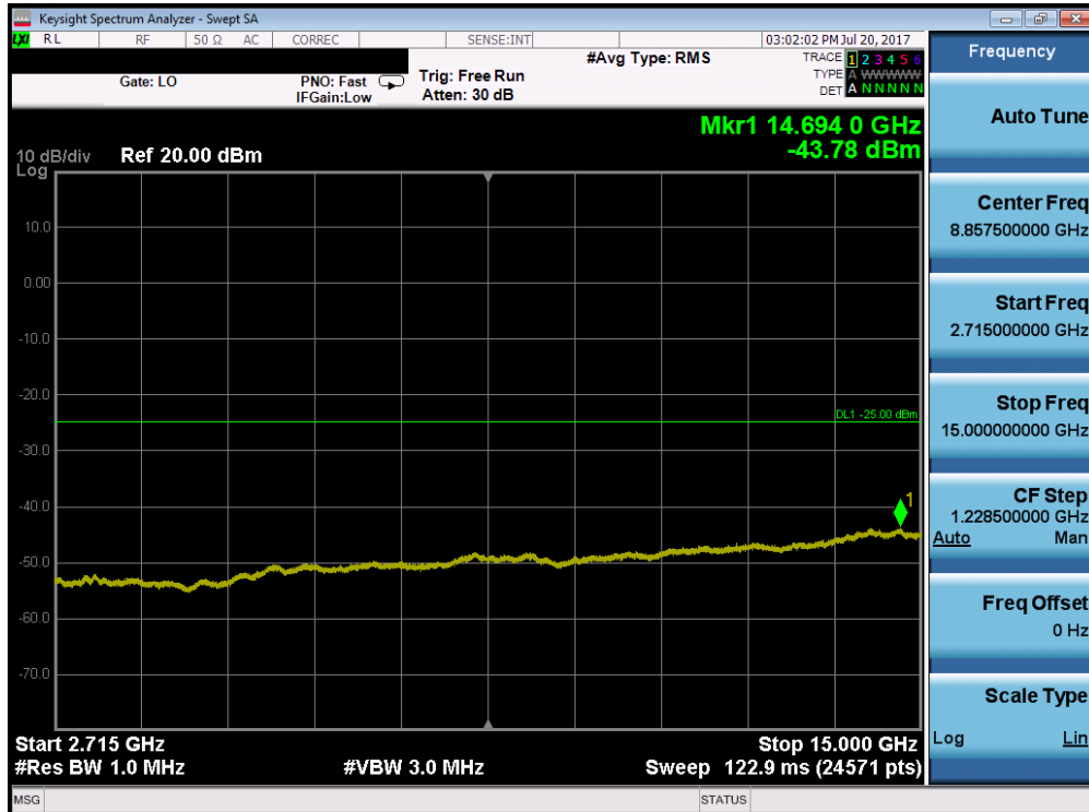
Plot 7-137. Conducted Spurious Plot (Band 41 – 20.0MHz QPSK – RB Size 1, RB Offset 0 – High Channel)
