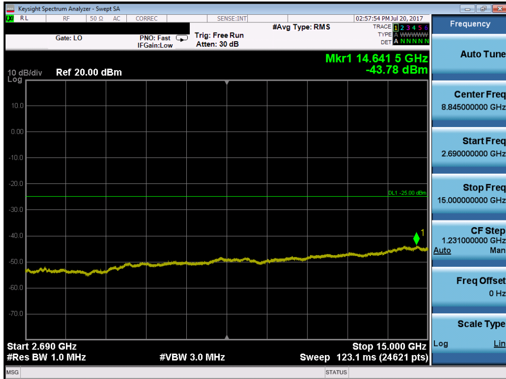
Plot 7-131. Conducted Spurious Plot (Band 41 – 20.0MHz QPSK – RB Size 1, RB Offset 0 – Low Channel)
