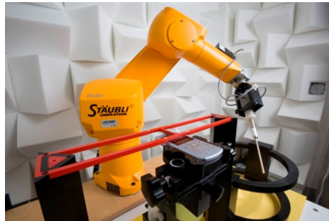
Figure 4-3 SPEAG Robotic System
