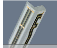
Figure 4-1 E-field Free-space Probe
