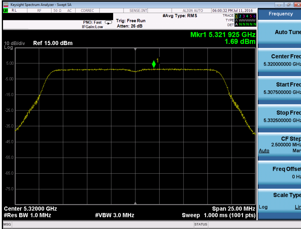
Plot 7-129. Power Spectral Density Plot (20MHz BW 802.11n (UNII Band 2A) – Ch. 64)
