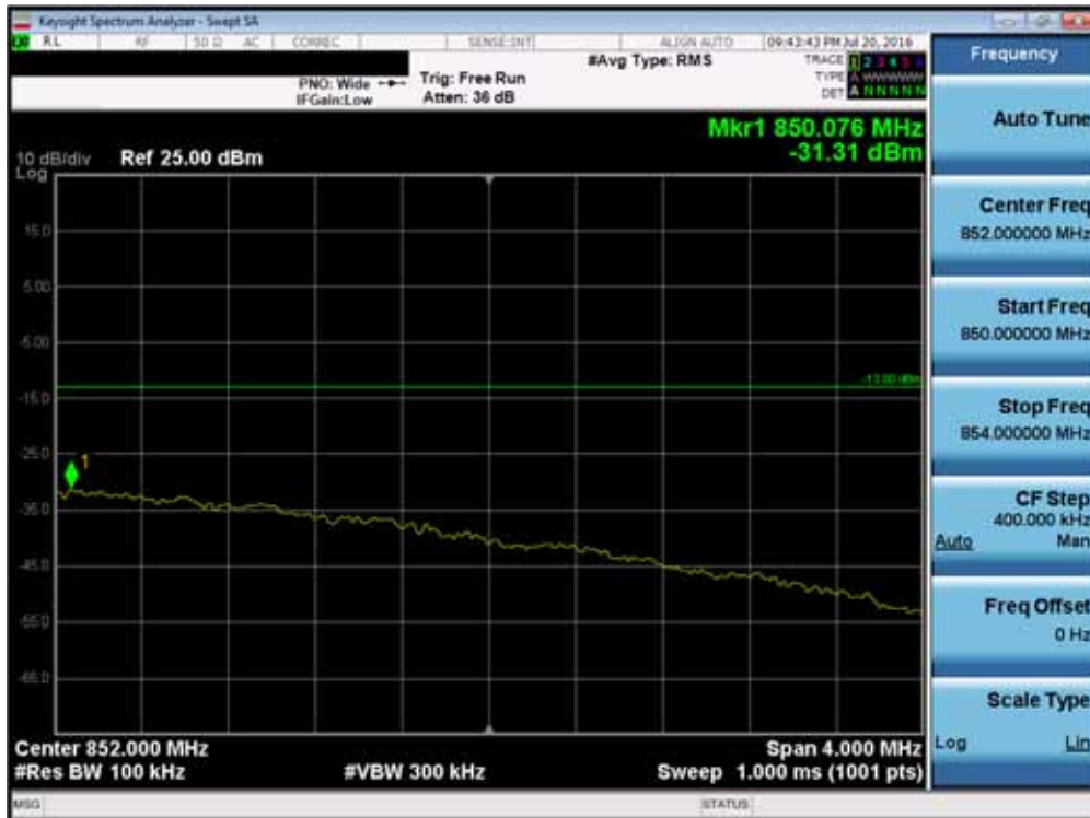
Plot 7-115. Upper Extended Band Edge Plot (Band 5 – Band 5 – 3.0MHz QPSK – RB Size 15)
