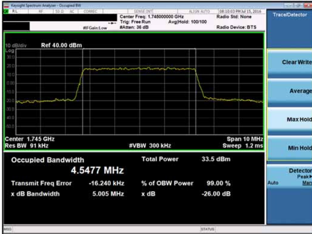
Plot 7-25. Occupied Bandwidth Plot (Band 4/66– 5.0MHz QPSK – RB Size 25)
