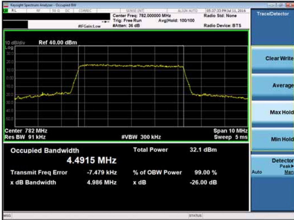
Plot 7-9. Occupied Bandwidth Plot (Band 13 – 5.0MHz QPSK – RB Size 25)
