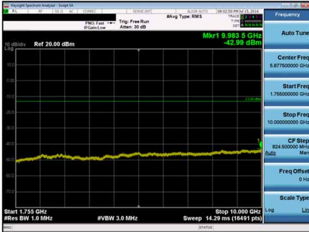
Plot 7-67. Conducted Spurious Plot (Band 4/66– 10.0MHz QPSK – RB Size 1, RB Offset 0 – Low Channel)
