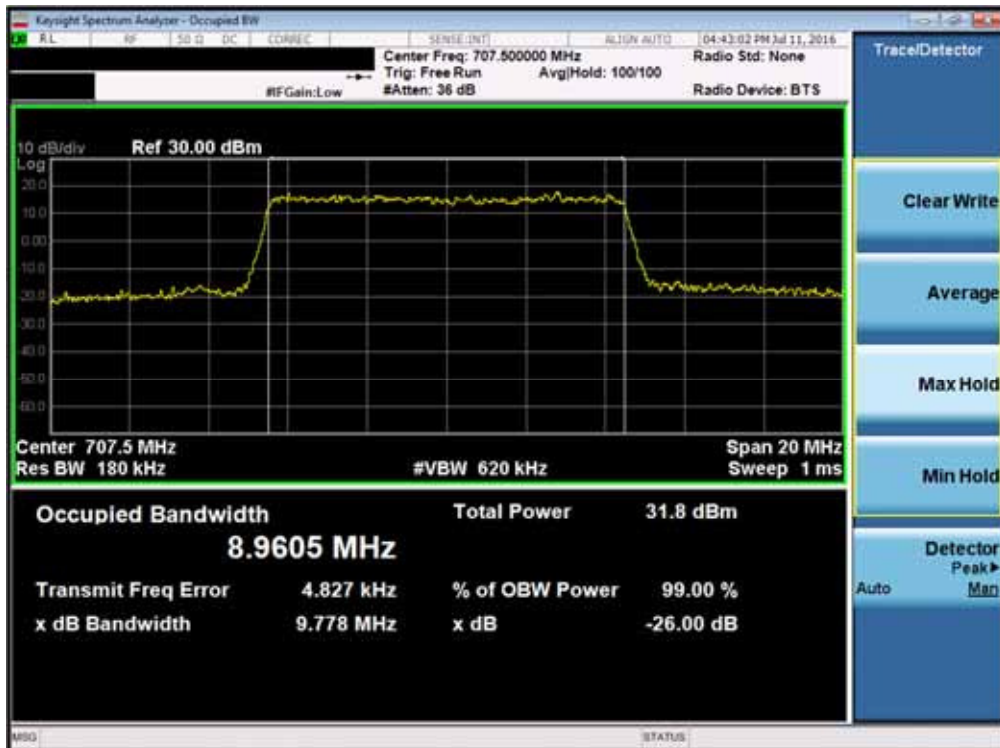
Plot 7-8. Occupied Bandwidth Plot (Band 12 – 10.0MHz 16-QAM – RB Size 50)
