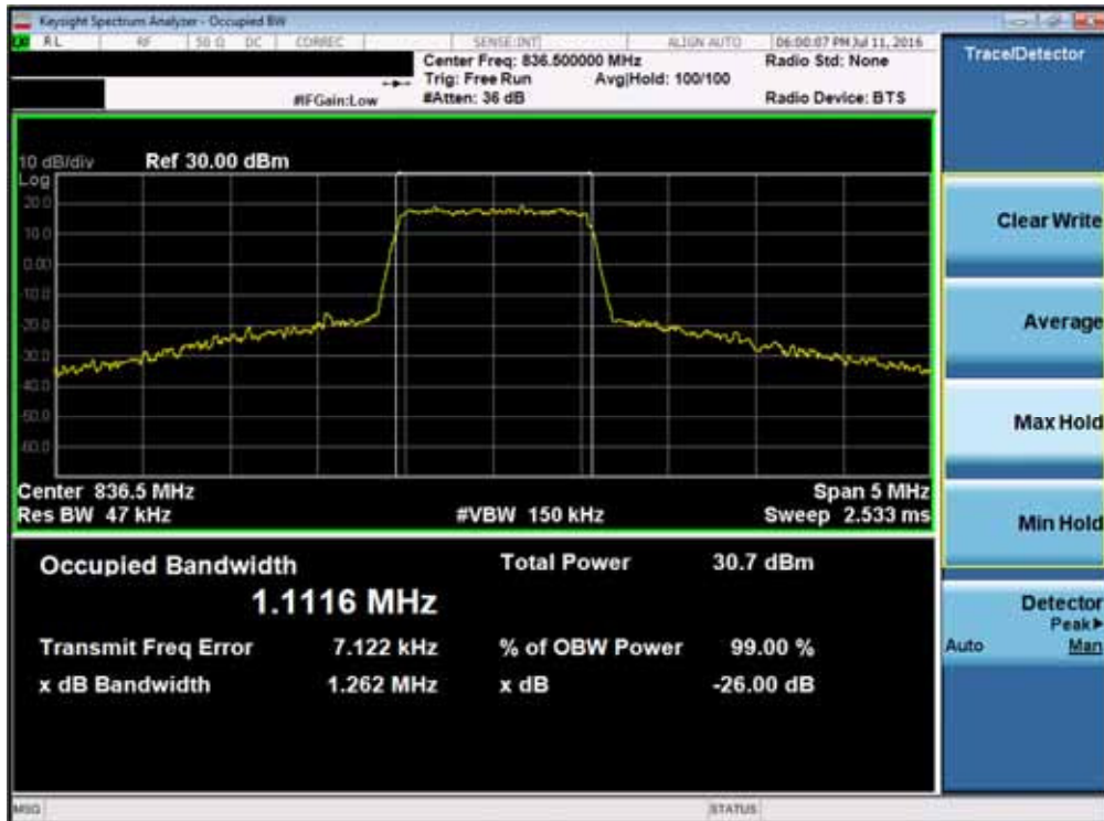
Plot 7-14. Occupied Bandwidth Plot (Band 5 – 1.4MHz 16-QAM – RB Size 6)
