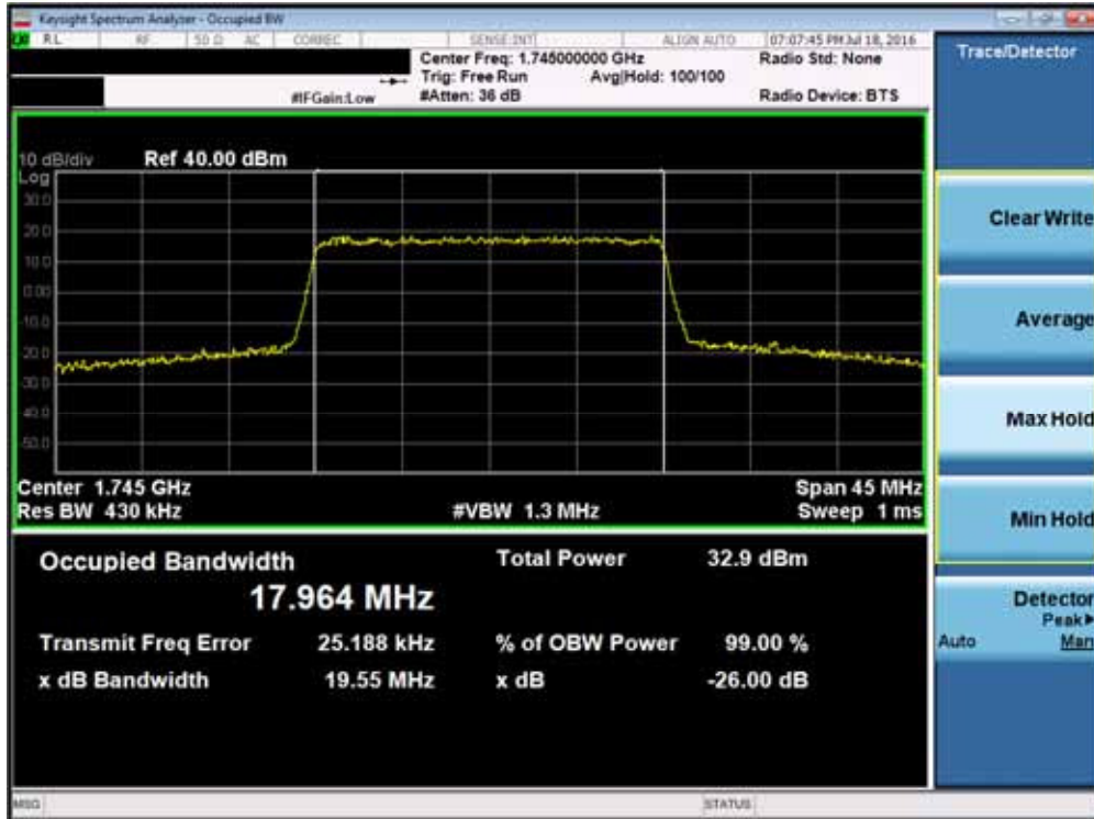
Plot 7-31. Occupied Bandwidth Plot (Band 4/66– 20.0MHz QPSK – RB Size 100)
