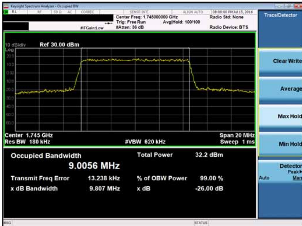
Plot 7-28. Occupied Bandwidth Plot (Band 4/66– 10.0MHz 16-QAM – RB Size 50)
