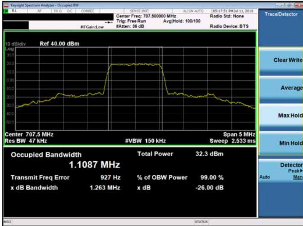
Plot 7-1. Occupied Bandwidth Plot (Band 12 – 1.4MHz QPSK – RB Size 6)
