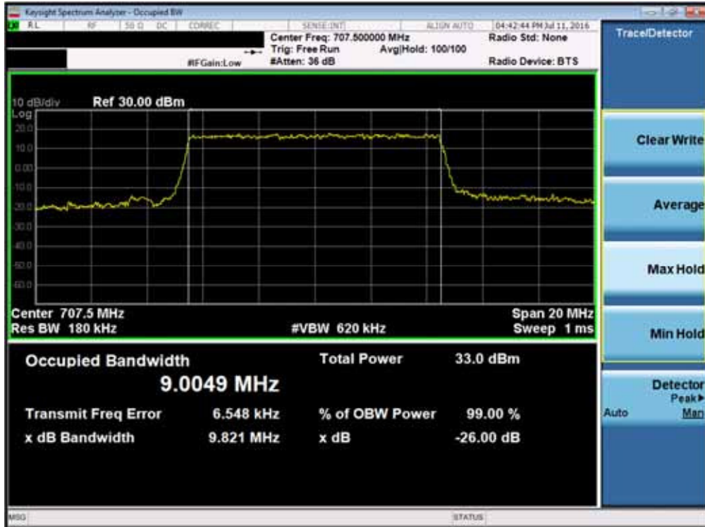
Plot 7-7. Occupied Bandwidth Plot (Band 12 – 10.0MHz QPSK – RB Size 50)
