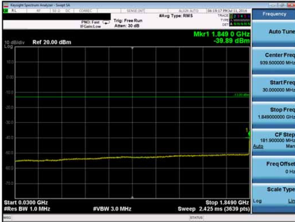
Plot 7-75. Conducted Spurious Plot (Band 2 – 20.0MHz QPSK – RB Size 1, RB Offset 0– Low Channel)
