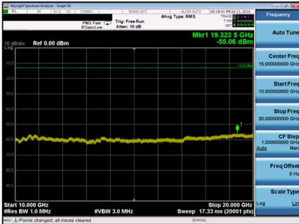
Plot 7-80. Conducted Spurious Plot (Band 2 – 20.0MHz QPSK – RB Size 1, RB Offset 0 – Mid Channel)
