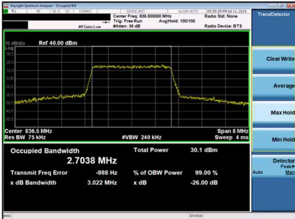
Plot 7-16. Occupied Bandwidth Plot (Band 5 – 3.0MHz 16-QAM – RB Size 15)
