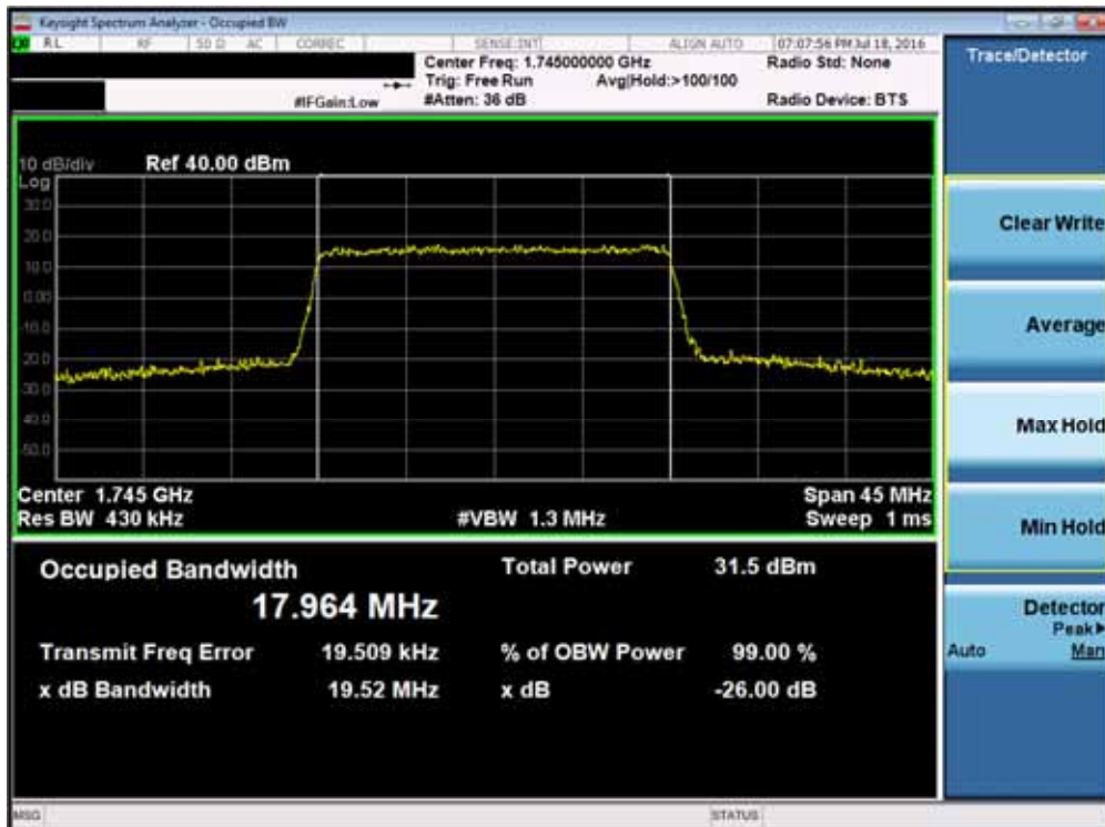
Plot 7-32. Occupied Bandwidth Plot (Band 4/66– 20.0MHz 16-QAM – RB Size 100)
