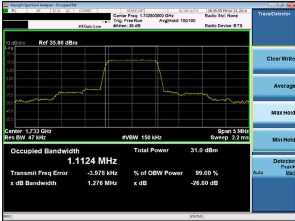
Plot 7-21. Occupied Bandwidth Plot (Band 4 – 1.4MHz QPSK – RB Size 6)
