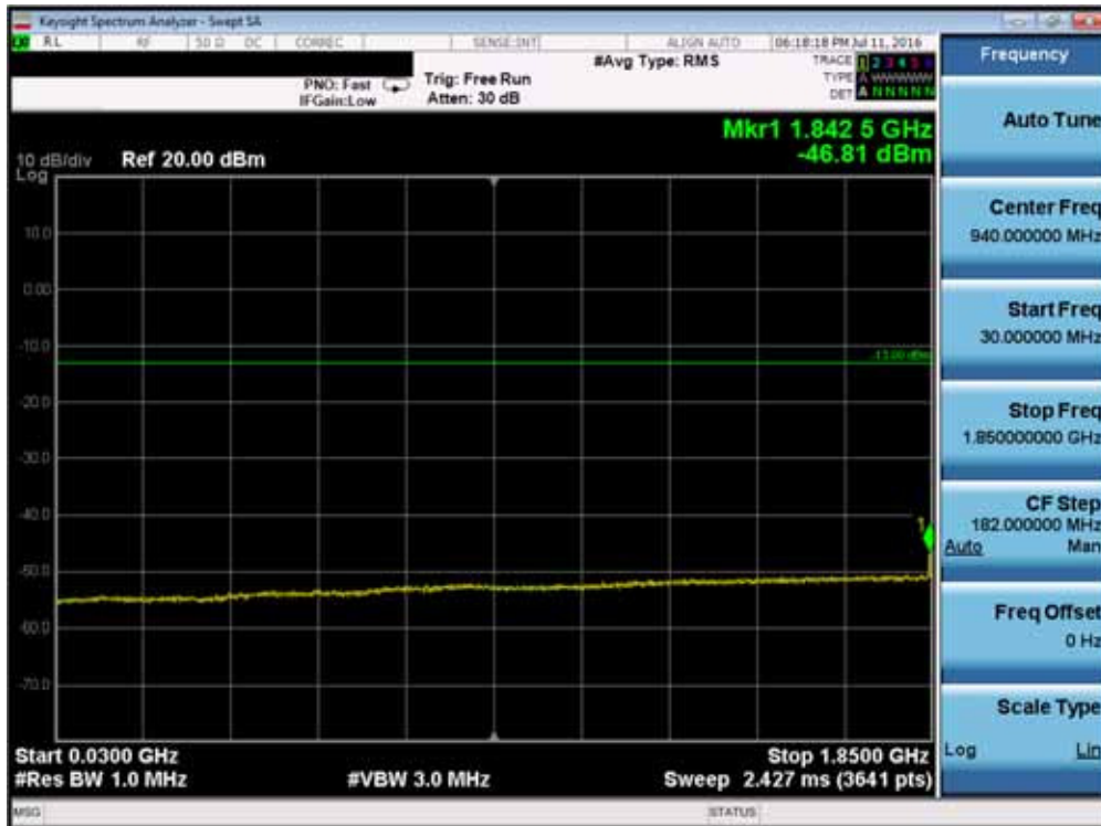
Plot 7-78. Conducted Spurious Plot (Band 2 – 20.0MHz QPSK – RB Size 1, RB Offset 0 – Mid Channel)
