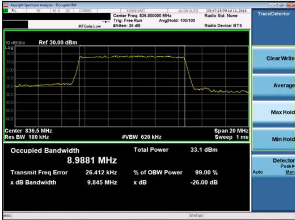
Plot 7-19. Occupied Bandwidth Plot (Band 5 – 10.0MHz QPSK – RB Size 50)
