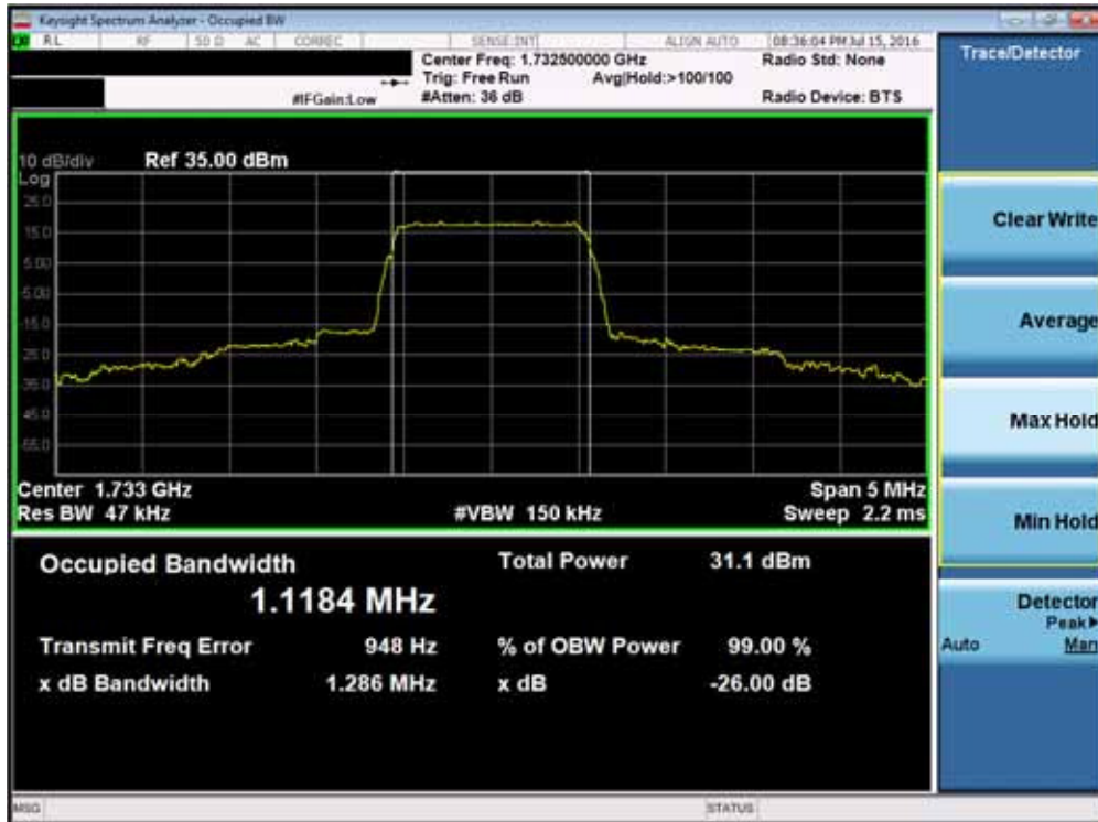
Plot 7-22. Occupied Bandwidth Plot (Band 4 – 1.4MHz 16-QAM – RB Size 6)
