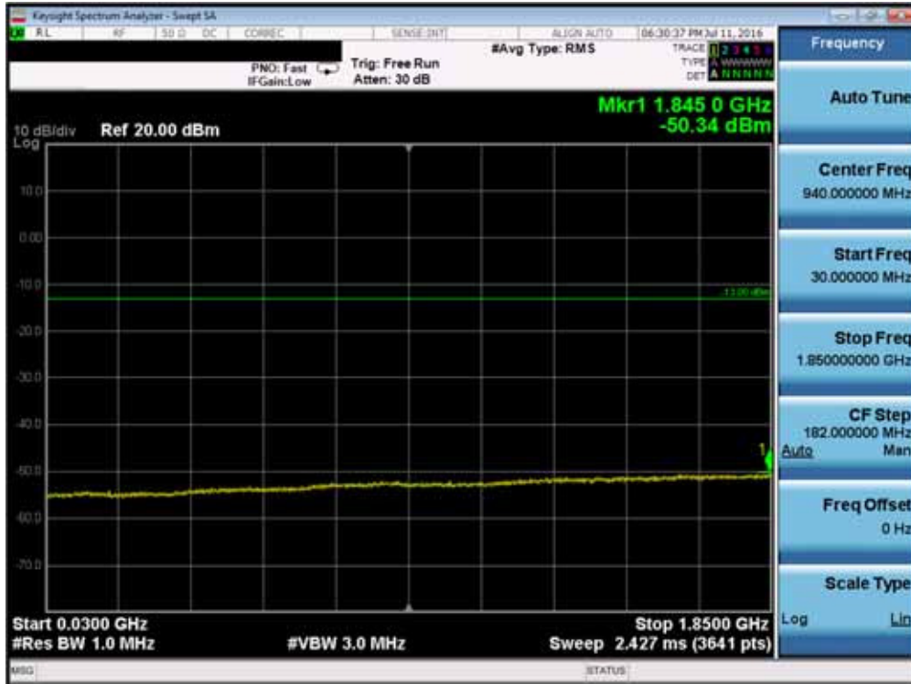
Plot 7-81. Conducted Spurious Plot (Band 2 – 20.0MHz QPSK – RB Size 1, RB Offset 0 – High Channel)
