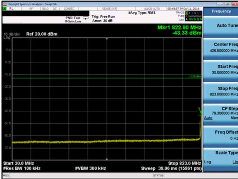
Plot 7-57. Conducted Spurious Plot (Band 5 – 10.0MHz QPSK – RB Size 1, RB Offset 0– Low Channel)
