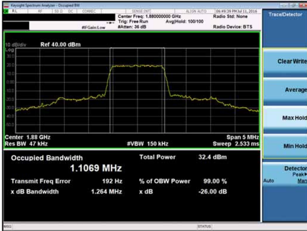
Plot 7-33. Occupied Bandwidth Plot (Band 2 – 1.4MHz QPSK – RB Size 6)
