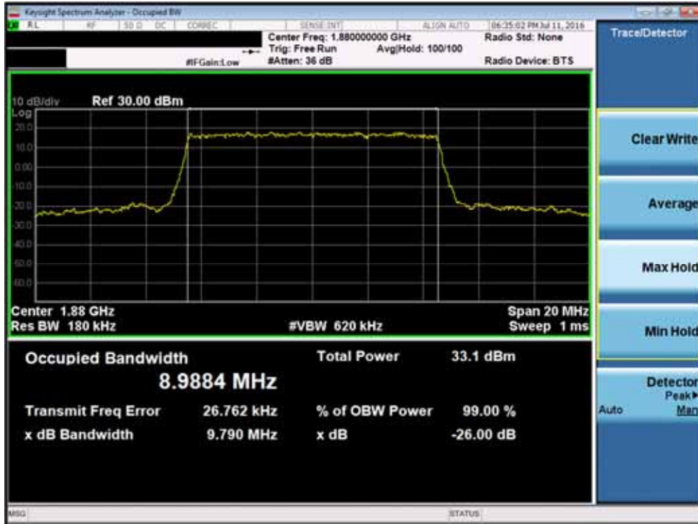
Plot 7-39. Occupied Bandwidth Plot (Band 2 – 10.0MHz QPSK – RB Size 50)
