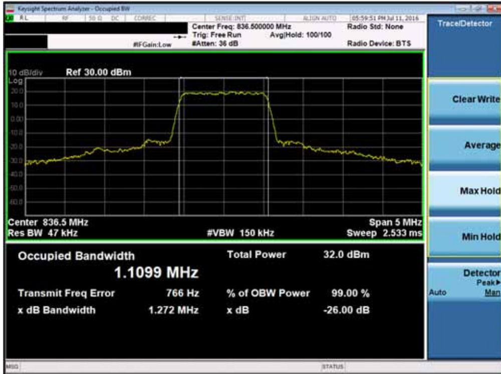
Plot 7-13. Occupied Bandwidth Plot (Band 5 – 1.4MHz QPSK – RB Size 6)
