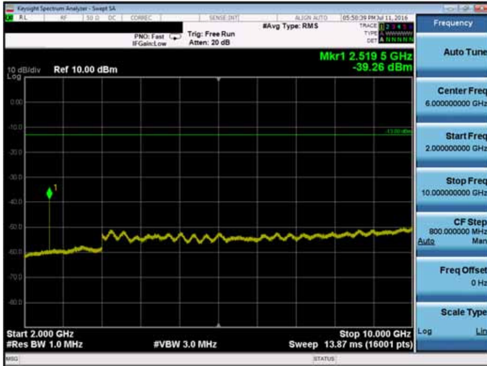
Plot 7-65. Conducted Spurious Plot (Band 5 – 10.0MHz QPSK – RB Size 1, RB Offset 0 – High Channel)
