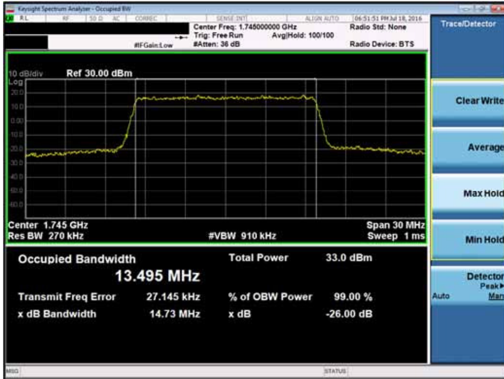
Plot 7-29. Occupied Bandwidth Plot (Band 4/66– 15.0MHz QPSK – RB Size 75)
