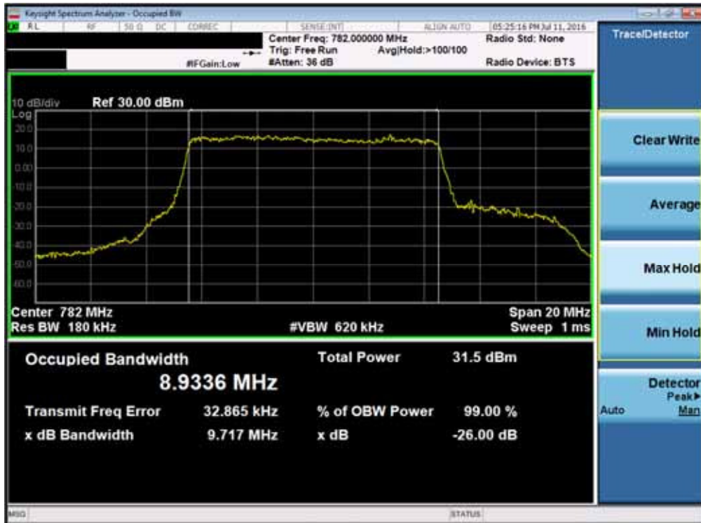
Plot 7-12. Occupied Bandwidth Plot (Band 13 – 10.0MHz 16-QAM – RB Size 50)
