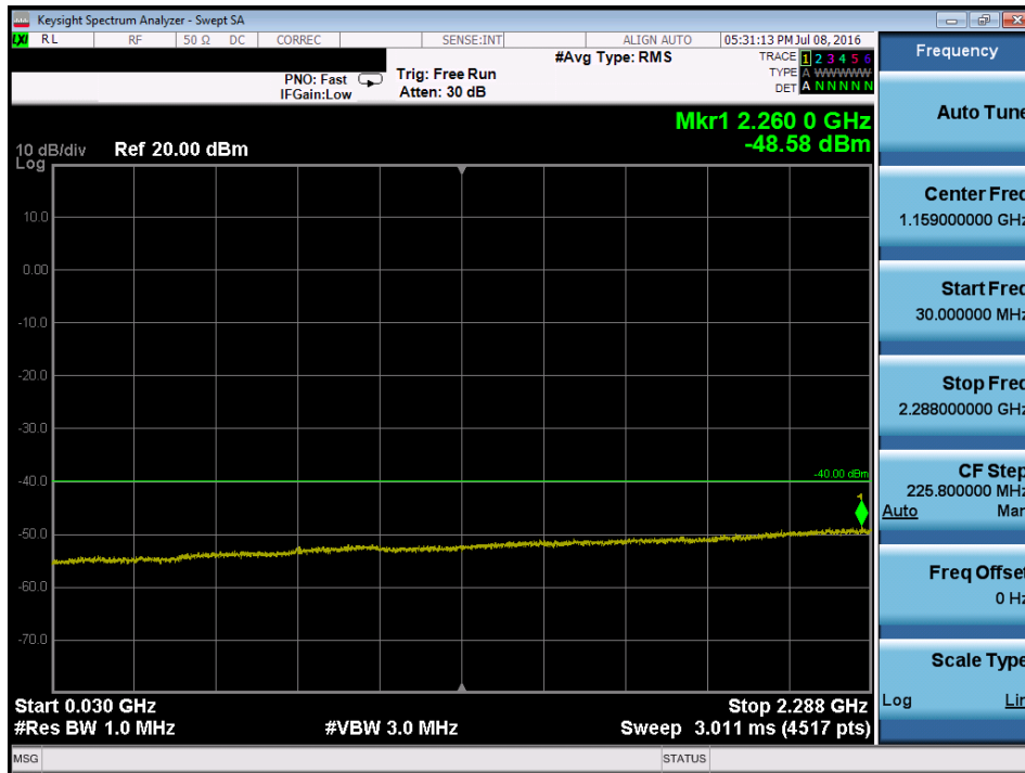
Plot 7-92. Conducted Spurious Plot (Band 30 – 5.0MHz QPSK – RB Size 1, RB Offset 0 – Mid Channel)
