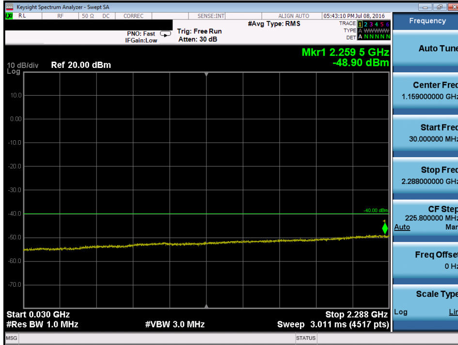
Plot 7-89. Conducted Spurious Plot (Band 30 – 5.0MHz QPSK – RB Size 1, RB Offset 0 – Low Channel)
