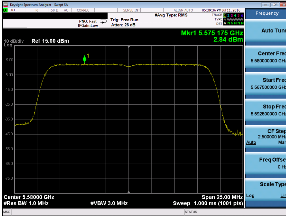
Plot 7-99. Power Spectral Density Plot (20MHz BW 802.11n (UNII Band 2C) – Ch. 116)
