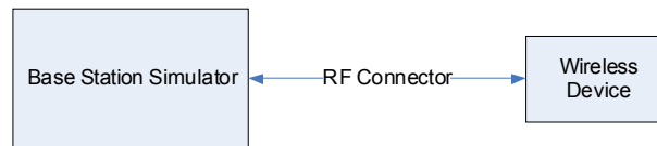
Figure 9-2 Power Measurement Setup
