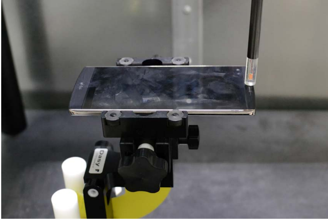
Figure 13-1 Test Setup for Wireless Device
