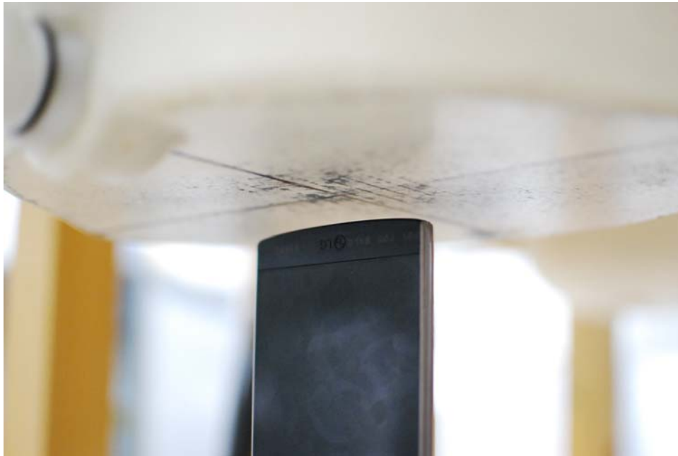
SAR Test Setup Photo 16: Bottom Edge, Standard Cover at 10 mm
