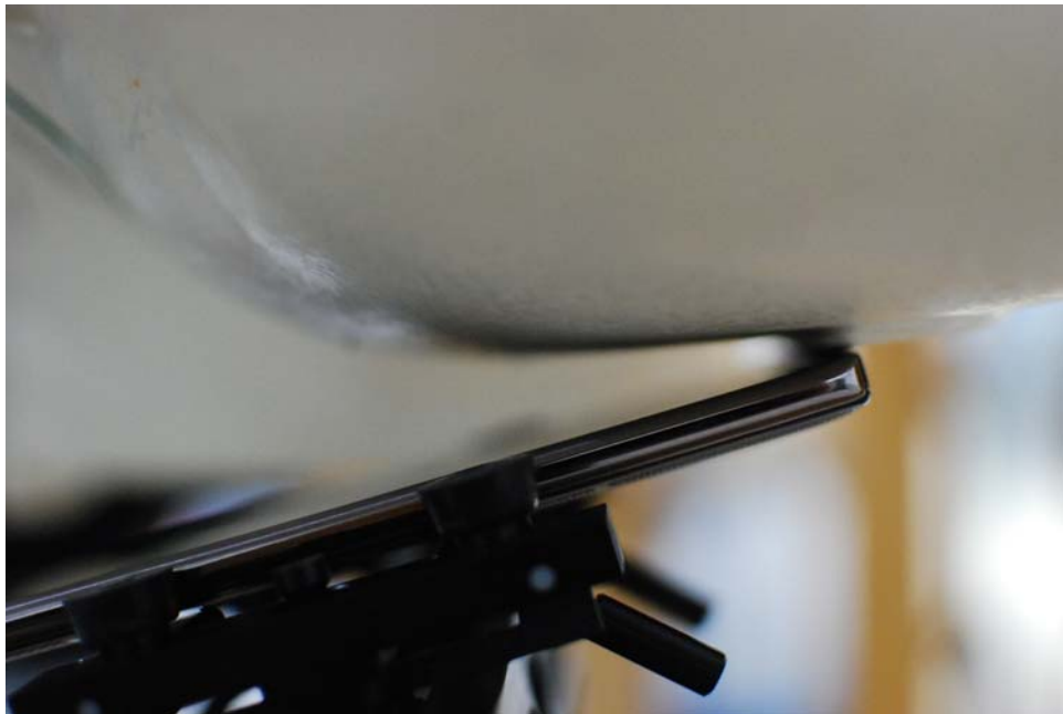
SAR Test Setup Photo 6: Left Tilt, Standard Cover
