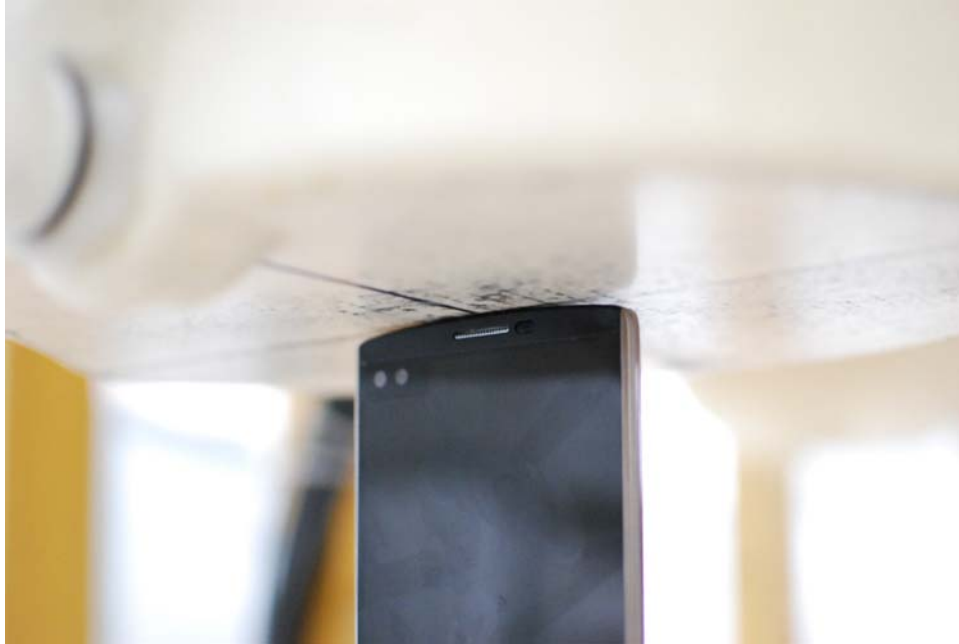
SAR Test Setup Photo 15: Top Edge, Standard Cover at 0 mm
