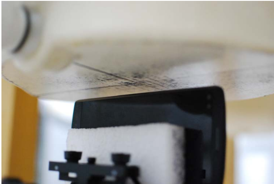
SAR Test Setup Photo 20: Left Edge, Standard Cover at 10 mm
