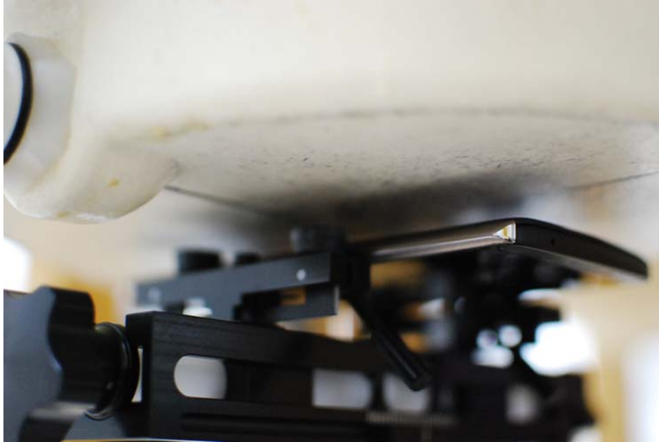
SAR Test Setup Photo 7: Back Side, Standard Cover at 10 mm
