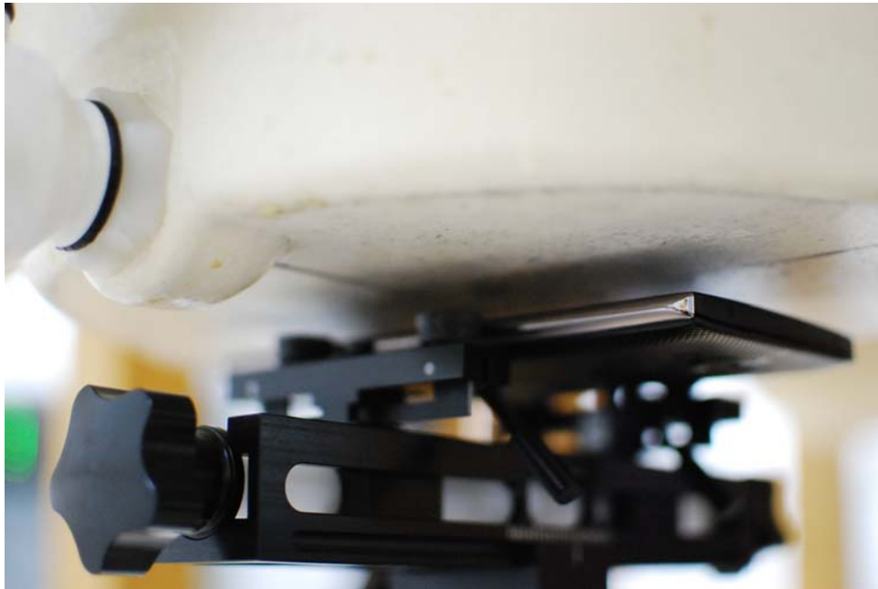
SAR Test Setup Photo 12: Front Side, Wireless Charging Cover at 10 mm
