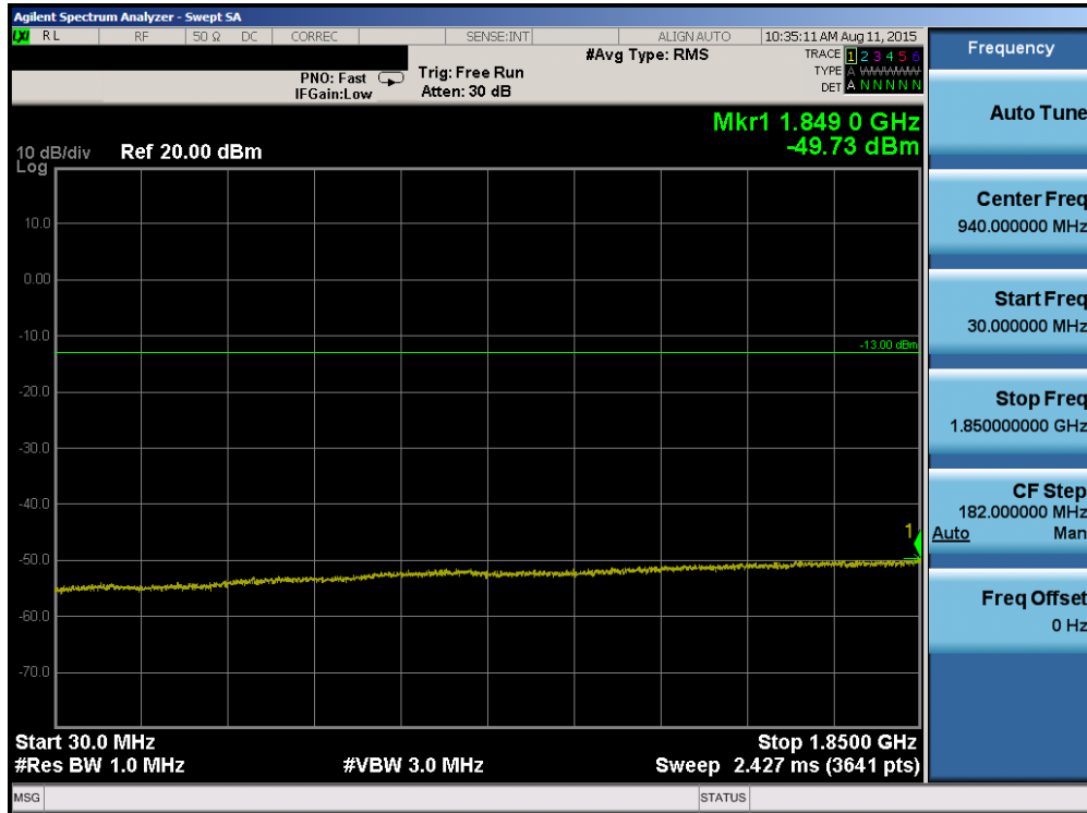
Plot 6-75. Conducted Spurious Plot (Band 2 – 20.0MHz QPSK – RB Size 1, RB Offset 0 – High Channel)
