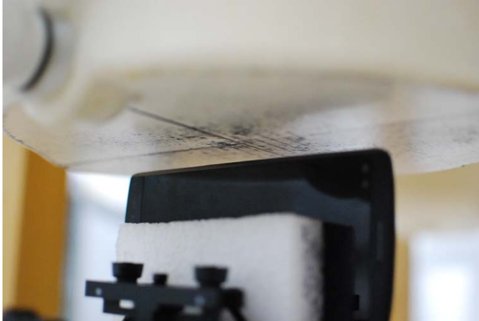
SAR Test Setup Photo 21: Left Edge, Wireless Charging Cover at 10 mm
