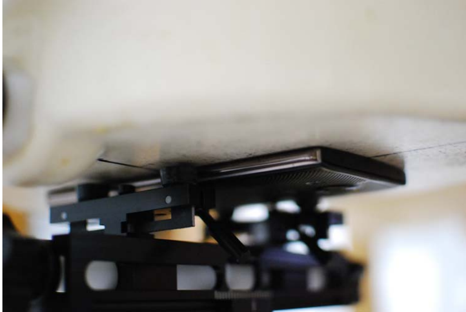
SAR Test Setup Photo 13: Front Side, Standard Cover at 0 mm
