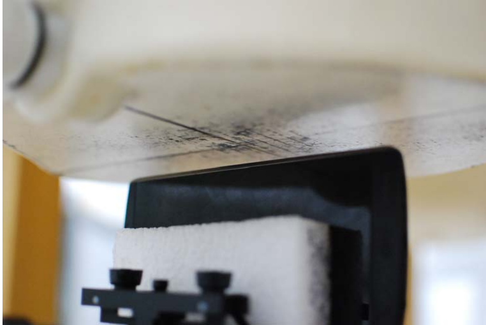
SAR Test Setup Photo 19: Right Edge, Wireless Charging Cover at 10 mm
