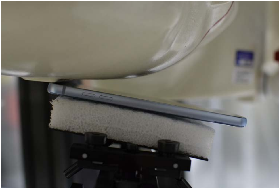
SAR Test Setup Photo 2: Right Tilt
