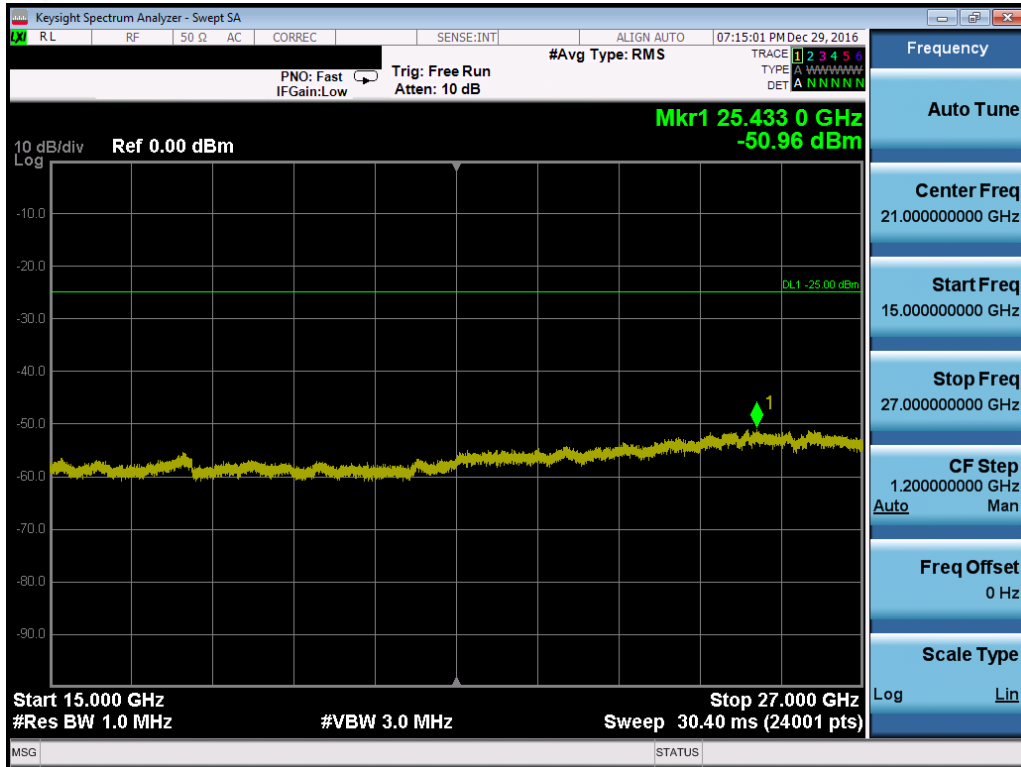
Plot 7-130. Conducted Spurious Plot (Band 7 – 20.0MHz QPSK – RB Size 1, RB Offset 0 – Low Channel)
