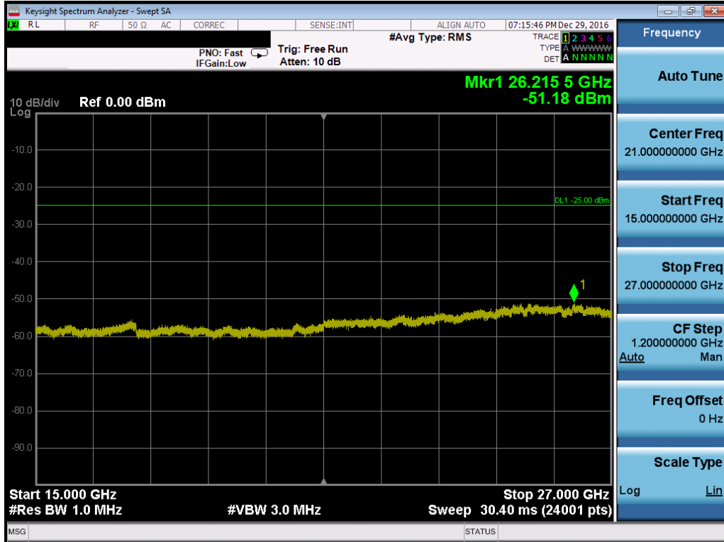
Plot 7-136. Conducted Spurious Plot (Band 7 – 20.0MHz QPSK – RB Size 1, RB Offset 0 – High Channel)
