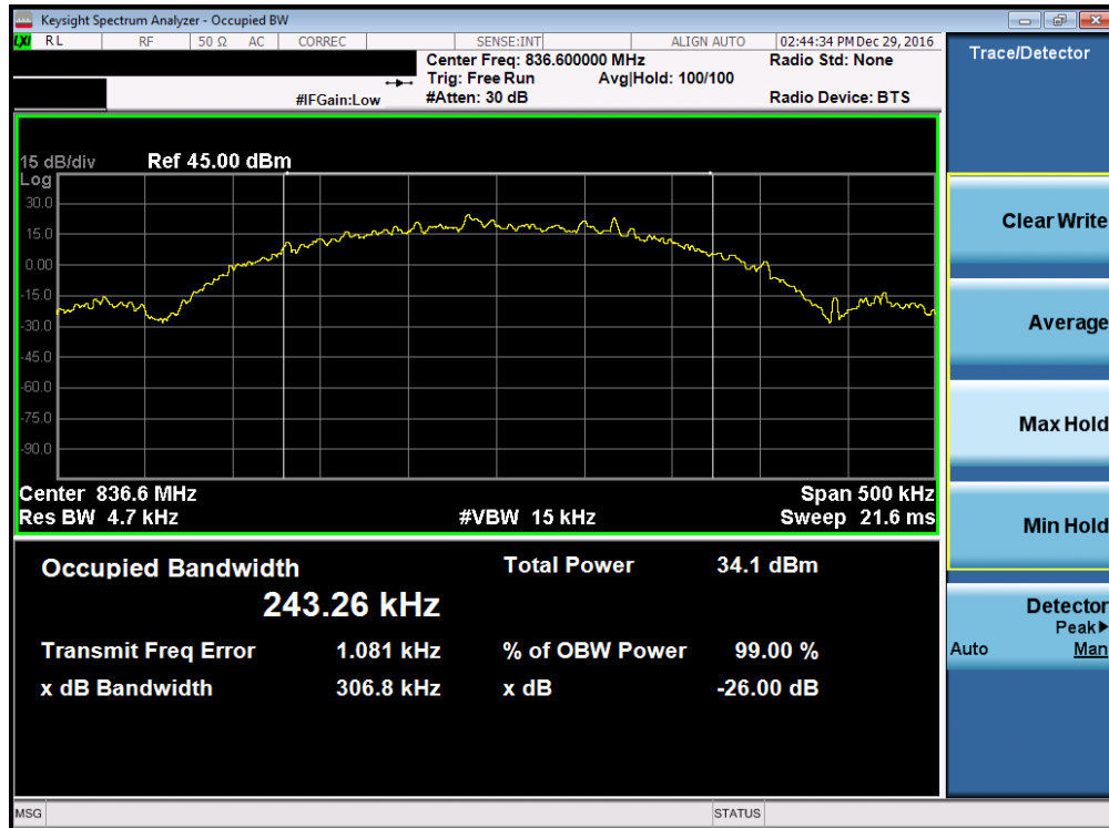
Plot 7-2. Occupied Bandwidth Plot (EDGE850 Mode – Ch. 190)
