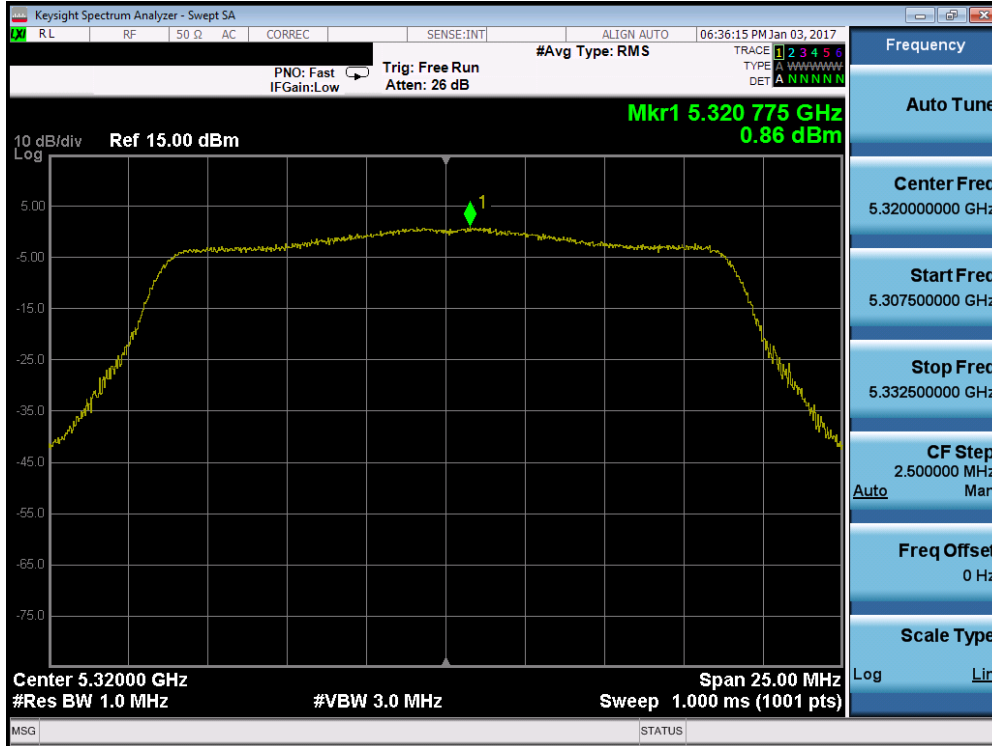
Plot 7-91. Power Spectral Density Plot (20MHz BW 802.11n (UNII Band 2A) – Ch. 64)
