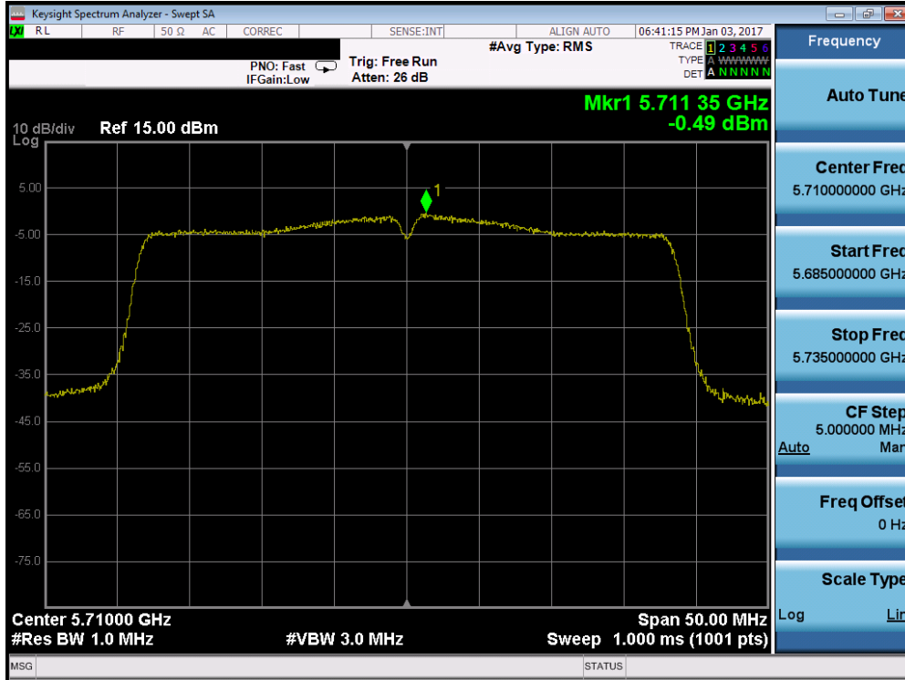
Plot 7-103. Power Spectral Density Plot (40MHz BW 802.11n (UNII Band 2C) – Ch. 142)
