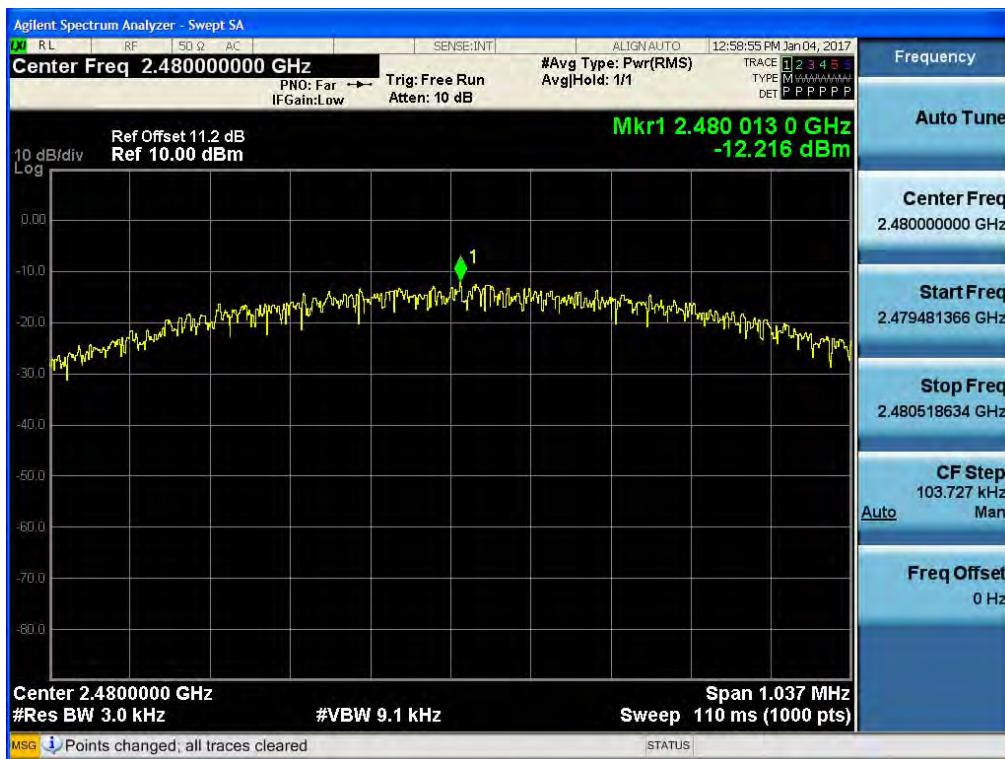
**9.6 OUT OF BAND EMISSIONS AT THE BAND EDGE/ CONDUCTED SPURIOUS EMISSIONS****Test Requirements and limit, §15.247(d) / RSS-247(Issue 1) Section 5.5.**
