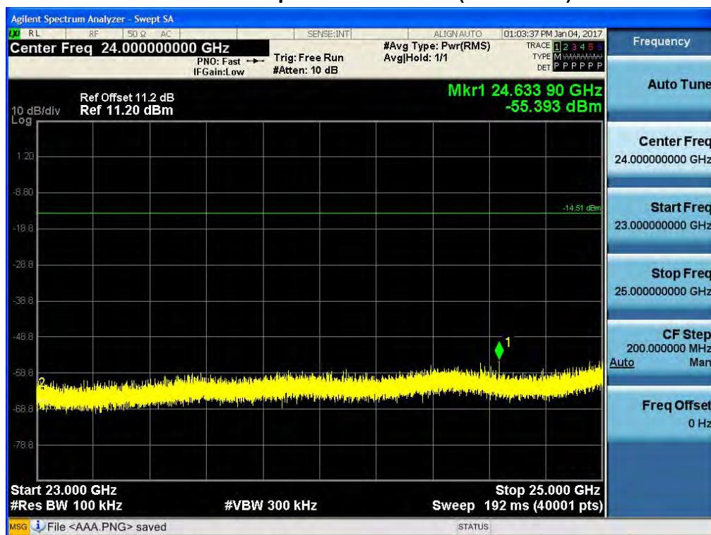
**9.7 RADIATED MEASUREMENT.****9.7.1 RADIATED SPURIOUS EMISSIONS.****Test Requirements and limit, §15.205, §15.209, RSS-Gen(Issue 4) Section 8.9**
