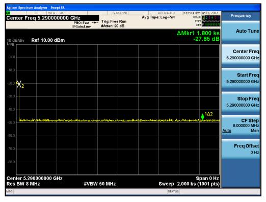
Non-occupancy Period - Monitoring live time spectrum analyzer - Elapse time 30 minutes
