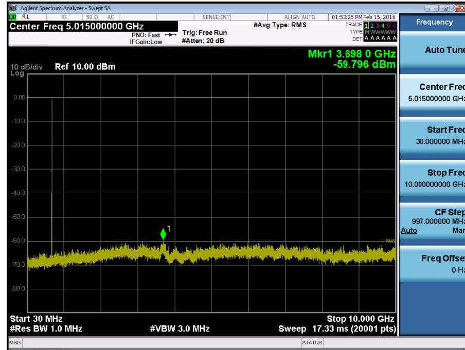
BAND 12. Conducted Spurious Plot \_ (23165ch\_3MHz\_QPSK\_RB 1\_0)
