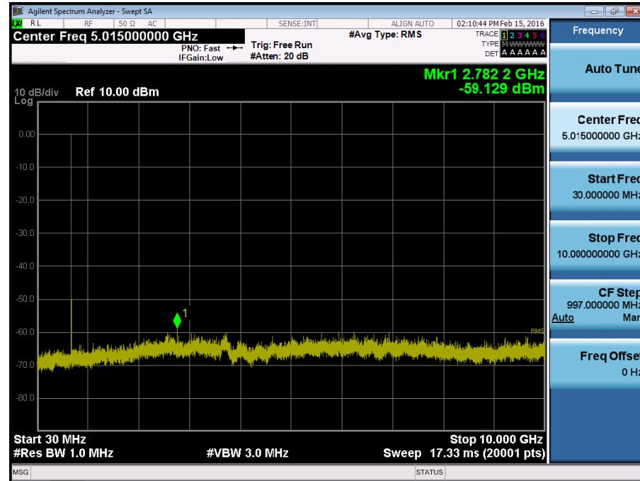
BAND 12. Conducted Spurious Plot \_ (23095ch\_5MHz\_QPSK\_RB 1\_0)
