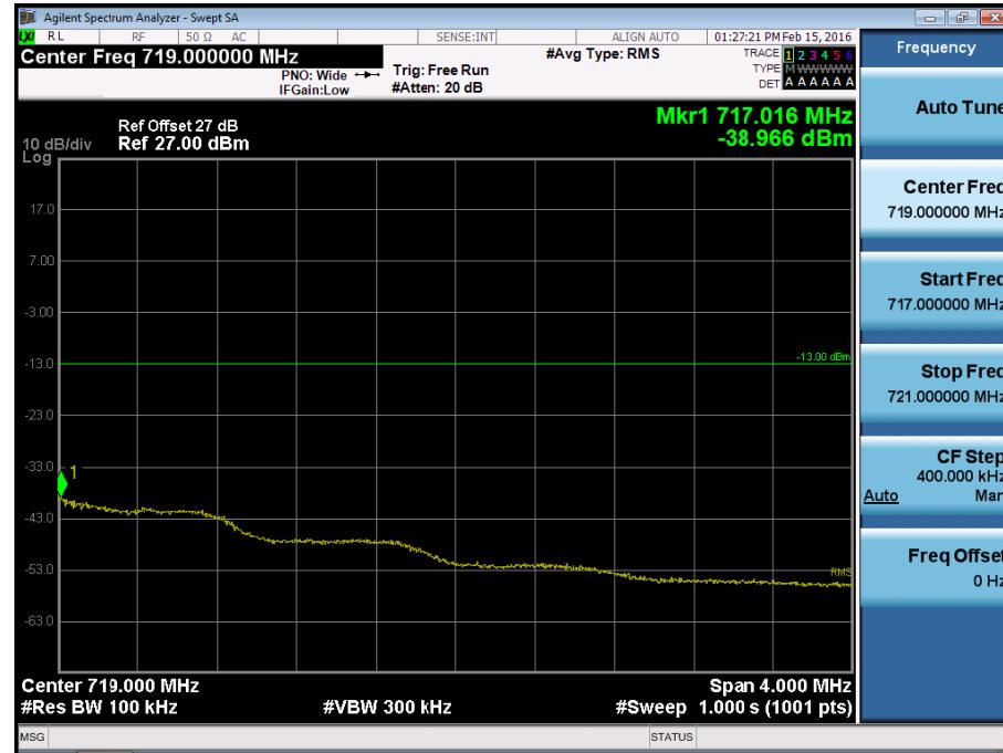
BAND 12. Upper Band Edge Plot (3M BW Ch.23165 QPSK\_RB1\_Offset 14)
