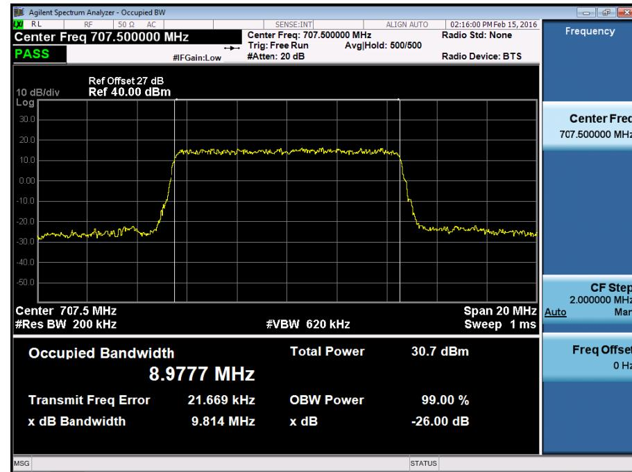
BAND 12. Occupied Bandwidth Plot (10M BW Ch.23095 16QAM\_RB50\_0)
