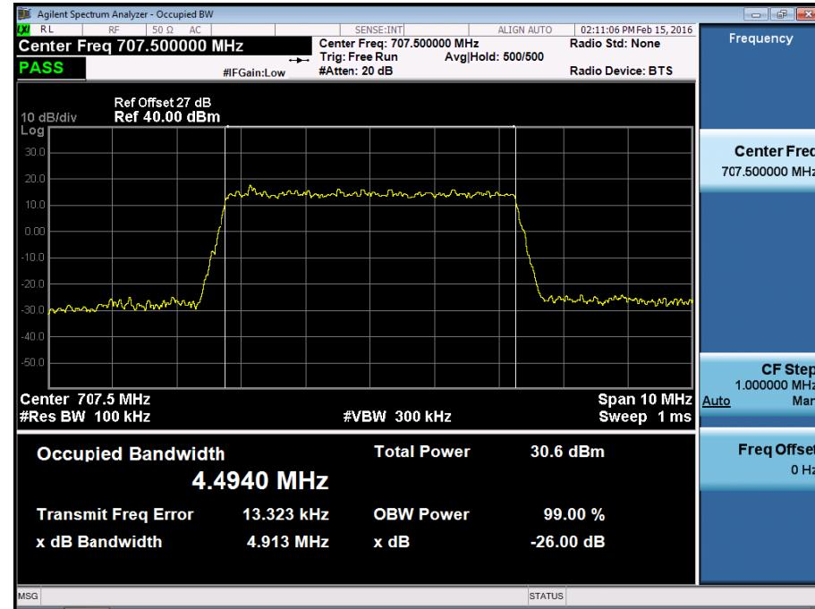
BAND 12. Occupied Bandwidth Plot (5M BW Ch.23095 16QAM\_RB25\_0)
