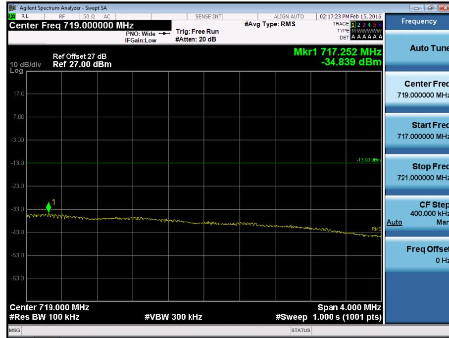
BAND 12. Conducted Spurious Plot \_ (23017ch\_1.4MHz\_QPSK\_RB 1\_0)
