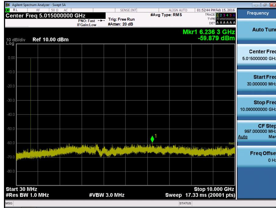
BAND 12. Conducted Spurious Plot \_ (23095ch\_3MHz\_QPSK\_RB 1\_0)
