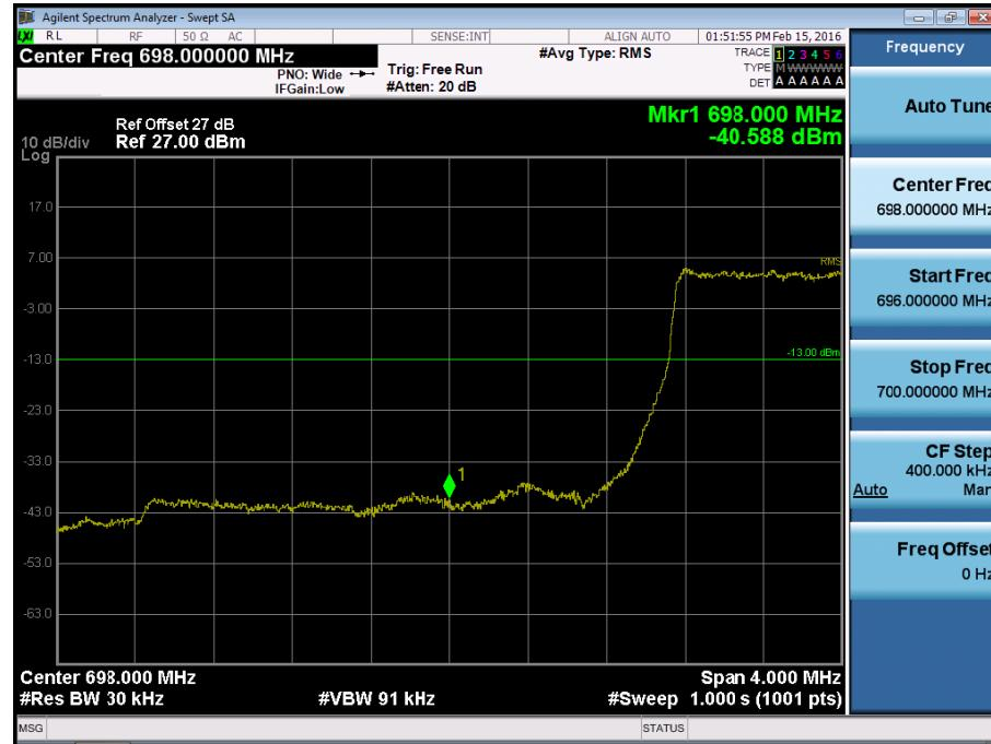
BAND 12. Lower Extended Band Edge Plot (3M BW Ch.23025 QPSK\_RB15\_0)
