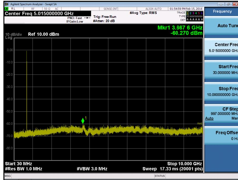
BAND 12. Conducted Spurious Plot \_ (23035ch\_5MHz\_QPSK\_RB 1\_0)
