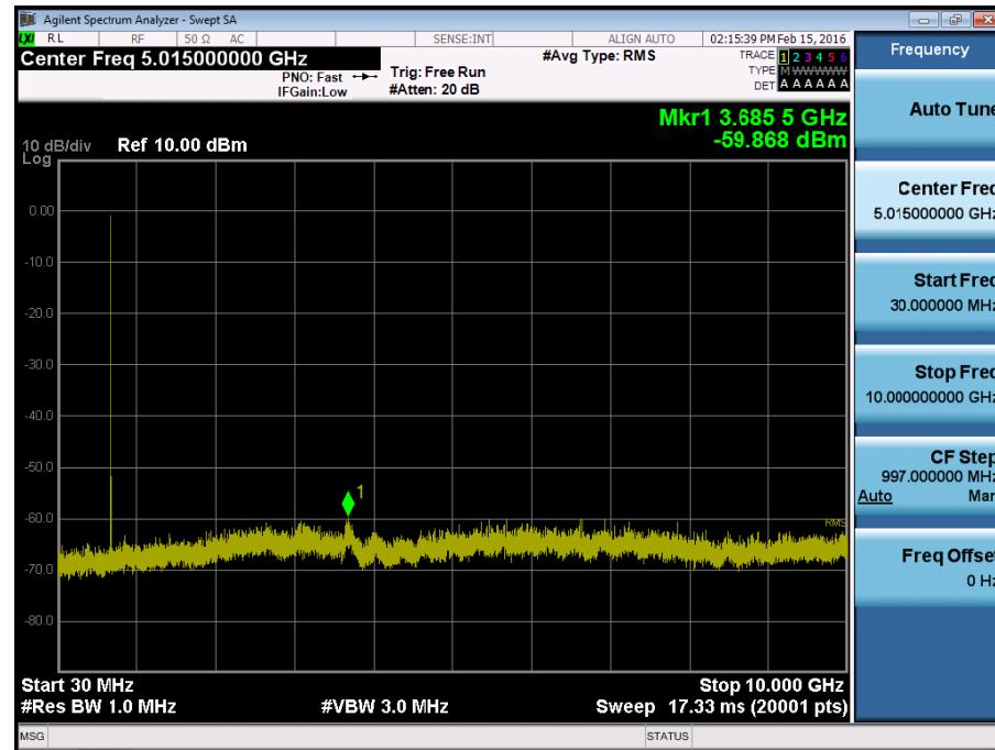
BAND 12. Conducted Spurious Plot \_ (23095ch\_10MHz\_QPSK\_RB 1\_0)
