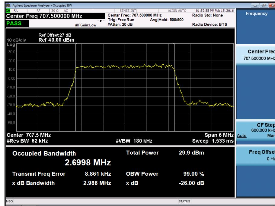
BAND 12. Occupied Bandwidth Plot (5M BW Ch.23095 QPSK\_RB25\_0)
