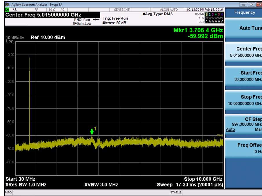
BAND 12. Conducted Spurious Plot \_ (23060ch\_10MHz\_QPSK\_RB 1\_0)
