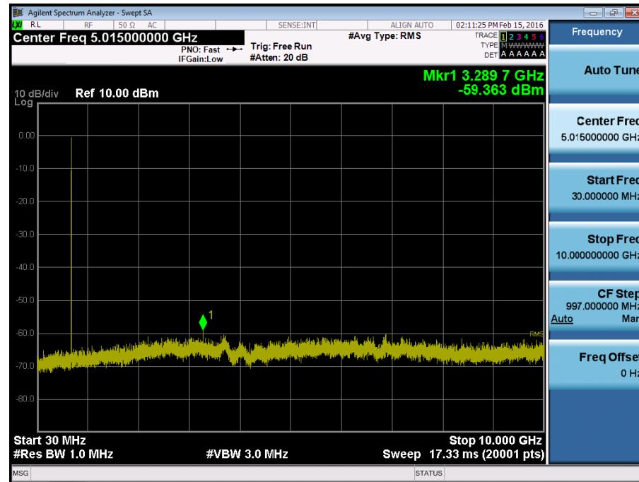
BAND 12. Conducted Spurious Plot \_ (23155ch\_5MHz\_QPSK\_RB 1\_0)
