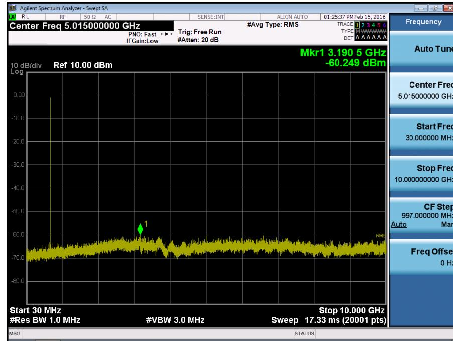
BAND 12. Conducted Spurious Plot \_ (23095ch\_1.4MHz\_QPSK\_RB 1\_0)
