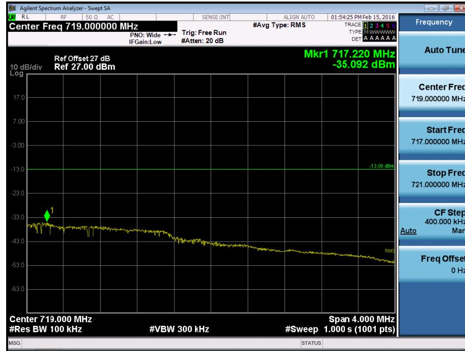
BAND 12. Upper Band Edge Plot (5M BW Ch.23155 QPSK\_RB1\_Offset 24)
