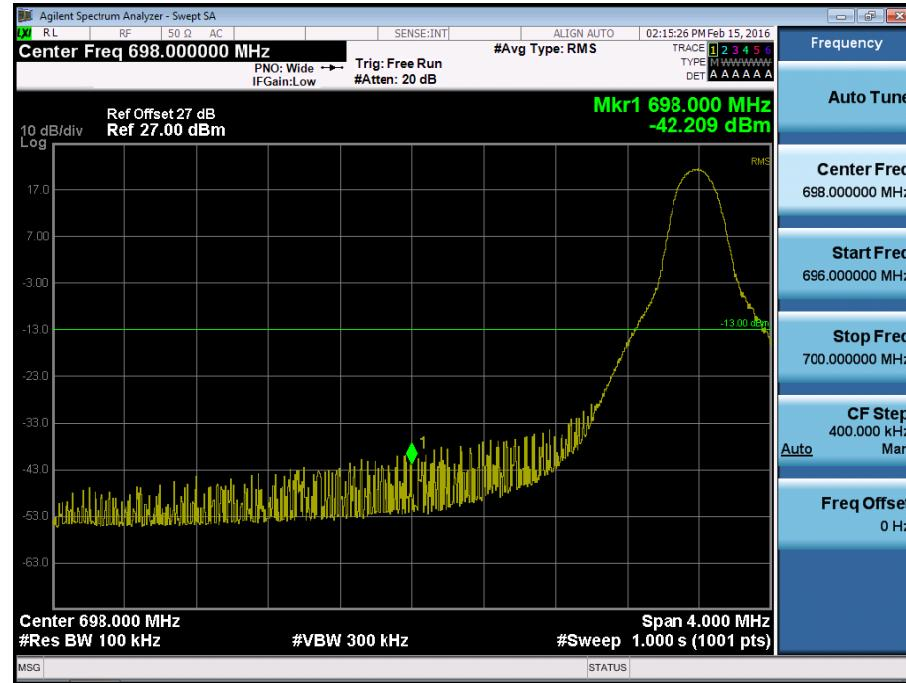
BAND 12. Lower Band Edge Plot (10M BW Ch.23060 QPSK\_RB50\_Offset 0)
