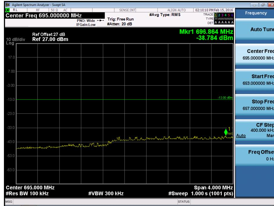
BAND 12. Lower Band Edge Plot (10M BW Ch.23060 QPSK\_RB1\_Offset 0)
