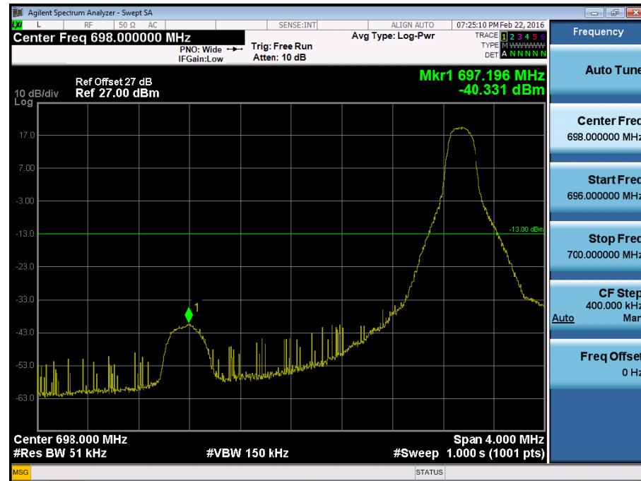
BAND 12. Lower Band Edge Plot (5M BW Ch.23035 QPSK\_RB25\_Offset 0)
