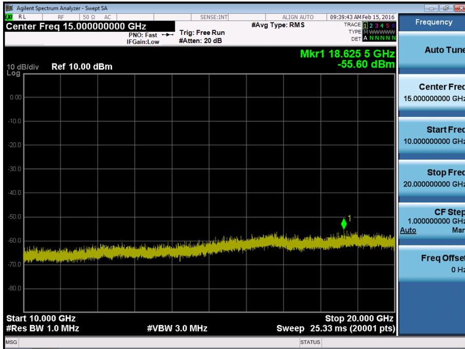
BAND 4. Conducted Spurious Plot\_1 (19965ch\_3MHz\_QPSK\_RB 1\_0)
