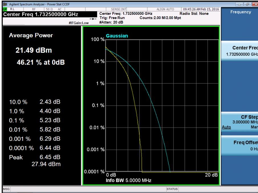
BAND 4. PAR Plot (5M BW\_Ch.20175\_16QAM\_RB25\_0)
