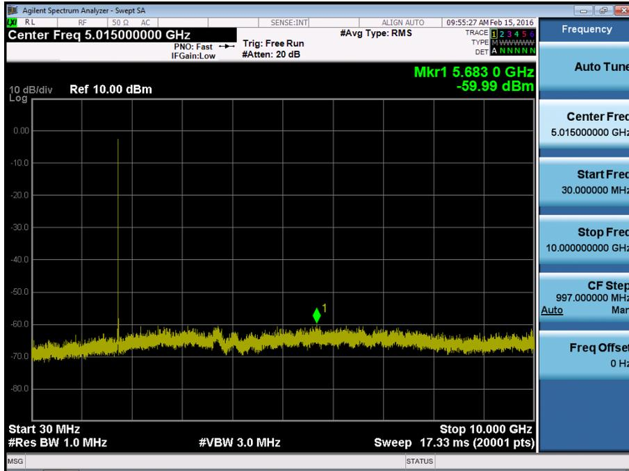
BAND 4. Conducted Spurious Plot\_2 (20325ch\_15MHz\_QPSK\_RB 1\_0)
