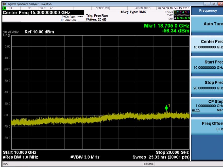
BAND 17. Conducted Spurious Plot\_ (23755ch\_5MHz\_QPSK\_RB 1\_0)
