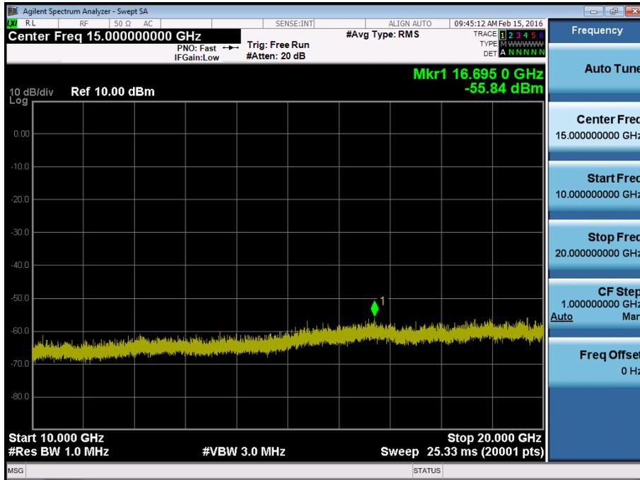
BAND 4. Conducted Spurious Plot\_1 (20175ch\_5MHz\_QPSK\_RB 1\_0)
