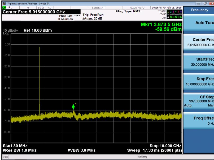
BAND 4. Conducted Spurious Plot\_2 (19957ch\_1.4MHz\_QPSK\_RB 1\_0)
