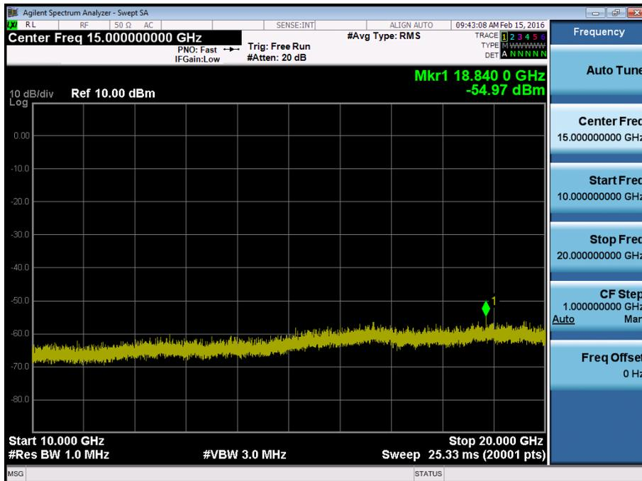
BAND 4. Conducted Spurious Plot\_1 (20385ch\_3MHz\_QPSK\_RB 1\_0)
