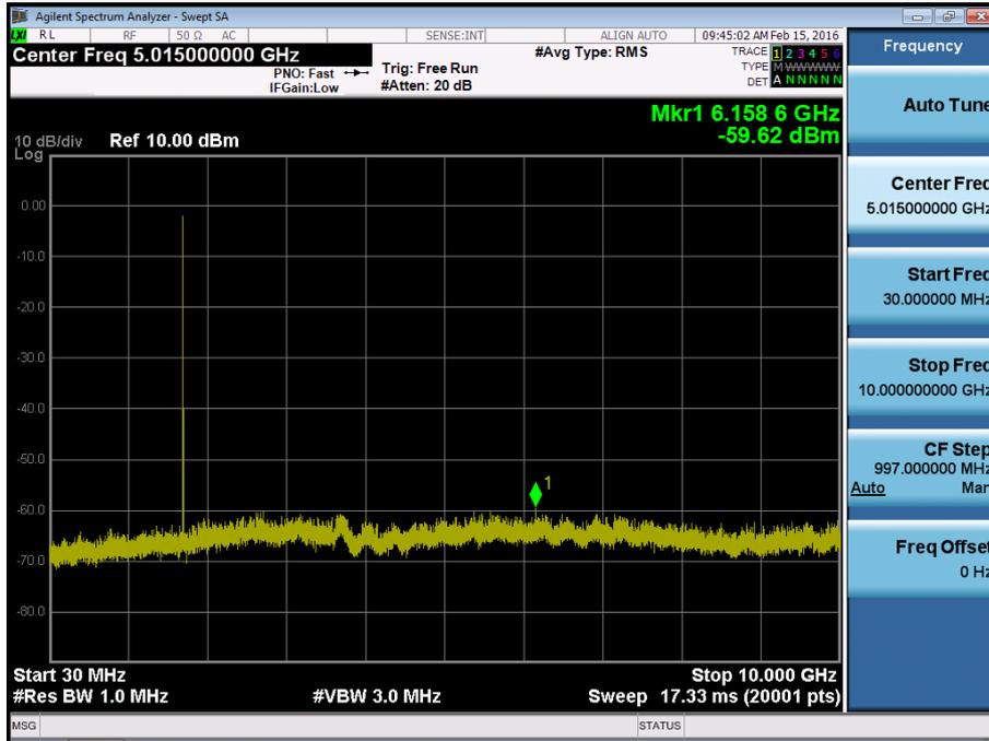
BAND 4. Conducted Spurious Plot\_2 (19975ch\_5MHz\_QPSK\_RB 1\_0)
