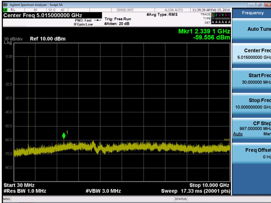
BAND 17. Conducted Spurious Plot\_ (23825ch\_5MHz\_QPSK\_RB 1\_0)
