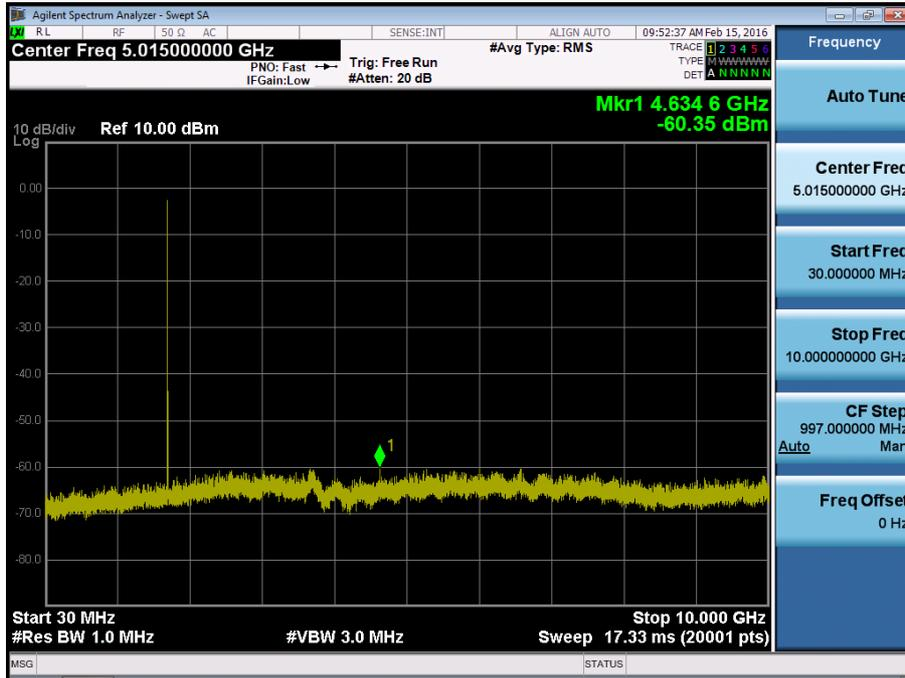
BAND 4. Conducted Spurious Plot\_2 (20025ch\_15MHz\_QPSK\_RB 1\_0)
