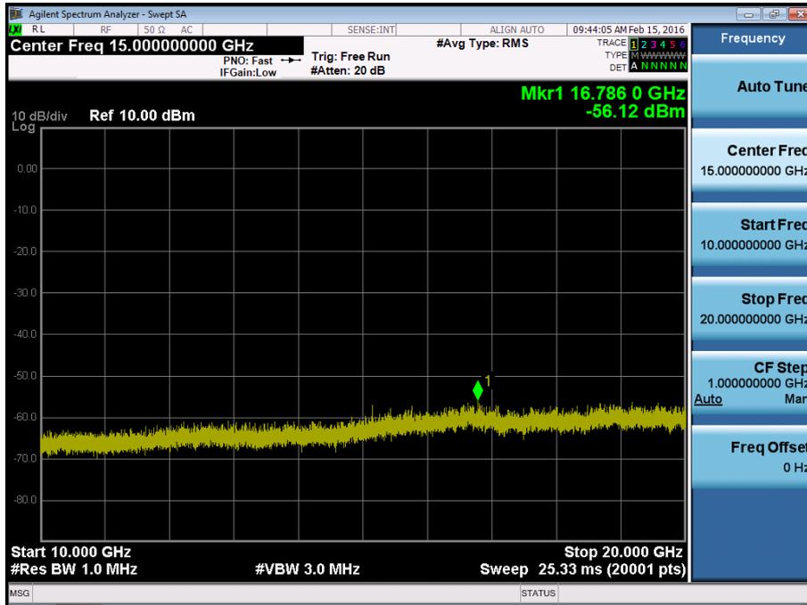
BAND 4. Conducted Spurious Plot\_1 (19975ch\_5MHz\_QPSK\_RB 1\_0)
