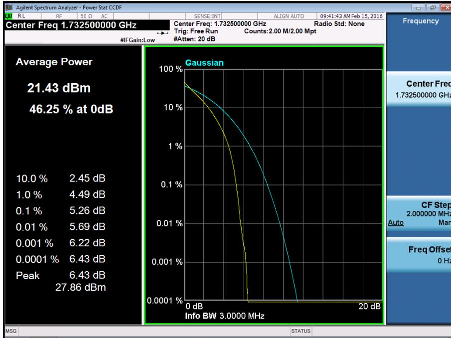
BAND 4. PAR Plot (3M BW\_Ch.20175\_16QAM\_RB15\_0)
