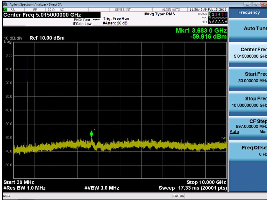
BAND 17. Conducted Spurious Plot\_ (23800ch\_10MHz\_QPSK\_RB 1\_0)
