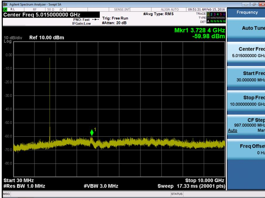
BAND 4. Conducted Spurious Plot\_2 (20350ch\_10MHz\_QPSK\_RB 1\_0)
