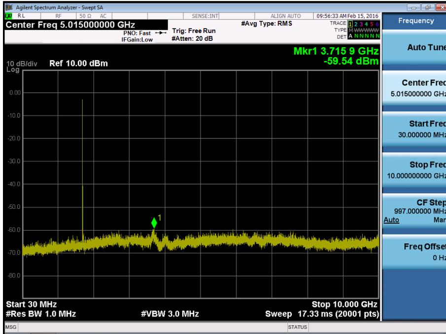
BAND 4. Conducted Spurious Plot\_2 (20050ch\_20MHz\_QPSK\_RB 1\_0)
