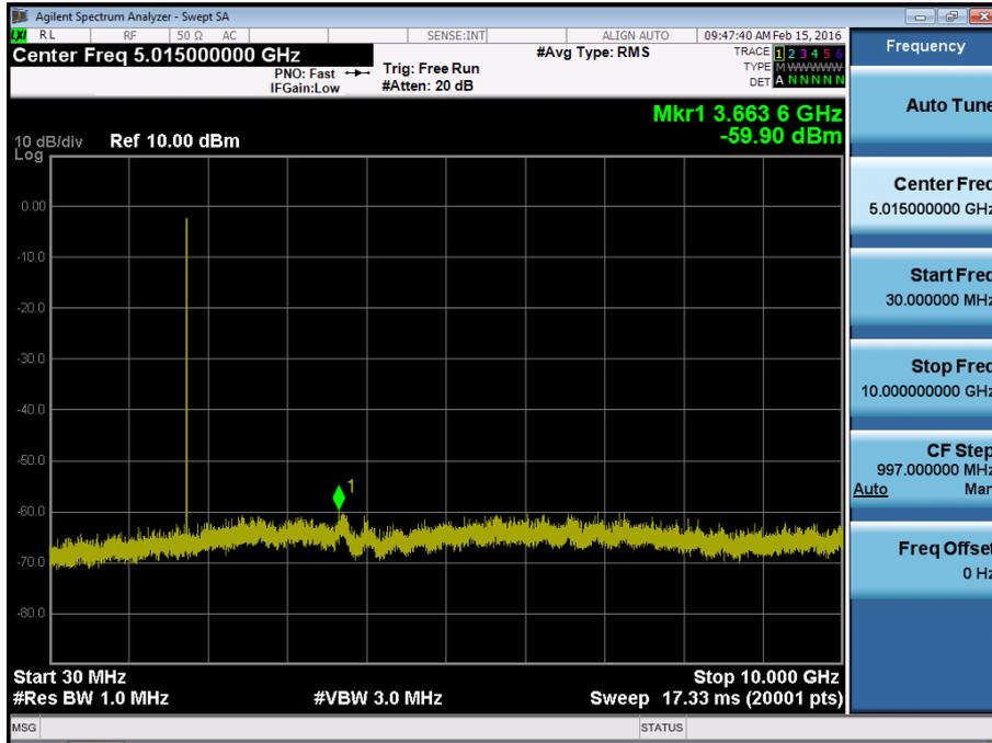
BAND 4. Conducted Spurious Plot\_2 (20375ch\_5MHz\_QPSK\_RB 1\_0)
