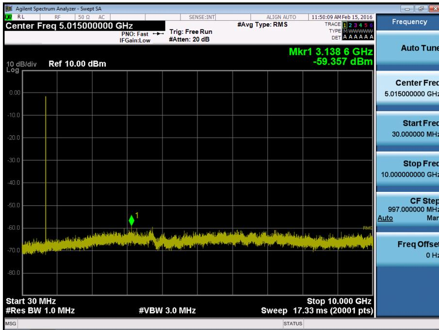
BAND 17. Conducted Spurious Plot\_ (23790ch\_10MHz\_QPSK\_RB 1\_0)
