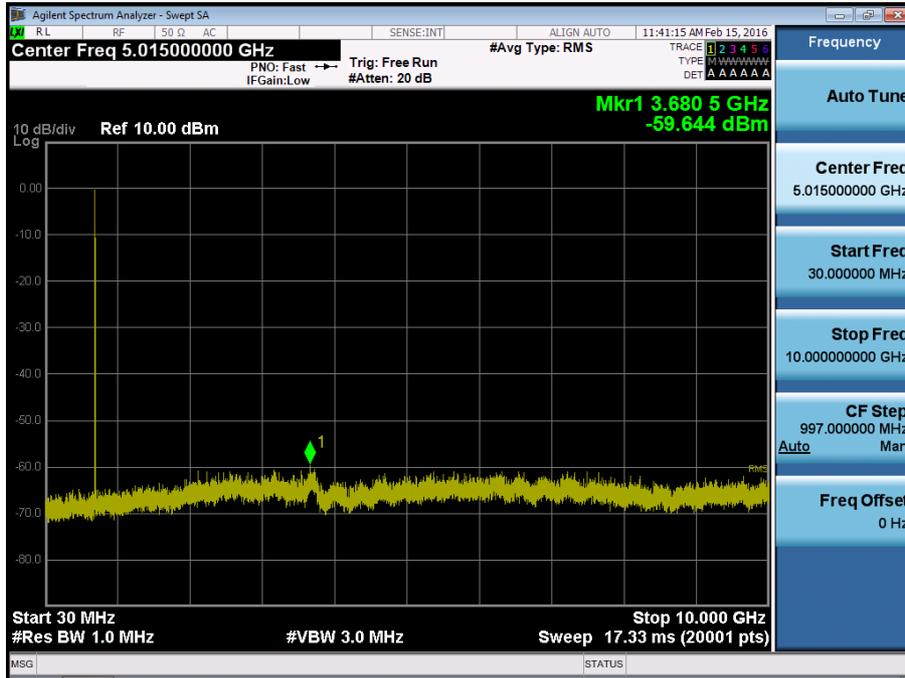
BAND 17. Conducted Spurious Plot\_ (23780ch\_10MHz\_QPSK\_RB 1\_0)
