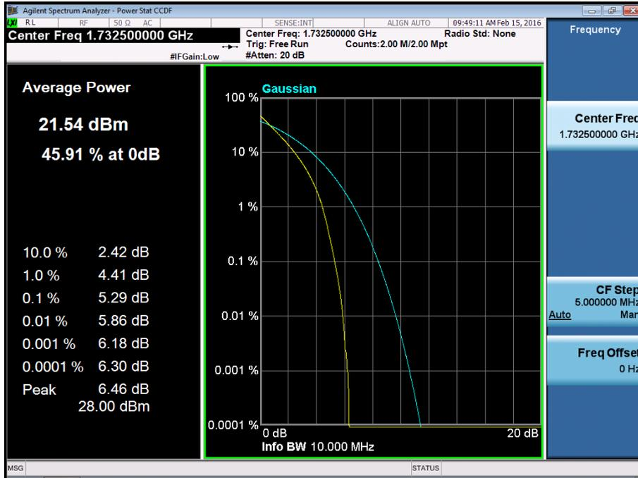
BAND 4. PAR Plot (10M BW\_Ch.20175\_16QAM\_RB50\_0)
