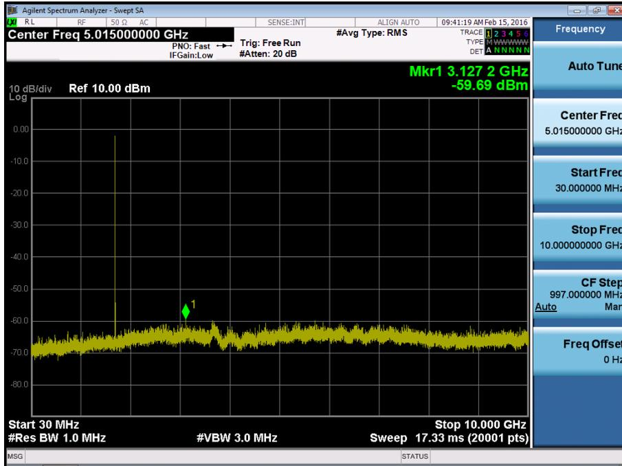
BAND 4. Conducted Spurious Plot\_2 (19965ch\_3MHz\_QPSK\_RB 1\_0)
