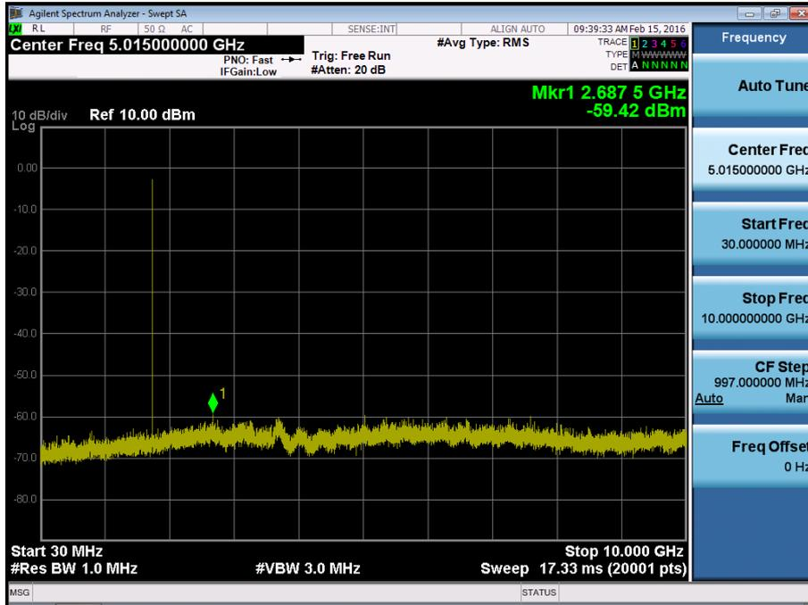
BAND 4. Conducted Spurious Plot\_2 (20393ch\_1.4MHz\_QPSK\_RB 1\_0)
