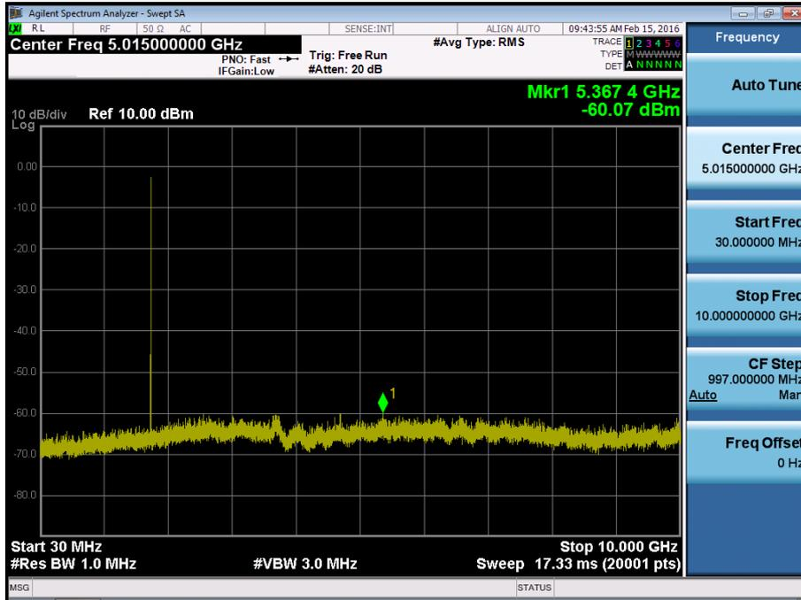
BAND 4. Conducted Spurious Plot\_2 (20385ch\_3MHz\_QPSK\_RB 1\_0)
