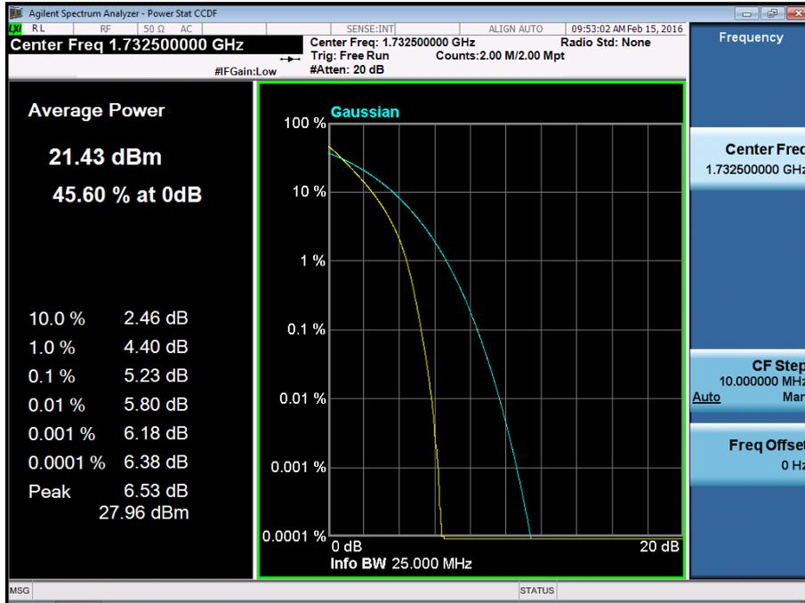
BAND 4. PAR Plot (15M BW\_Ch.20175\_16QAM\_RB75\_0)
