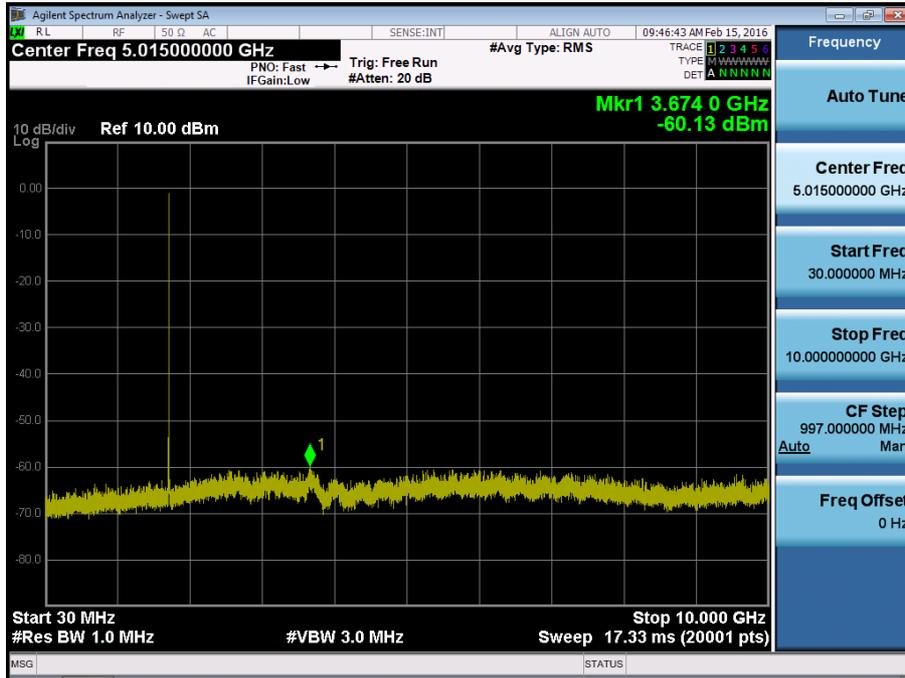
BAND 4. Conducted Spurious Plot\_2 (20175ch\_5MHz\_QPSK\_RB 1\_0)
