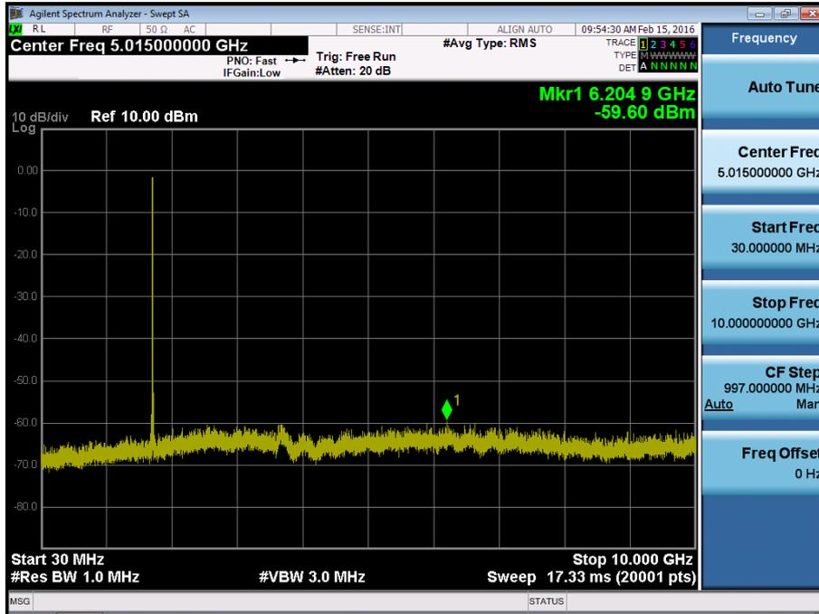
BAND 4. Conducted Spurious Plot\_2 (20175ch\_15MHz\_QPSK\_RB 1\_0)
