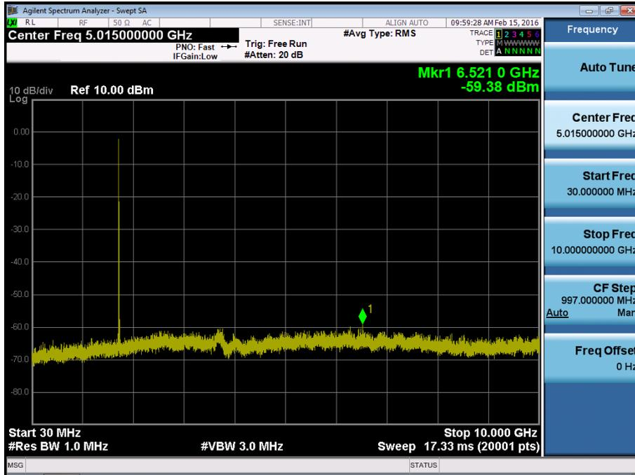
BAND 4. Conducted Spurious Plot\_2 (20300ch\_20MHz\_QPSK\_RB 1\_0)
