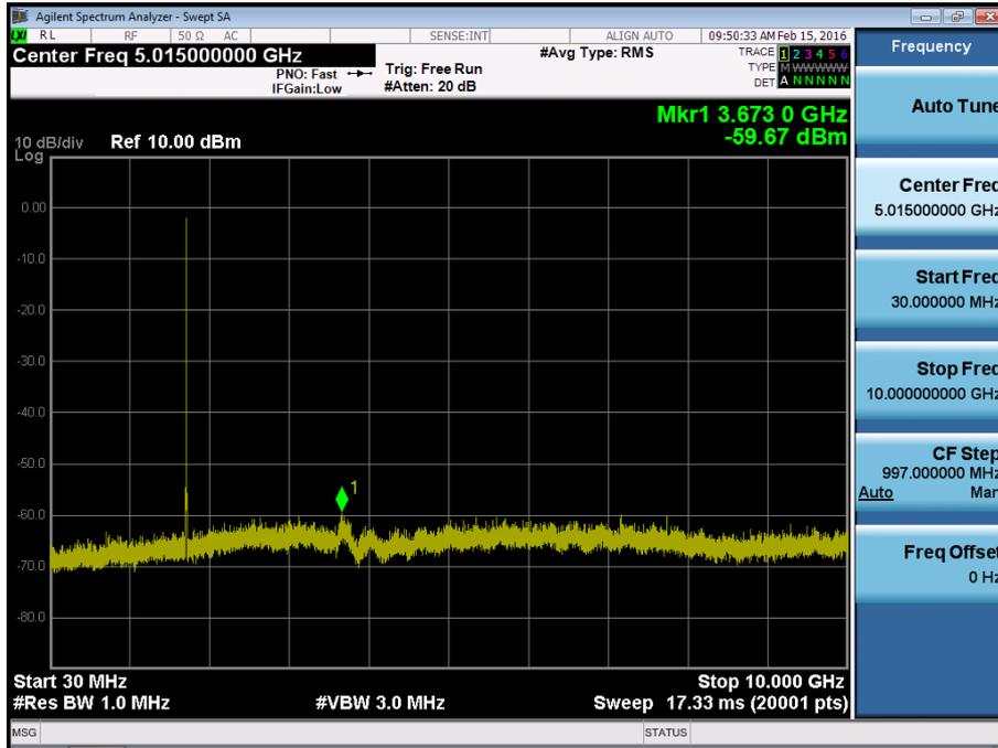
BAND 4. Conducted Spurious Plot\_2 (20175ch\_10MHz\_QPSK\_RB 1\_0)
