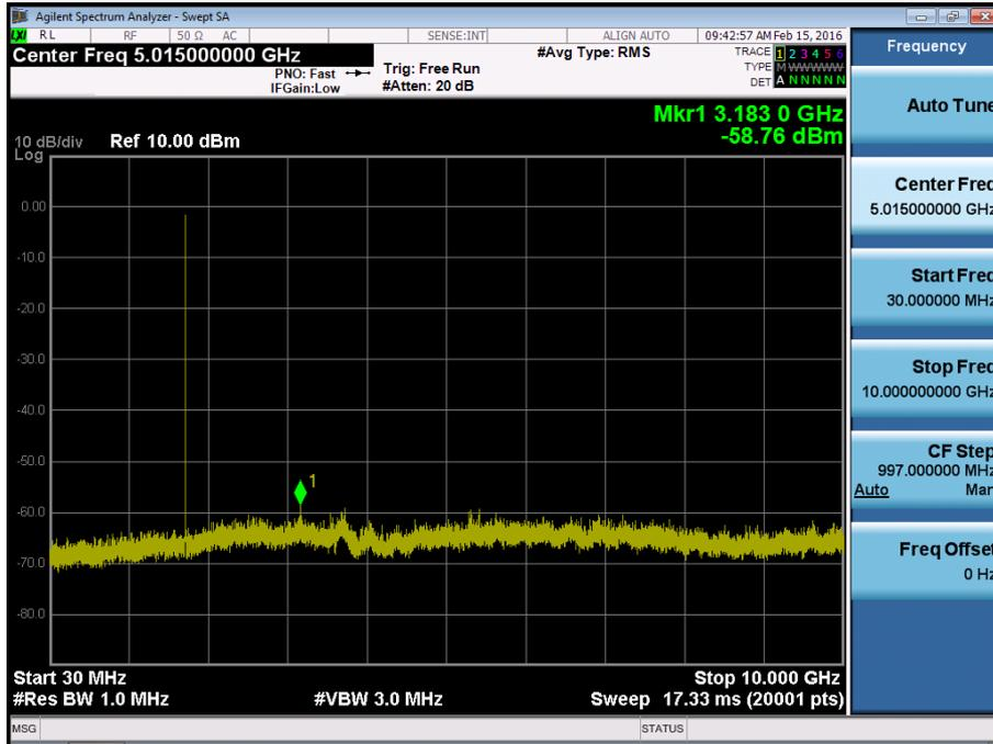
BAND 4. Conducted Spurious Plot\_2 (20175ch\_3MHz\_QPSK\_RB 1\_0)
