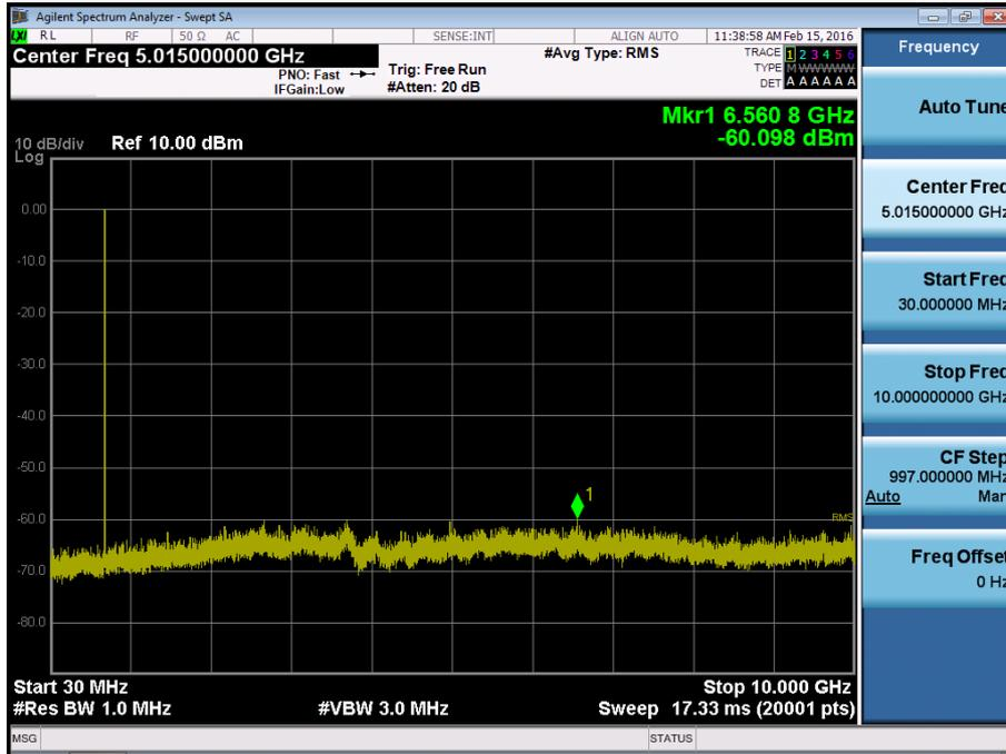
BAND 17. Conducted Spurious Plot\_ (23790ch\_5MHz\_QPSK\_RB 1\_0)
