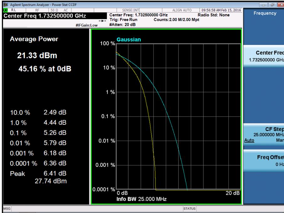
BAND 4. PAR Plot (20M BW\_Ch.20175\_16QAM\_RB100\_0)
