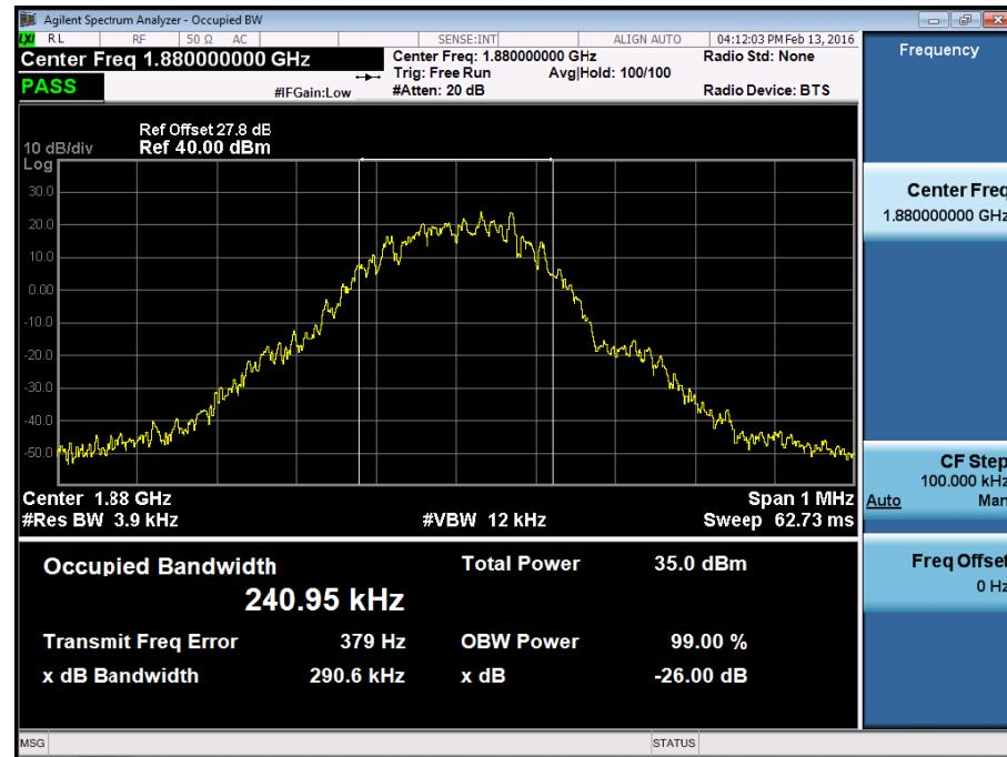
■ GSM1900 MODE (810 CH.) Occupied Bandwidth
