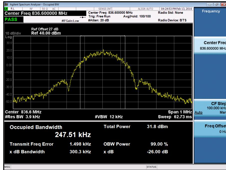
■ GSM1900 MODE (512 CH.) Occupied Bandwidth
