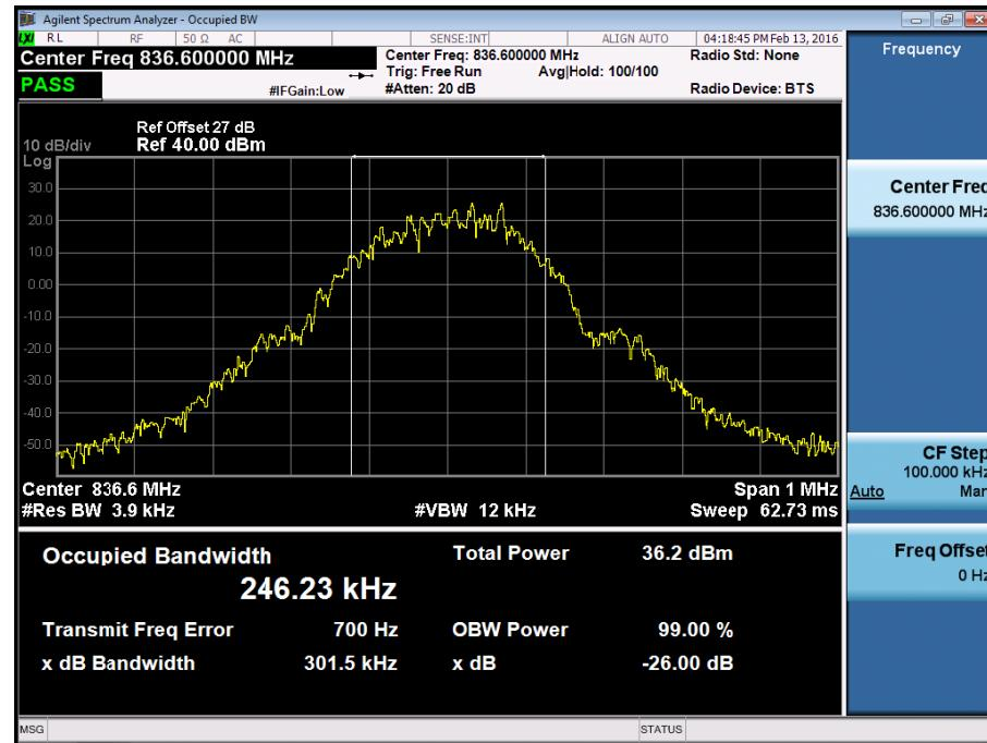
■ GSM850 MODE (251 CH.) Occupied Bandwidth
