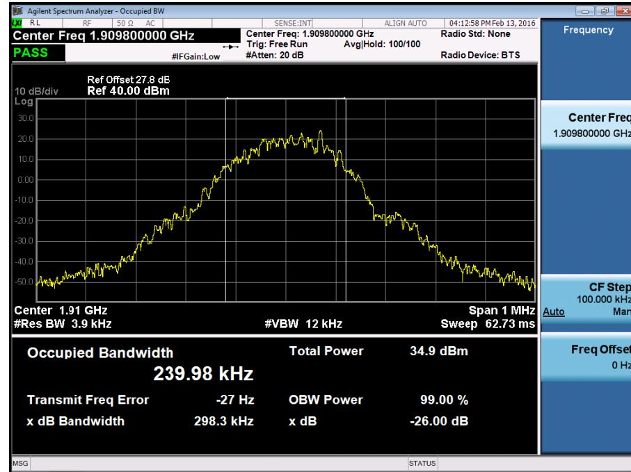
■ GSM1900 EDGE (512 CH.) Occupied Bandwidth
