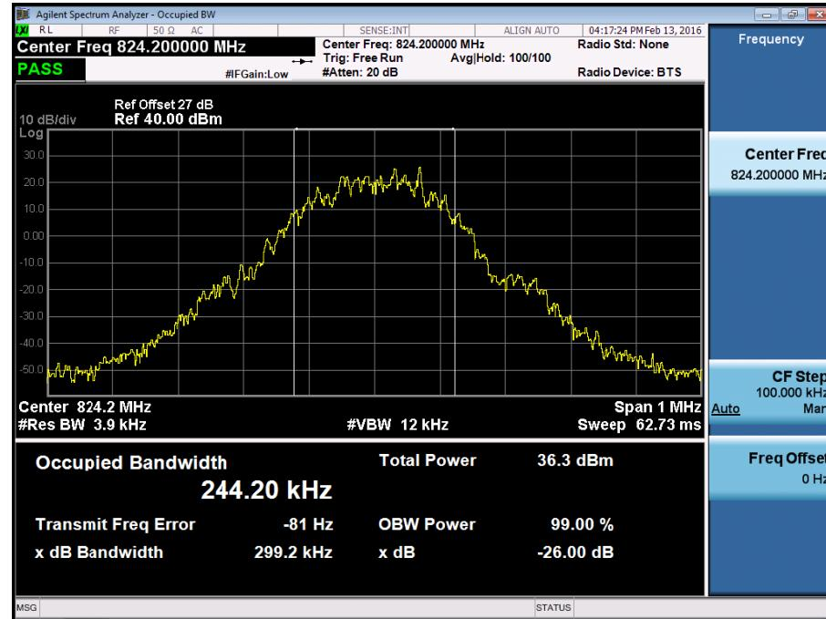
■ GSM850 MODE (190 CH.) Occupied Bandwidth
