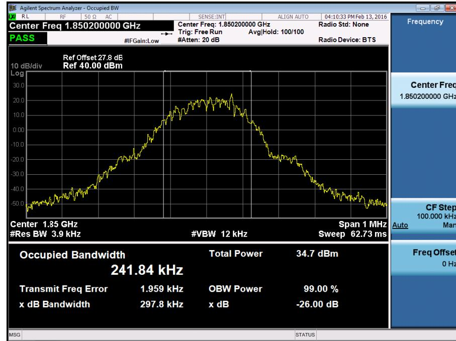
■ GSM1900 MODE (661 CH.) Occupied Bandwidth
