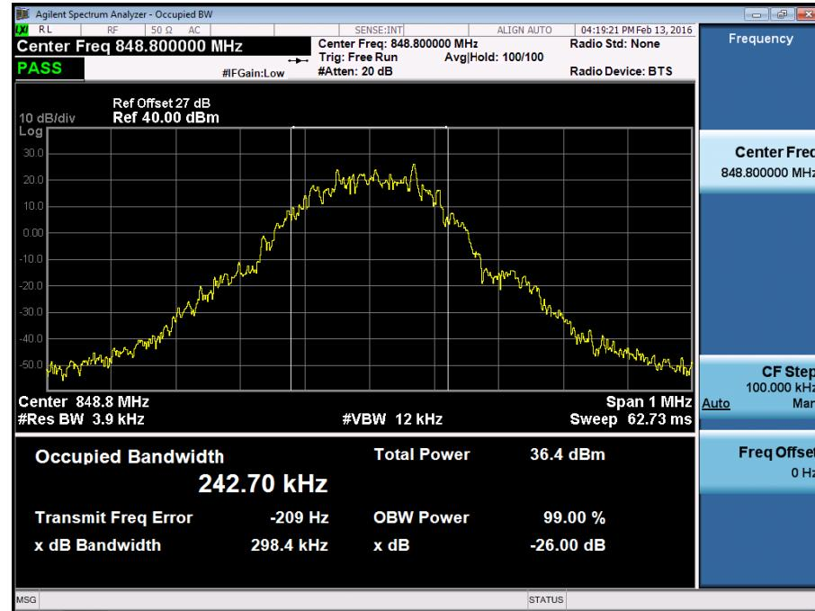
■ GSM850 EDGE (190 CH.) Occupied Bandwidth
