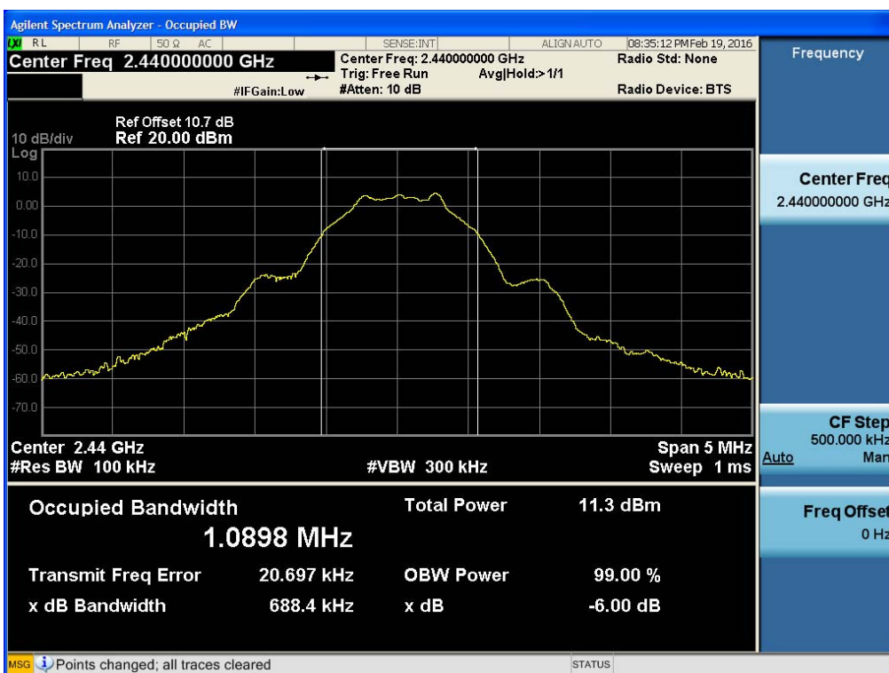
6dB Bandwidth plot (Mid-CH 19)
