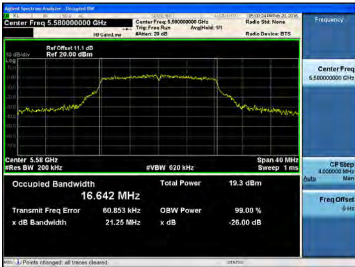
802.11a UNII 2C BAND 26dB Bandwidth (CH116)
