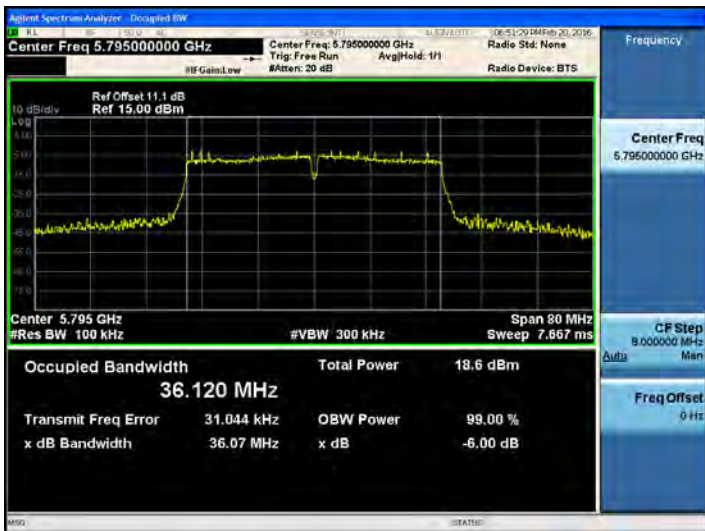
802.11n_40 MHz BW UNII 3 BAND 6dB Bandwidth(CH.159)
