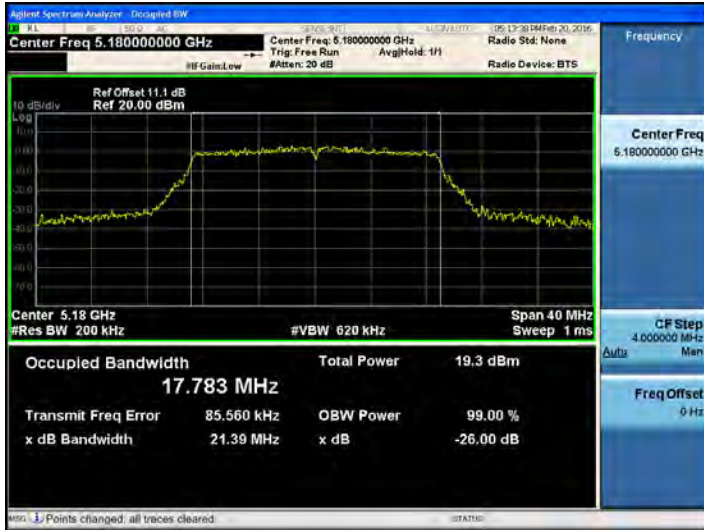
802.11n_20 MHz BW UNII 2C BAND 26dB Bandwidth(CH 100)
