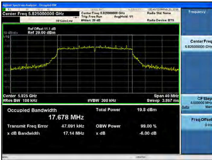
802.11ac_20 MHz BW UNII 3 BAND 6dB Bandwidth(CH.165)
