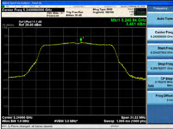
802.11a_20MHz BW UNII 2C BAND PSD CH 100
