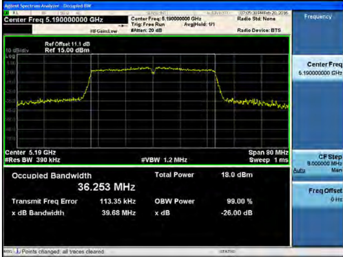
802.11ac_40 MHz BW UNII 2C BAND 26dB Bandwidth(CH 102)
