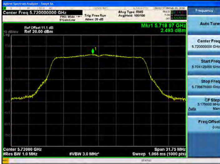
802.11n_20MHz BW UNII 2C Band PSD CH.144
