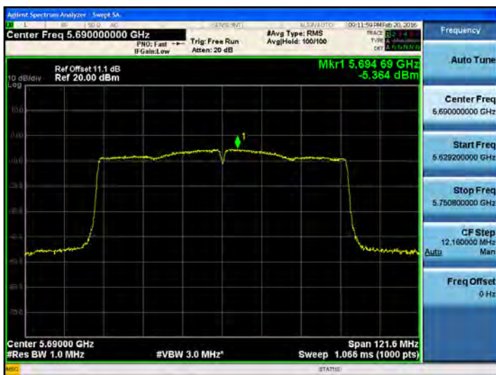
802.11ac_80MHz BW UNII 2C Band PSD CH.138
