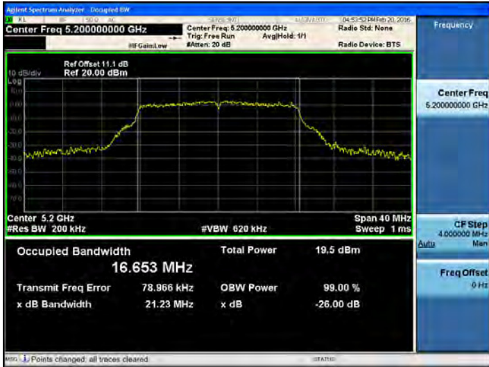
802.11a UNII 2C BAND 26dB Bandwidth (CH116)
