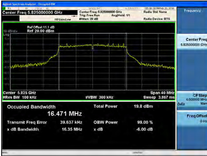
802.11ac_20 MHz BW UNII 3 BAND 6dB Bandwidth(CH.165)
