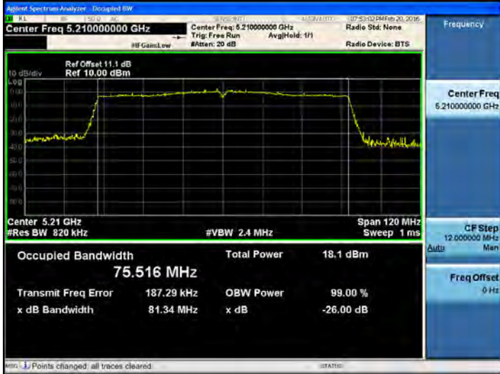
802.11ac_80 MHz BW UNII 2C BAND 26dB Bandwidth(CH 138)
