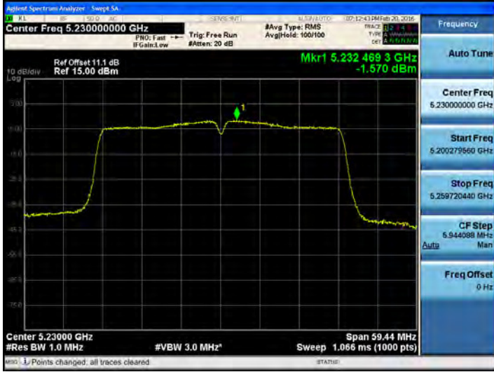
802.11ac_40MHz BW UNII 2C BAND PSD CH 110
