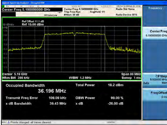
802.11n_40 MHz BW UNII 2C BAND 26dB Bandwidth(CH 102)
