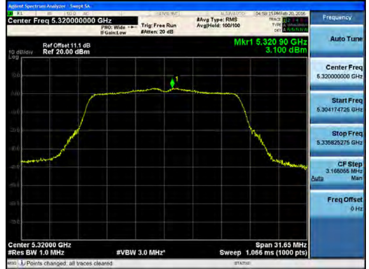
802.11a_20MHz BW UNII 3 BAND PSD CH 165
