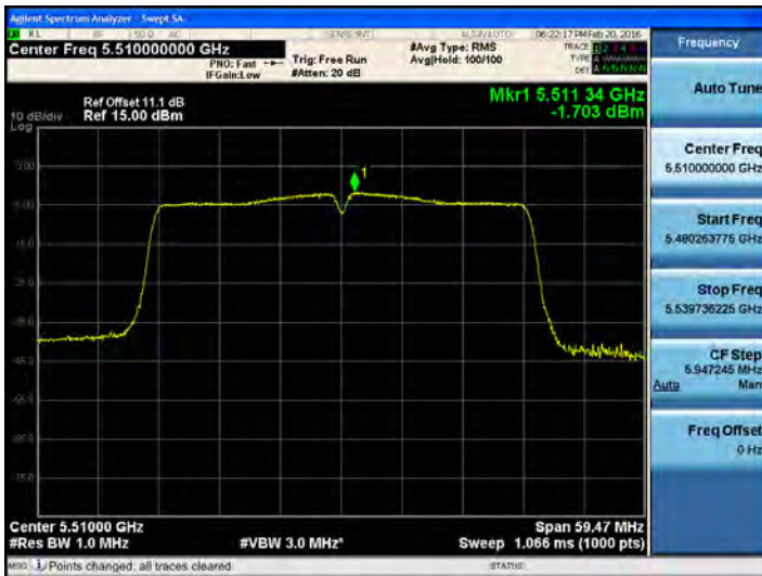
802.11n_40MHz BW UNII 2C BAND PSD CH 102
