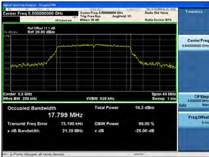
802.11n_20 MHz BW UNII 2C BAND 26dB Bandwidth(CH 100)
