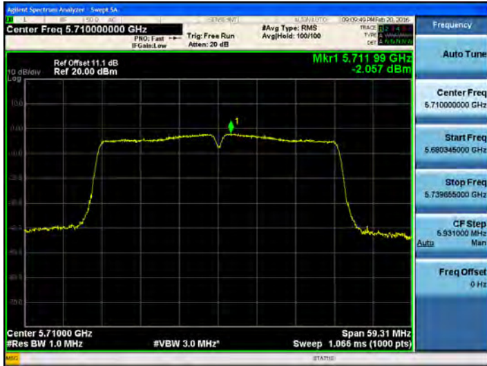
802.11ac_40MHz BW UNII 2C Band PSD CH.142
