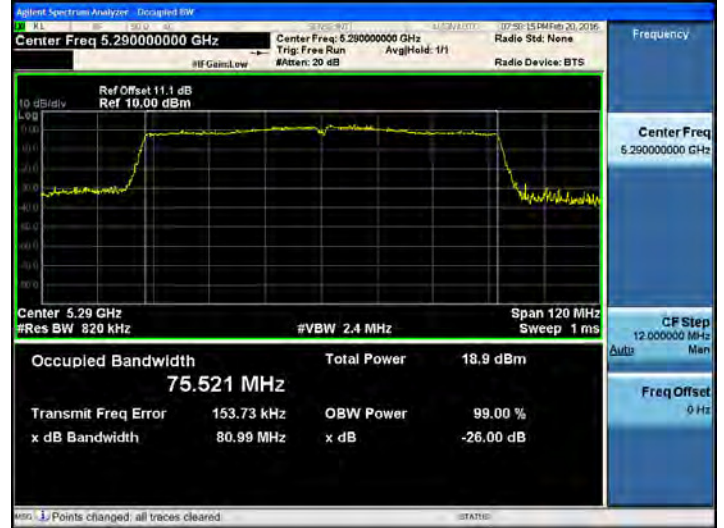
802.11ac_80 MHz BW UNII 3 BAND 26dB Bandwidth(CH 155)
