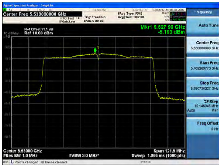
802.11ac_80MHz BW UNII 2C BAND PSD CH 106
