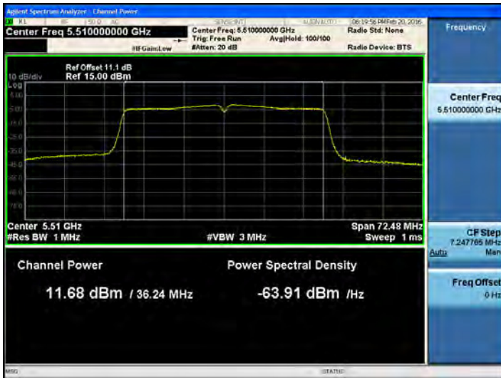
802.11n_40 MHz BW UNII 2C BAND Average Power (5510 MHz ~5710 MHz) CH 102MCS0
