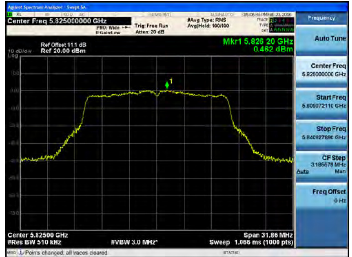
802.11a_20MHz BW UNII 3 BAND PSD CH 165
