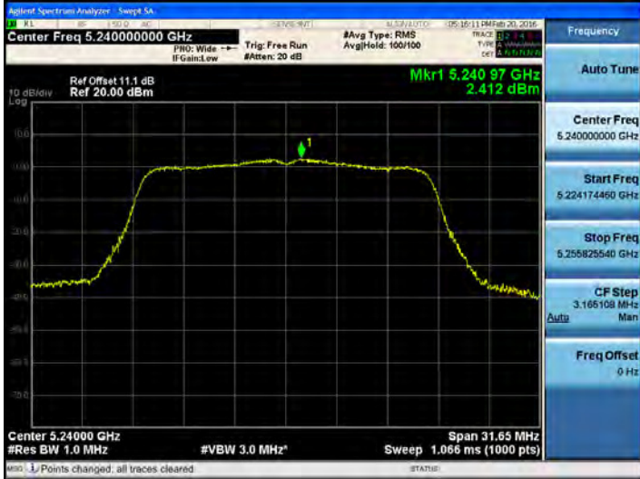
802.11n_20MHz BW UNII 2C BAND PSD CH 100
