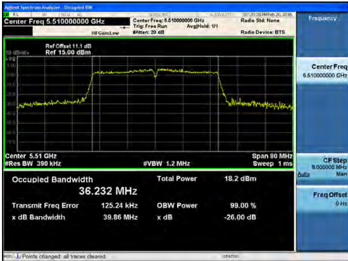
802.11ac_40 MHz BW UNII 2C BAND 26dB Bandwidth(CH 102)
