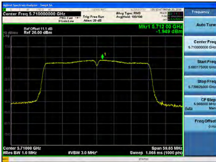
802.11ac_40MHz BW UNII 2C Band PSD CH.142
