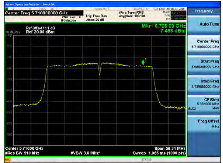
802.11ac_40MHz BW UNII 3 Band PSD CH.142
