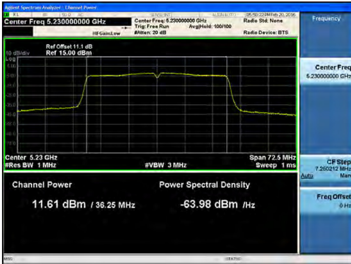
802.11n_40 MHz BW UNII 2C BAND Average Power (5510 MHz ~5710 MHz) CH 102MCS0
