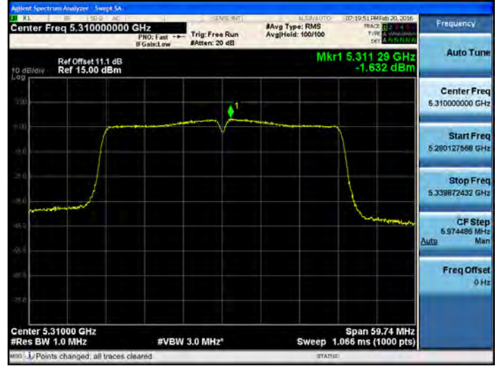
802.11ac_40MHz BW UNII 3 BAND PSD CH 159
