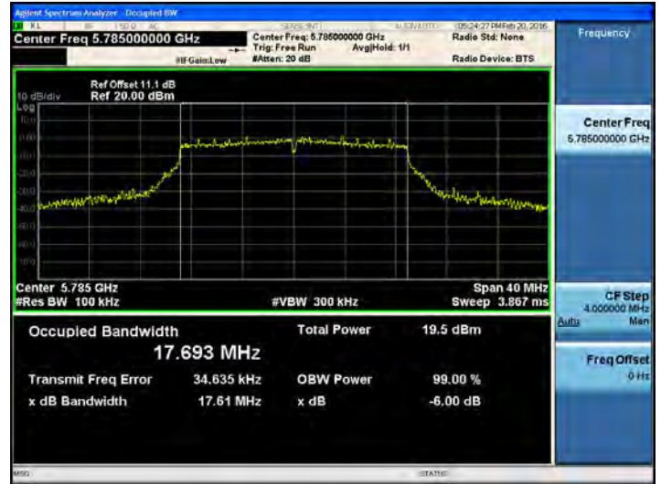
802.11n_20 MHz BW UNII 3 BAND 6dB Bandwidth(CH.157)
