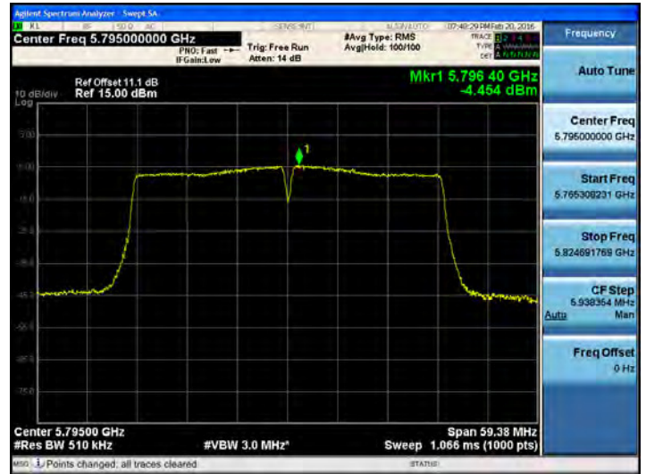
802.11ac_40MHz BW UNII 3 BAND PSD CH 159
