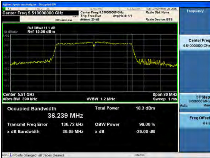
802.11n_40 MHz BW UNII 2C BAND 26dB Bandwidth(CH 102)
