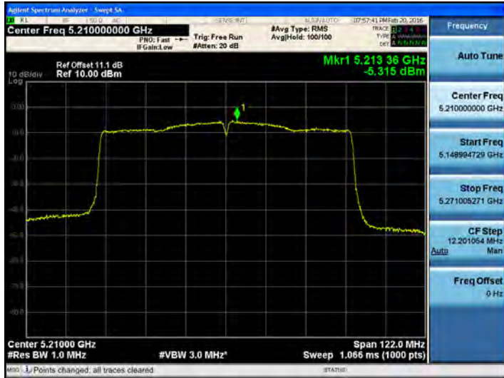
802.11ac_80MHz BW UNII 2C BAND PSD CH 106
