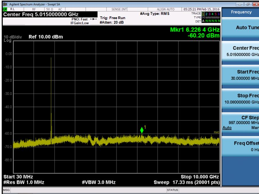
BAND 2. Conducted Spurious\_2 (18700ch\_20MHz\_QPSK\_RB 1\_0)
