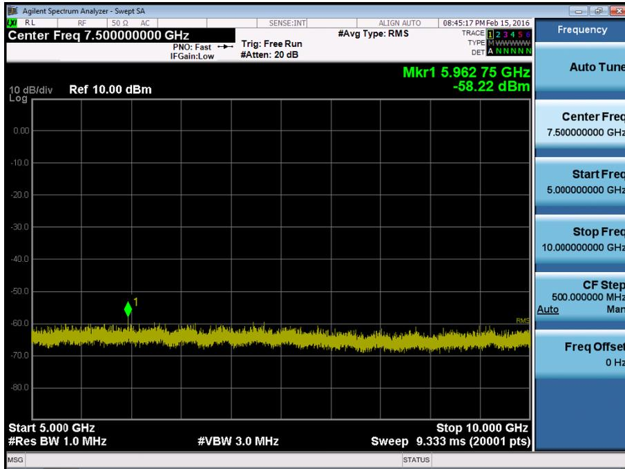
BAND 5. Conducted Spurious Plot \_1 (20425ch\_5MHz\_QPSK\_RB 1\_0)
