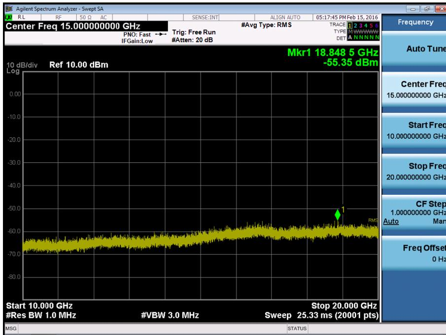
BAND 2. Conducted Spurious\_1 (18900ch\_10MHz\_QPSK\_RB 1\_0)
