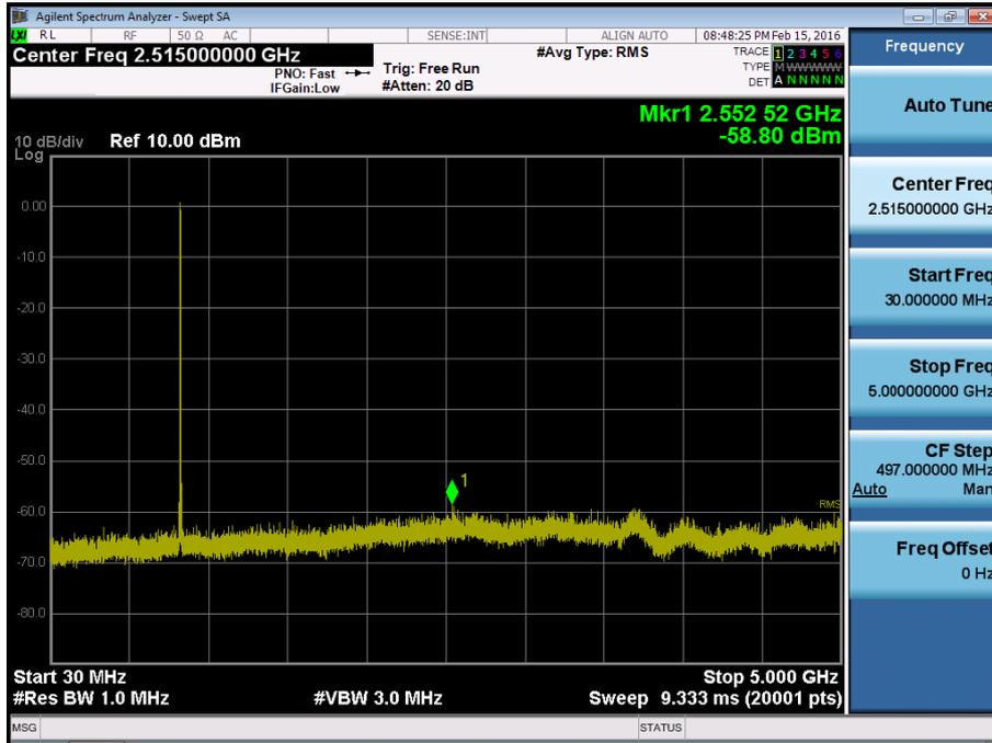
BAND 5. Conducted Spurious Plot \_2 (20625ch\_5MHz\_QPSK\_RB 1\_0)
