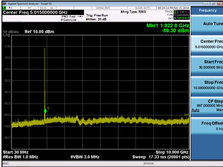
BAND 2. Conducted Spurious\_2 (19125ch\_15MHz\_QPSK\_RB 1\_0)
