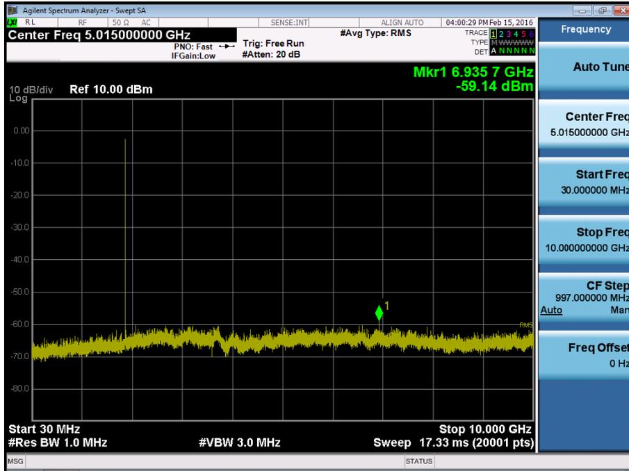
BAND 2. Conducted Spurious\_2 (18900ch\_1.4MHz\_QPSK\_RB 1\_0)
