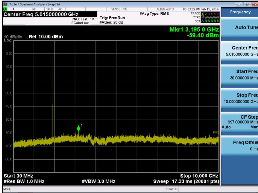
BAND 2. Conducted Spurious\_2 (19175ch\_5MHz\_QPSK\_RB 1\_0)
