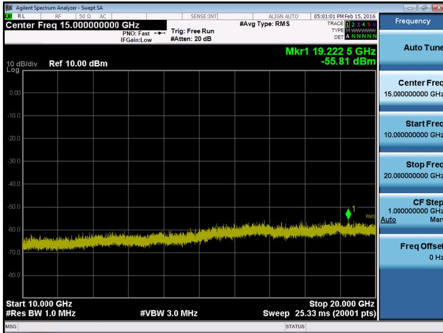
BAND 2. Conducted Spurious\_1 (18900ch\_5MHz\_QPSK\_RB 1\_0)
