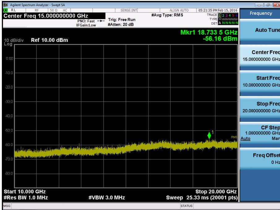
BAND 2. Conducted Spurious\_1 (18900ch\_15MHz\_QPSK\_RB 1\_0)
