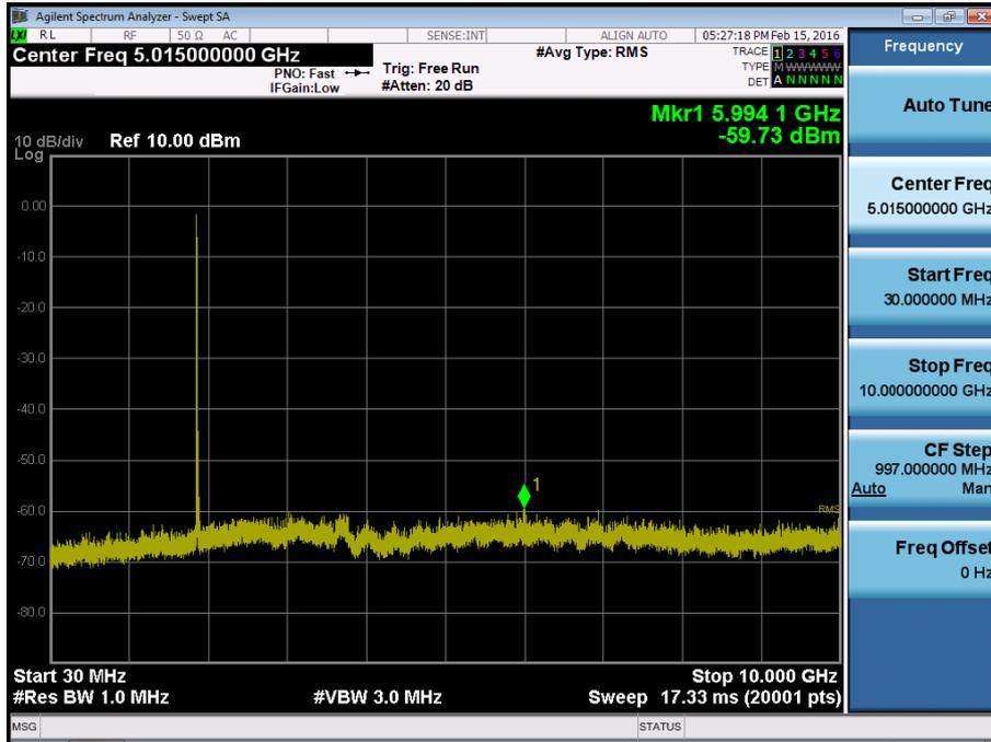
BAND 2. Conducted Spurious\_2 (18900ch\_20MHz\_QPSK\_RB 1\_0)
