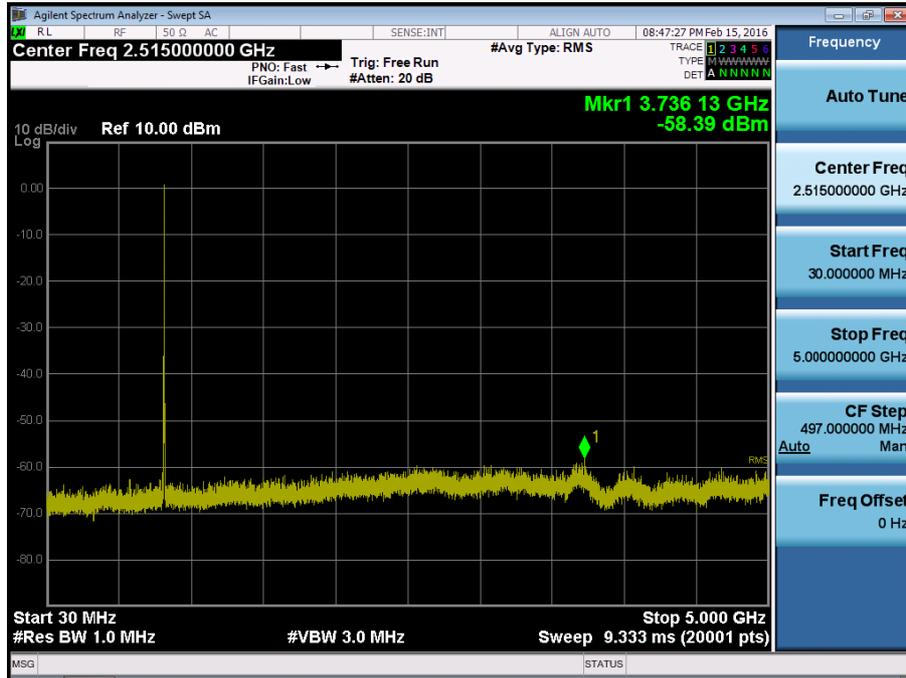
BAND 5. Conducted Spurious Plot \_2 (20525ch\_5MHz\_QPSK\_RB 1\_0)
