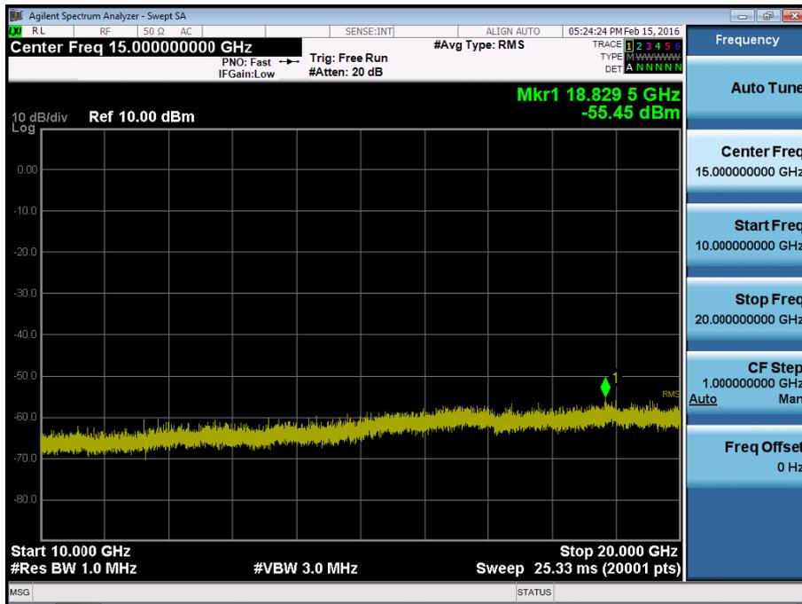
BAND 2. Conducted Spurious\_1 (18700ch\_20MHz\_QPSK\_RB 1\_0)
