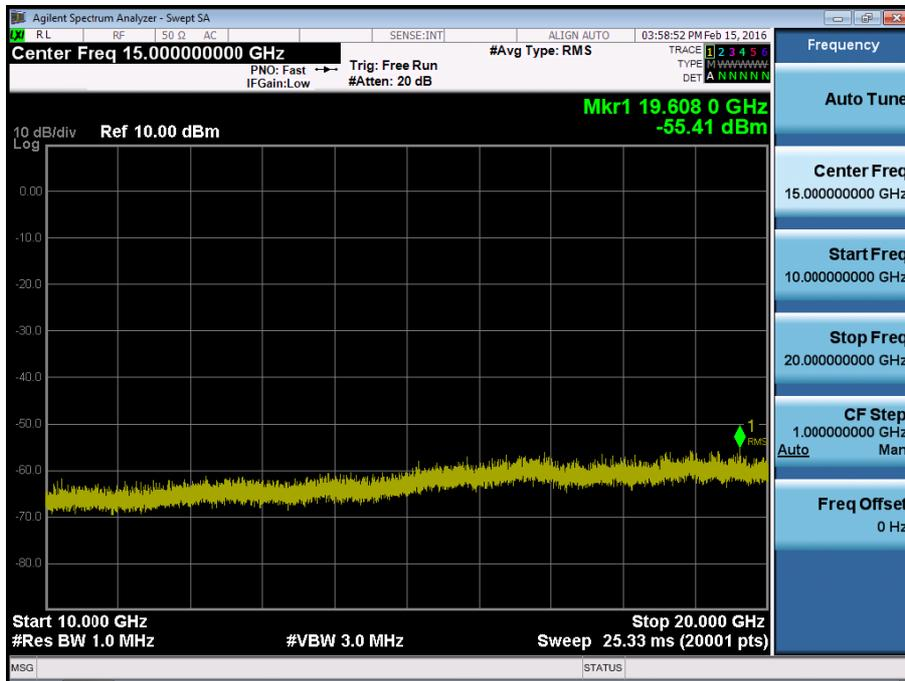
BAND 2. Conducted Spurious\_1 (18900ch\_1.4MHz\_QPSK\_RB 1\_0)
