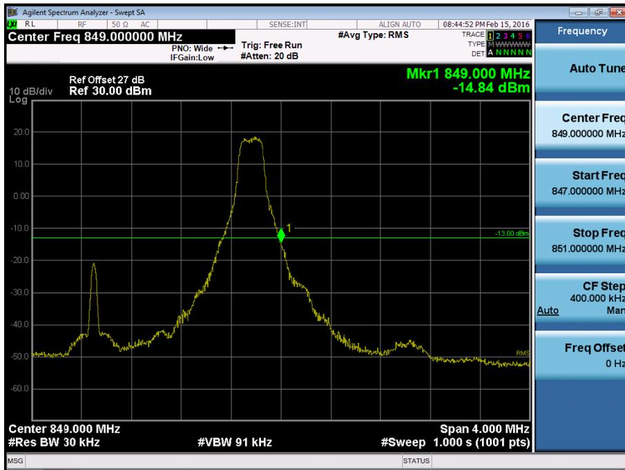
BAND 5. Upper Band Edge Plot (3M BW Ch.20635 QPSK\_RB15\_Offset 0)
