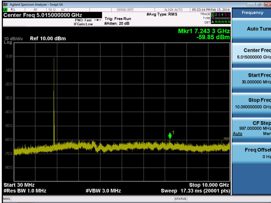
BAND 2. Conducted Spurious\_2 (18900ch\_15MHz\_QPSK\_RB 1\_0)
