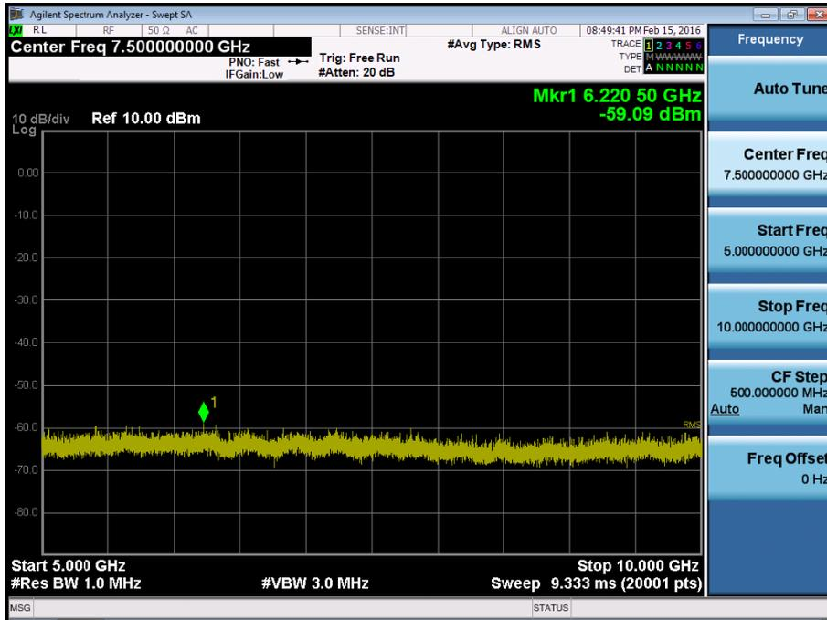
BAND 5. Conducted Spurious Plot \_1 (20525ch\_10MHz\_QPSK\_RB 1\_0)
