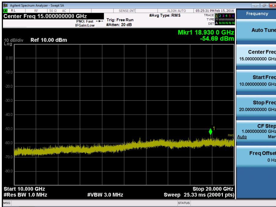
BAND 2. Conducted Spurious\_1 (18900ch\_20MHz\_QPSK\_RB 1\_0)
