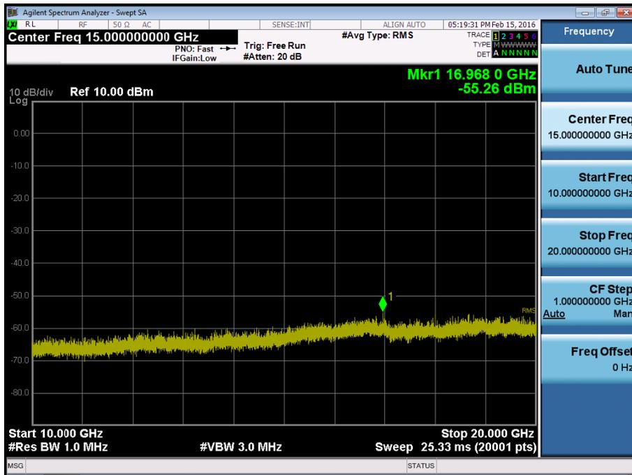
BAND 2. Conducted Spurious\_1 (19150ch\_10MHz\_QPSK\_RB 1\_0)
