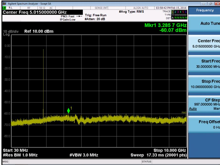
BAND 2. Conducted Spurious\_2 (18607ch\_1.4MHz\_QPSK\_RB 1\_0)
