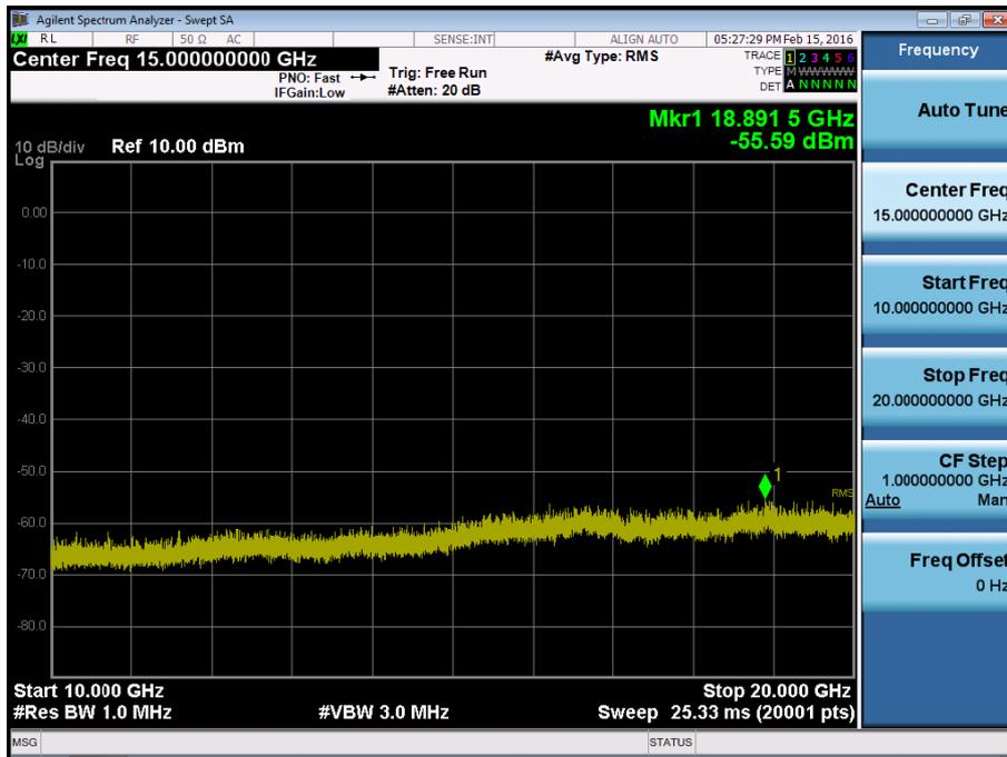
BAND 2. Conducted Spurious\_1 (19100ch\_20MHz\_QPSK\_RB 1\_0)
