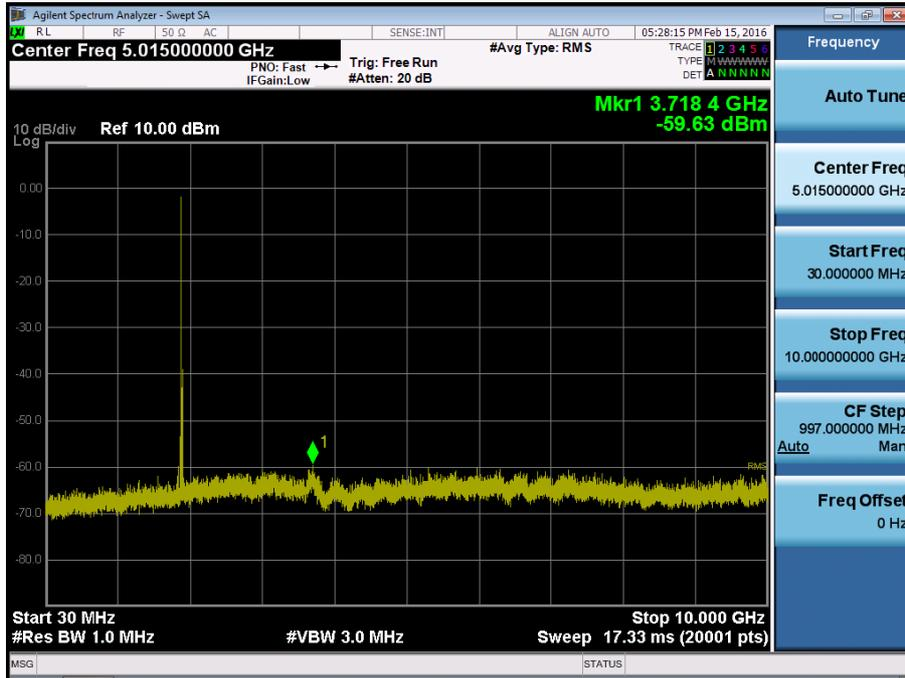
BAND 2. Conducted Spurious\_2 (19100ch\_20MHz\_QPSK\_RB 1\_0)
