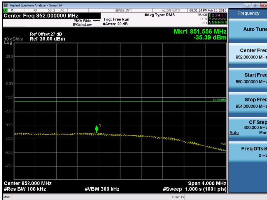
BAND 2. Conducted Spurious\_1 (18607ch\_1.4MHz\_QPSK\_RB 1\_0)
