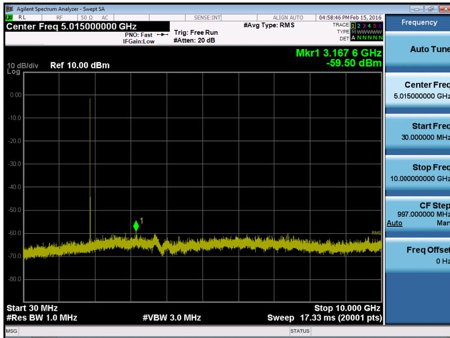
BAND 2. Conducted Spurious\_2 (18900ch\_3MHz\_QPSK\_RB 1\_0)
