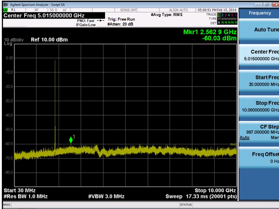
BAND 2. Conducted Spurious\_2 (18625ch\_5MHz\_QPSK\_RB 1\_0)
