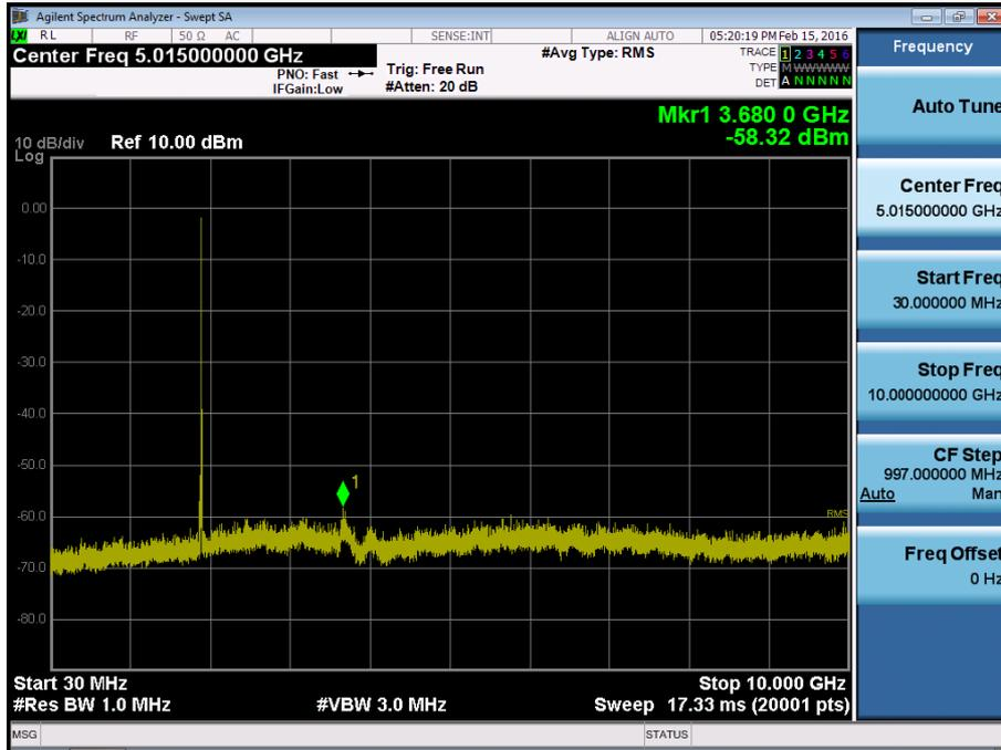
BAND 2. Conducted Spurious\_2 (19150ch\_10MHz\_QPSK\_RB 1\_0)
