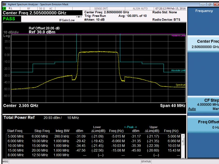
BAND7. Mid Channel Edge Plot (10MHz Ch.21100 QPSK RB 50)
