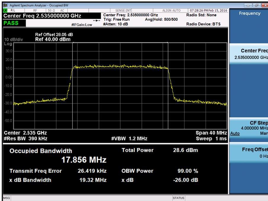
BAND7. Low Channel Edge Plot (5MHz Ch.20775 QPSK RB 25)
