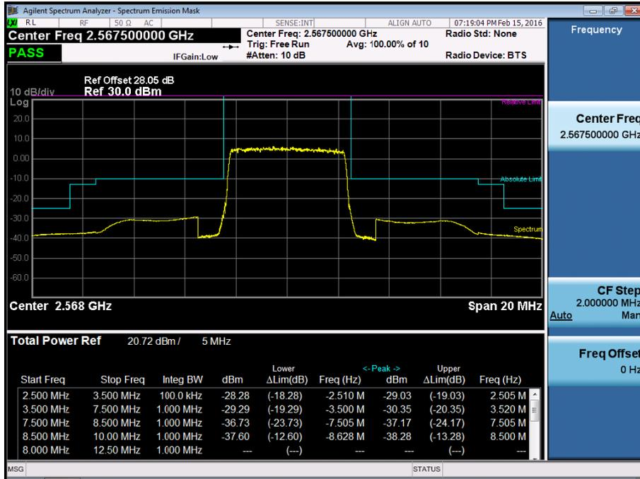
BAND7. Low Channel Edge Plot (10MHz Ch.20800 QPSK RB 50)
