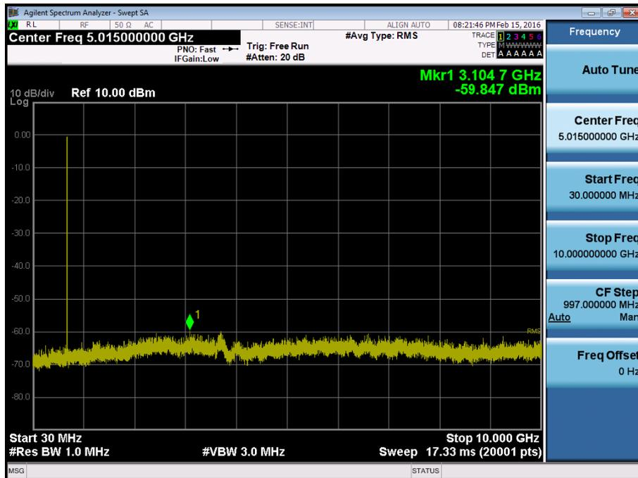
BAND 17. Conducted Spurious Plot\_ (23790ch\_10MHz\_QPSK\_RB 1\_0)
