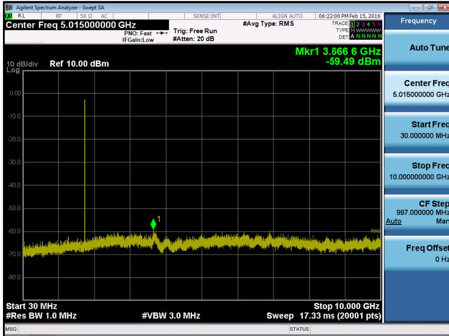
BAND 4. Conducted Spurious Plot\_2 (20375ch\_5MHz\_QPSK\_RB 1\_0)
