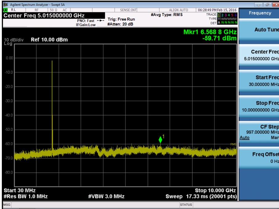
BAND 4. Conducted Spurious Plot\_2 (20175ch\_15MHz\_QPSK\_RB 1\_0)
