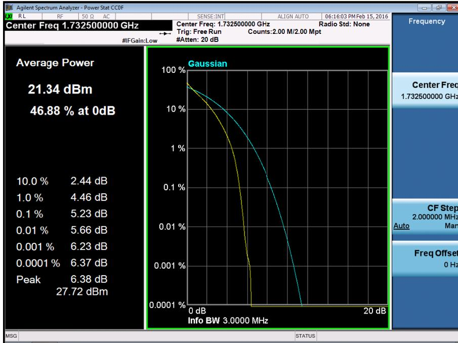
BAND 4. PAR Plot (3M BW\_Ch.20175\_16QAM\_RB15\_0)
