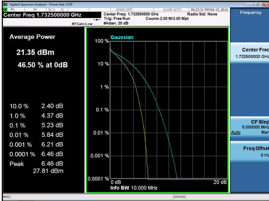
BAND 4. PAR Plot (10M BW\_Ch.20175\_16QAM\_RB50\_0)
