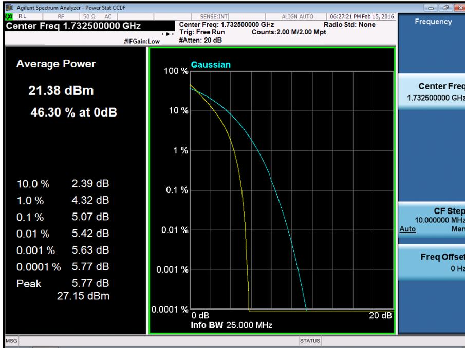
BAND 4. PAR Plot (15M BW\_Ch.20175\_16QAM\_RB75\_0)
