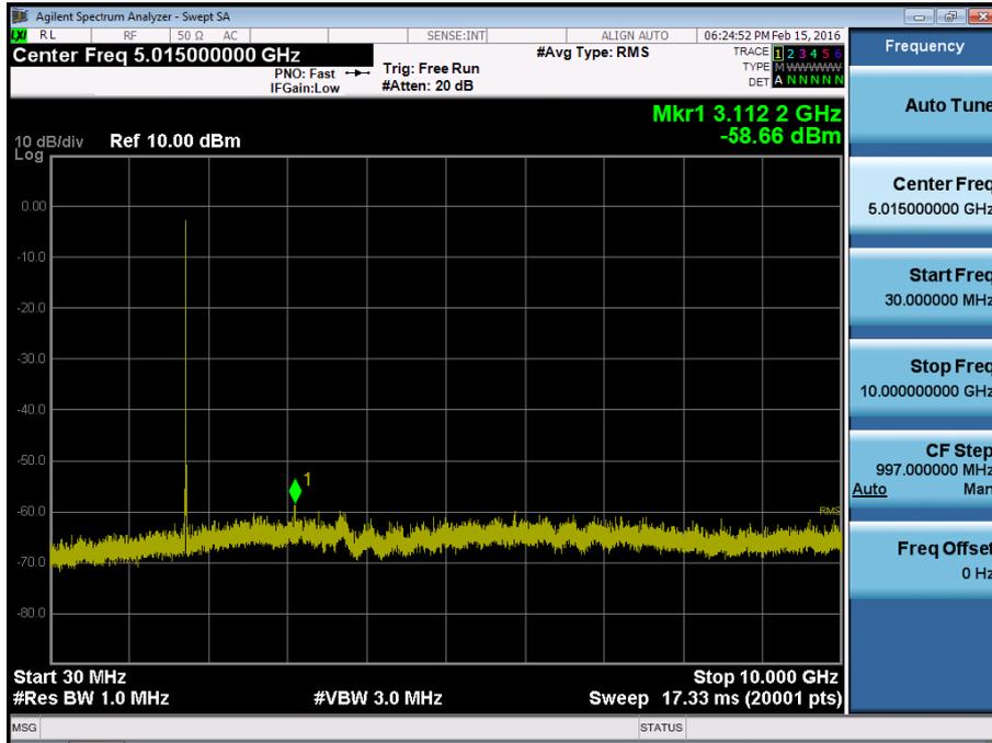
BAND 4. Conducted Spurious Plot\_2 (20175ch\_10MHz\_QPSK\_RB 1\_0)
