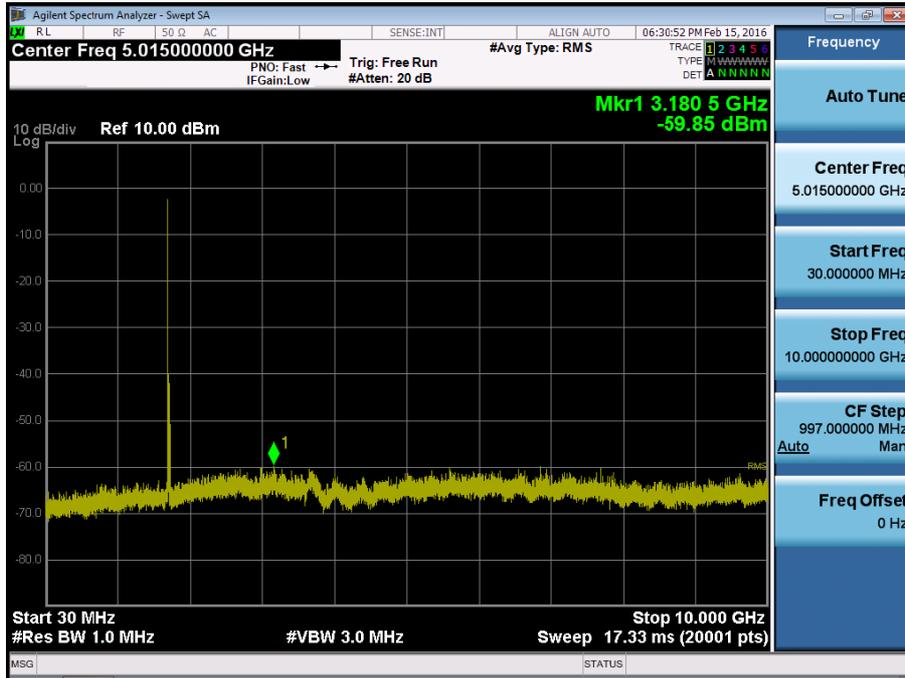
BAND 4. Conducted Spurious Plot\_2 (20050ch\_20MHz\_QPSK\_RB 1\_0)
