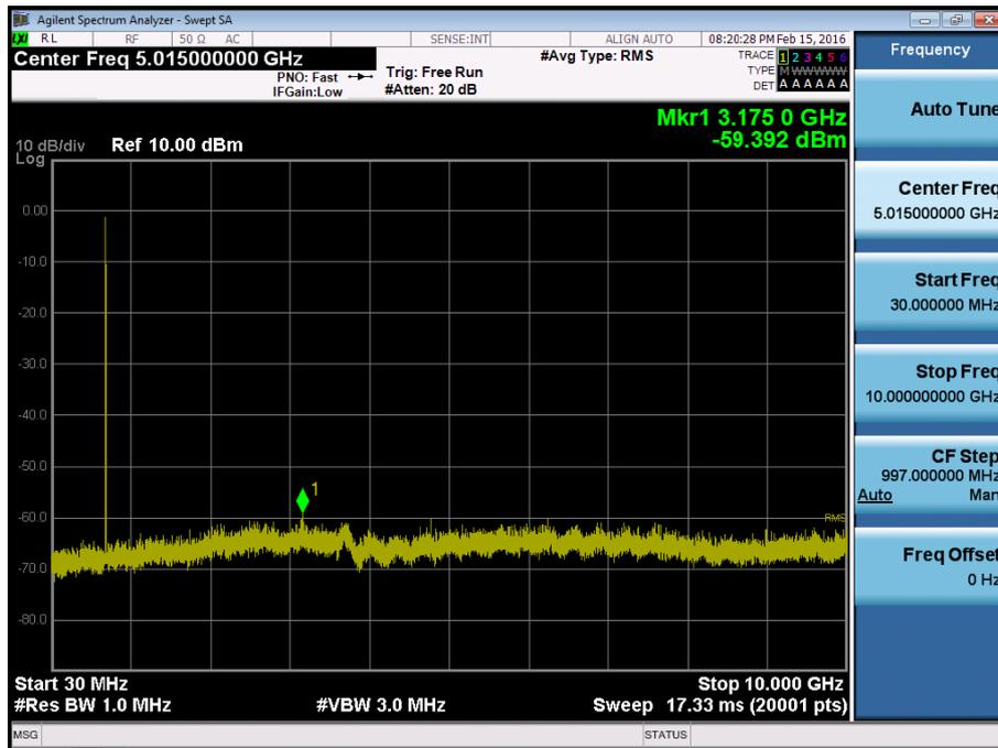
BAND 17. Conducted Spurious Plot\_ (23780ch\_10MHz\_QPSK\_RB 1\_0)
