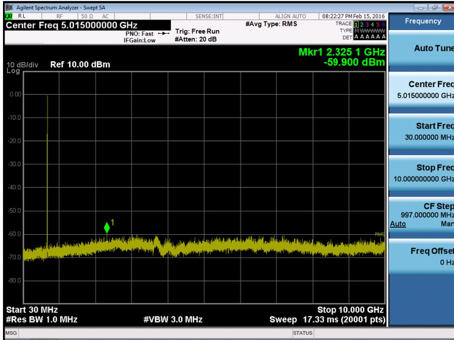
BAND 17. Conducted Spurious Plot\_ (23800ch\_10MHz\_QPSK\_RB 1\_0)
