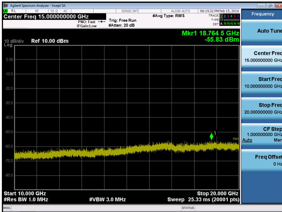
BAND 4. Conducted Spurious Plot\_1 (20175ch\_5MHz\_QPSK\_RB 1\_0)
