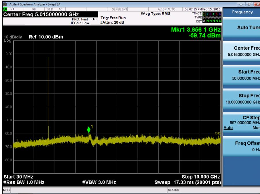
BAND 4. Conducted Spurious Plot\_2 (19957ch\_1.4MHz\_QPSK\_RB 1\_0)
