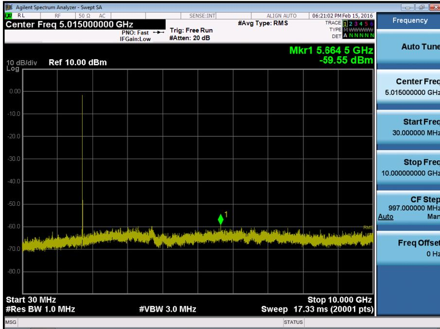
BAND 4. Conducted Spurious Plot\_2 (20175ch\_5MHz\_QPSK\_RB 1\_0)
