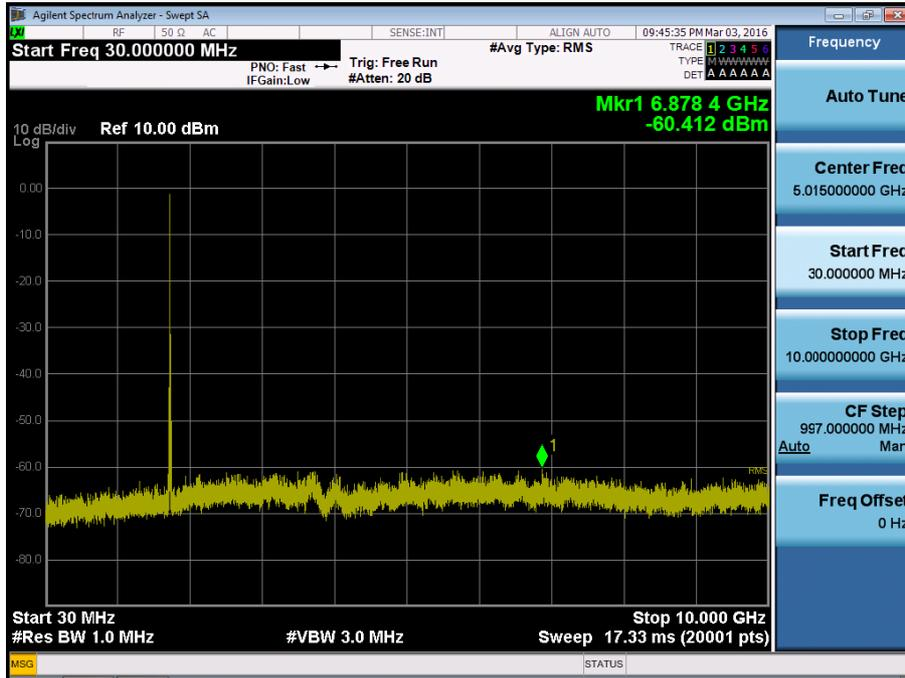
BAND 4. Conducted Spurious Plot\_2 (20325ch\_15MHz\_QPSK\_RB 1\_0)
