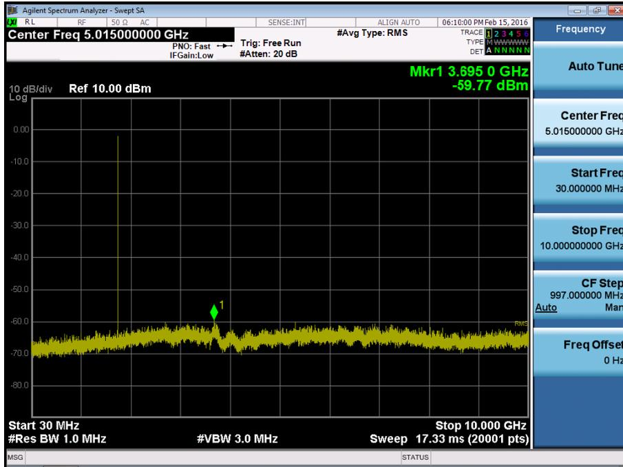
BAND 4. Conducted Spurious Plot\_2 (20393ch\_1.4MHz\_QPSK\_RB 1\_0)
