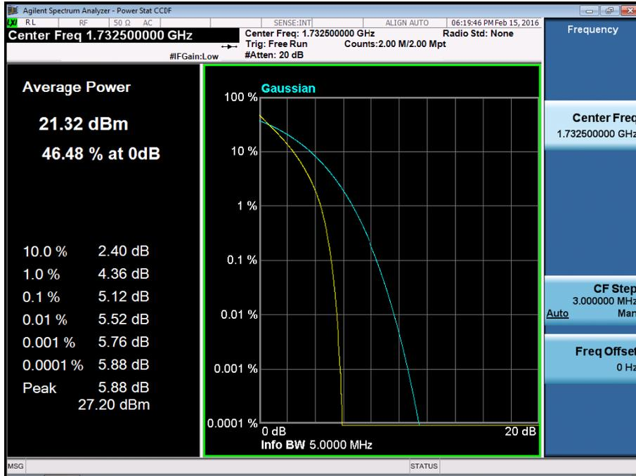
BAND 4. PAR Plot (5M BW\_Ch.20175\_16QAM\_RB25\_0)
