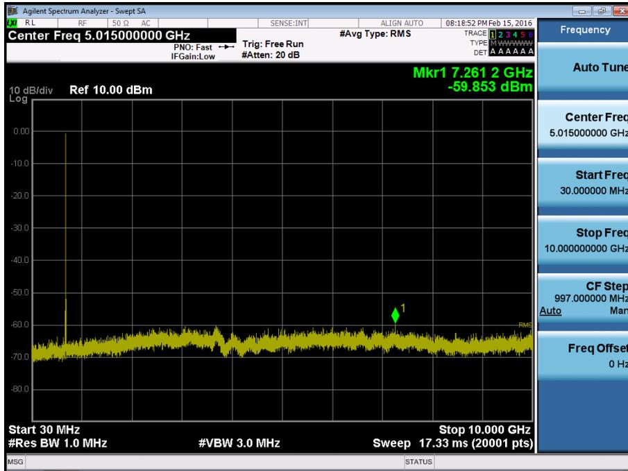
BAND 17. Conducted Spurious Plot\_ (23825ch\_5MHz\_QPSK\_RB 1\_0)
