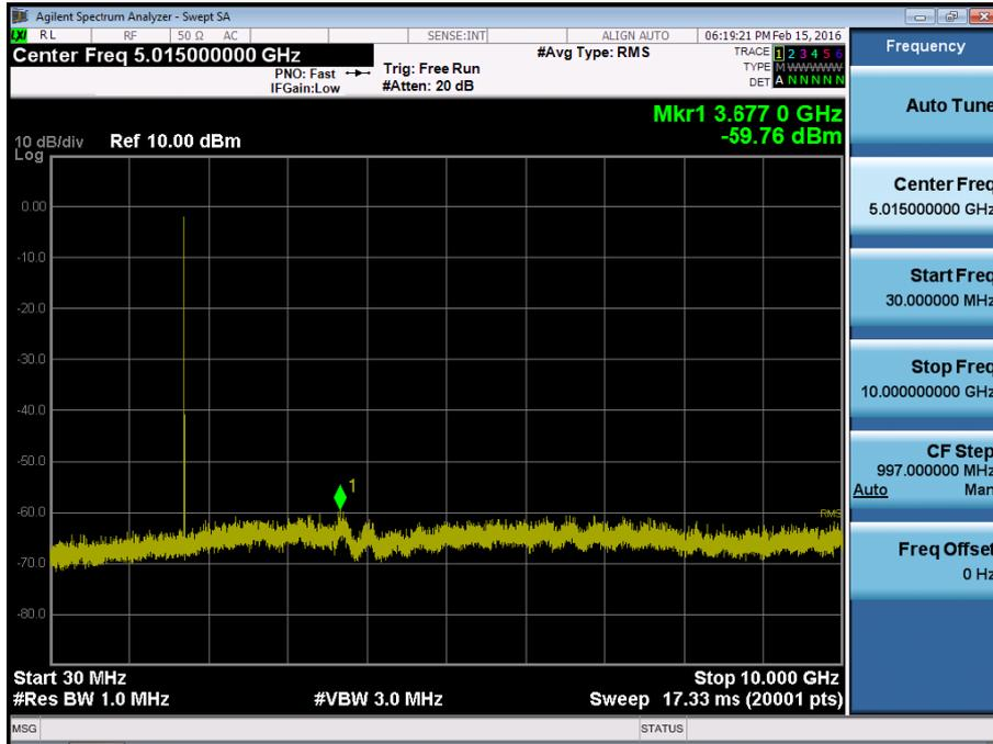
BAND 4. Conducted Spurious Plot\_2 (19975ch\_5MHz\_QPSK\_RB 1\_0)
