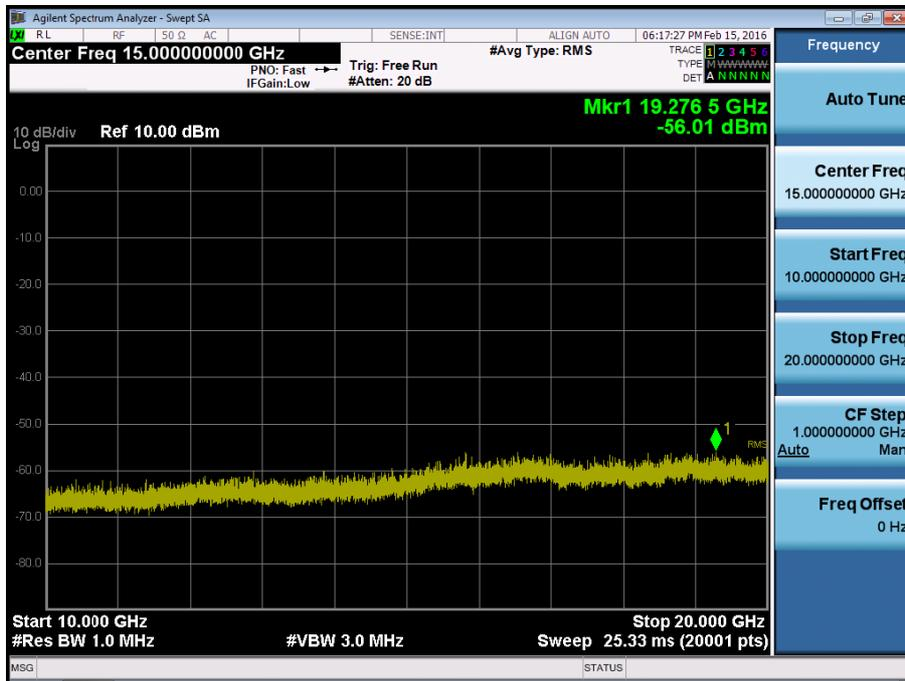
BAND 4. Conducted Spurious Plot\_1 (20385ch\_3MHz\_QPSK\_RB 1\_0)
