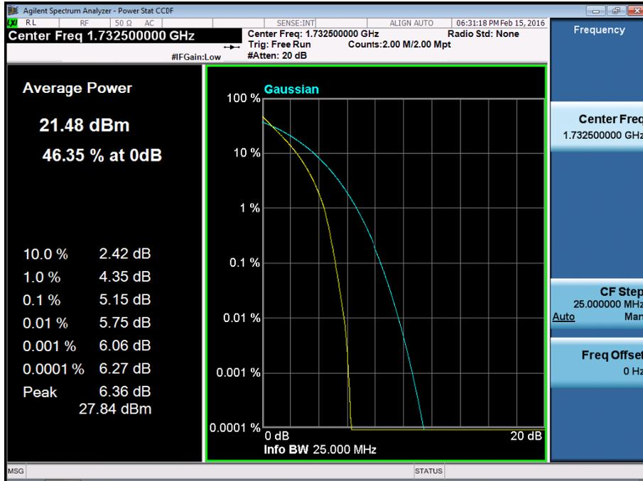
BAND 4. PAR Plot (20M BW\_Ch.20175\_16QAM\_RB100\_0)
