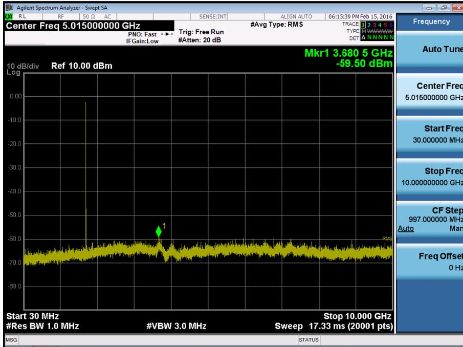
BAND 4. Conducted Spurious Plot\_2 (19965ch\_3MHz\_QPSK\_RB 1\_0)
