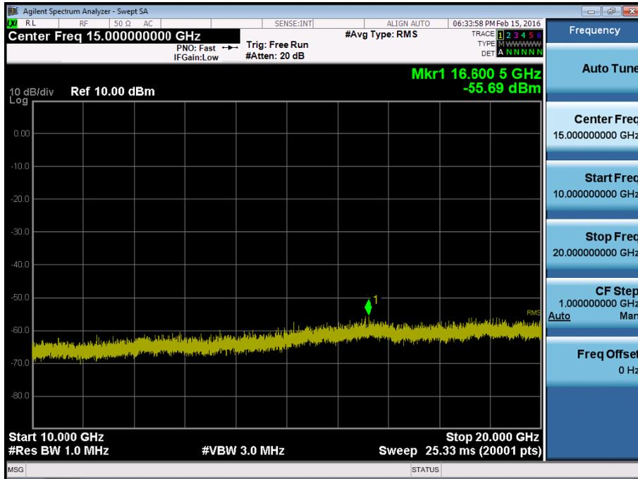
BAND 17. Conducted Spurious Plot\_ (23755ch\_5MHz\_QPSK\_RB 1\_0)
