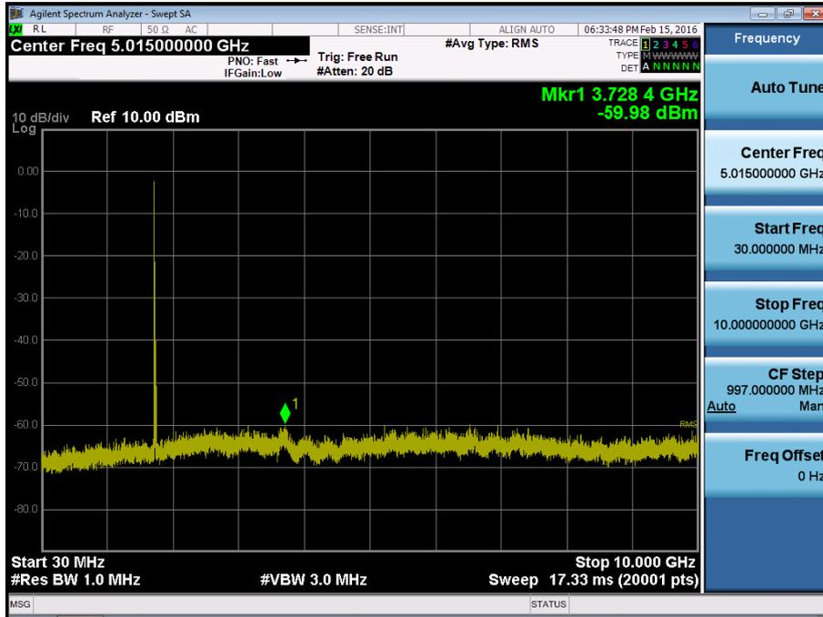
BAND 4. Conducted Spurious Plot\_2 (20300ch\_20MHz\_QPSK\_RB 1\_0)
