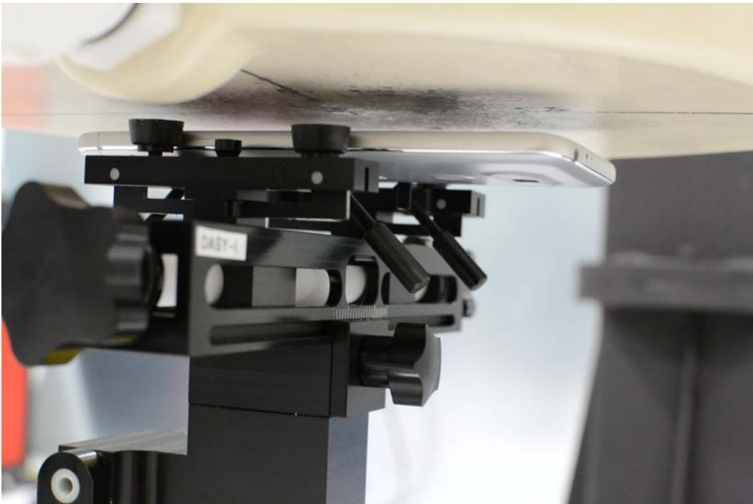
SAR Test Setup Photo 12: Front at 1.0 cm
