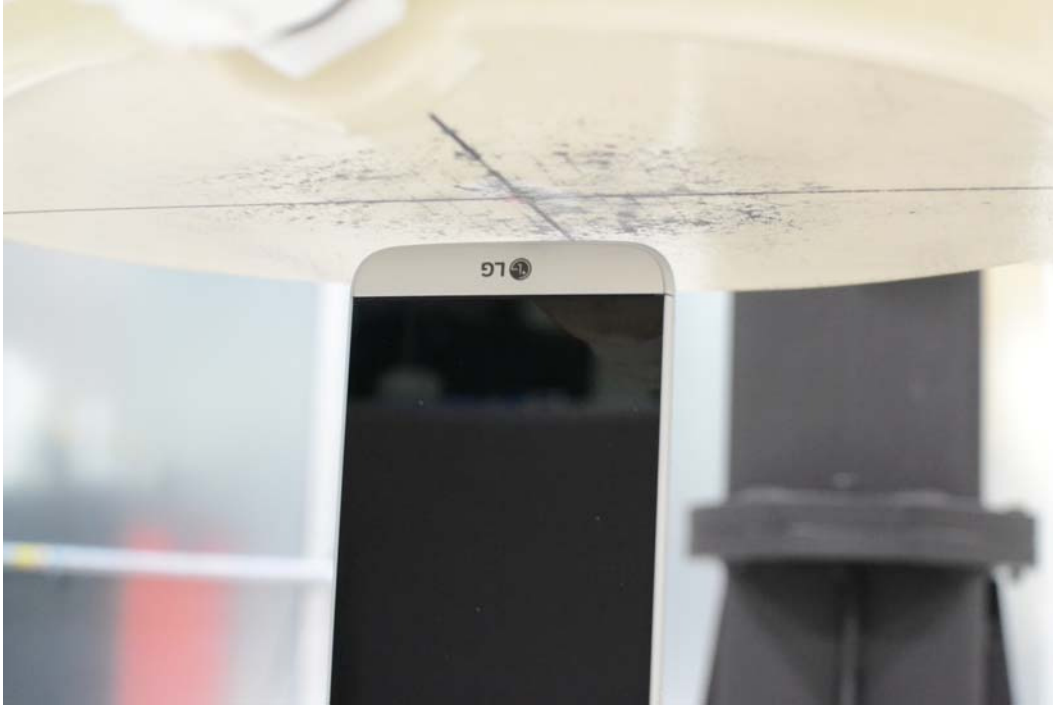
SAR Test Setup Photo 15: Bottom at 1.0 cm
