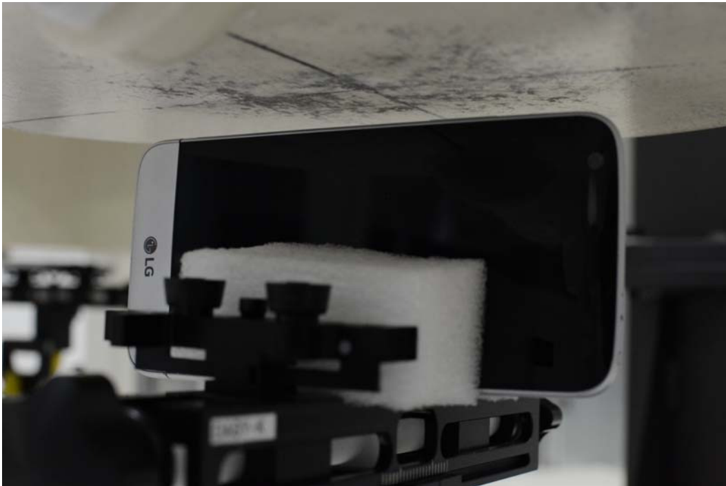
SAR Test Setup Photo 20: Left at 1.0 cm Camera Module Accessory
