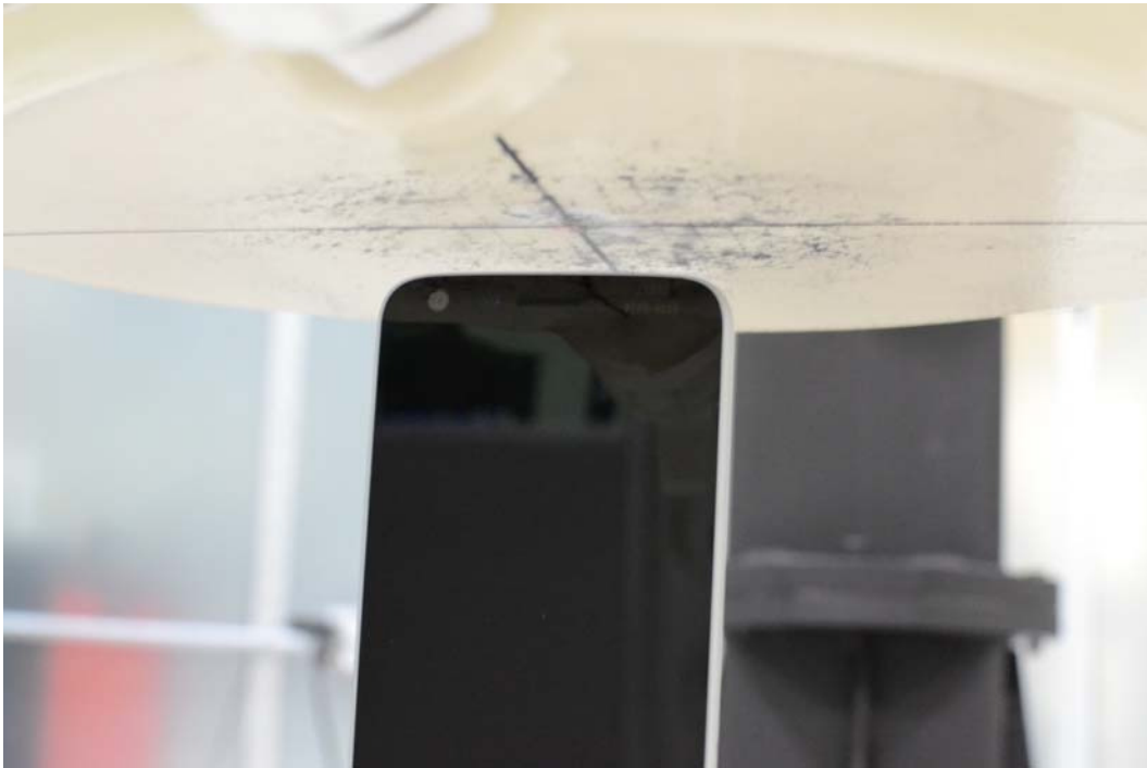
SAR Test Setup Photo 14: Top at 1.0 cm
