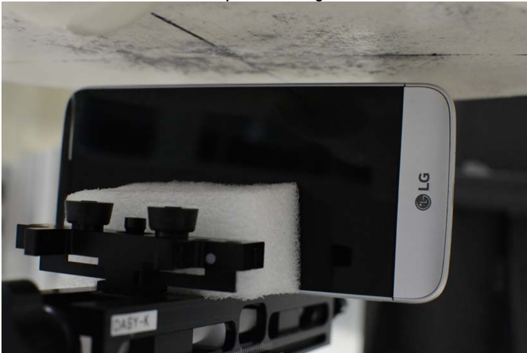
SAR Test Setup Photo 18: Right at 1.0 cm Camera Module Accessory
