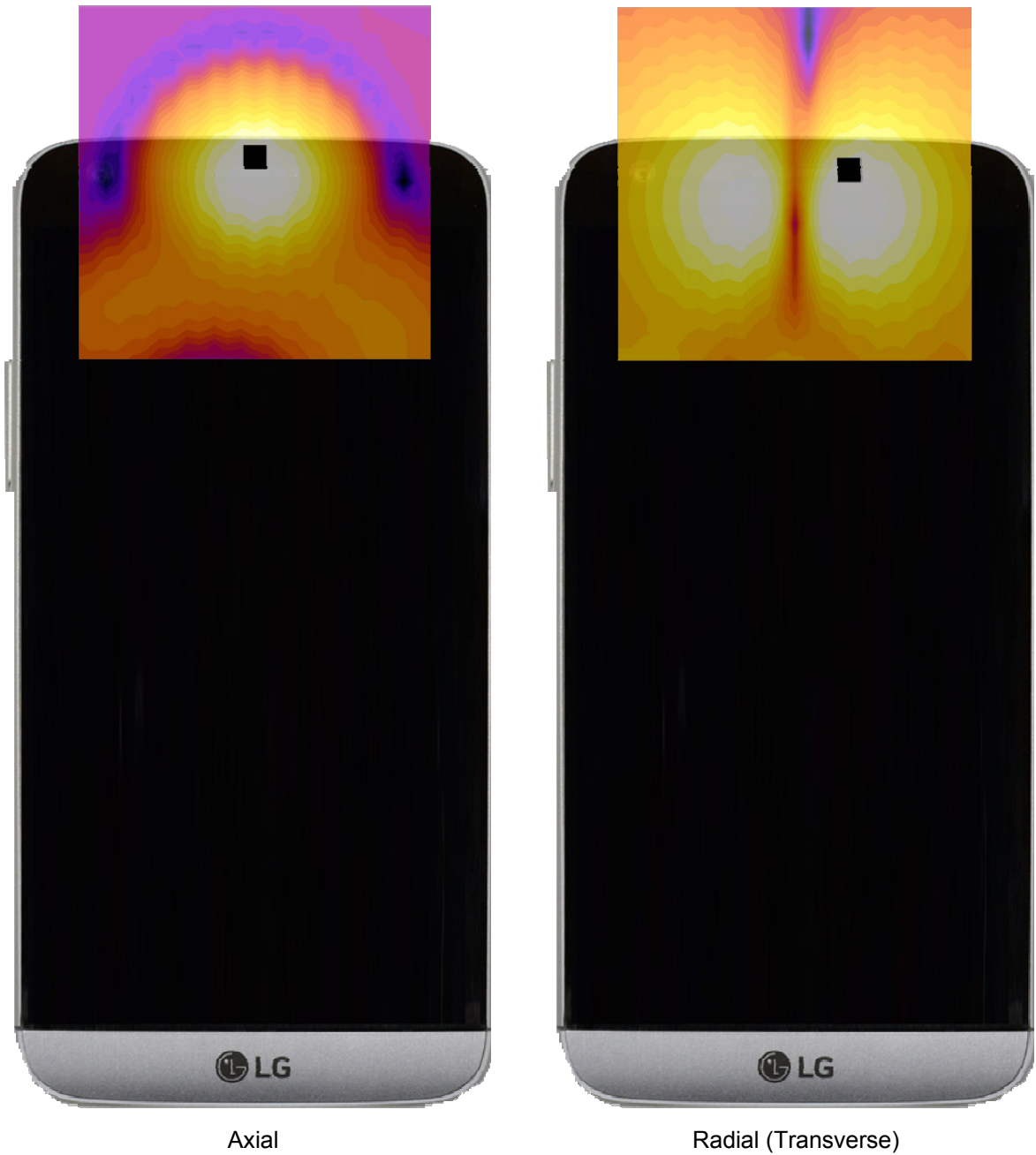
Figure 14-5 T-Coil Scan Overlay Magnetic Field Distributions
