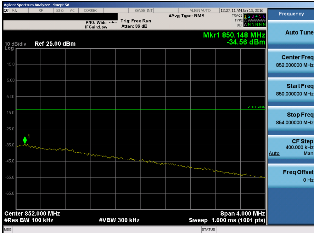
Plot 7-100. Upper Extended Band Edge Plot (Band 5 – Band 5 – 3.0MHz QPSK – RB Size 15)
