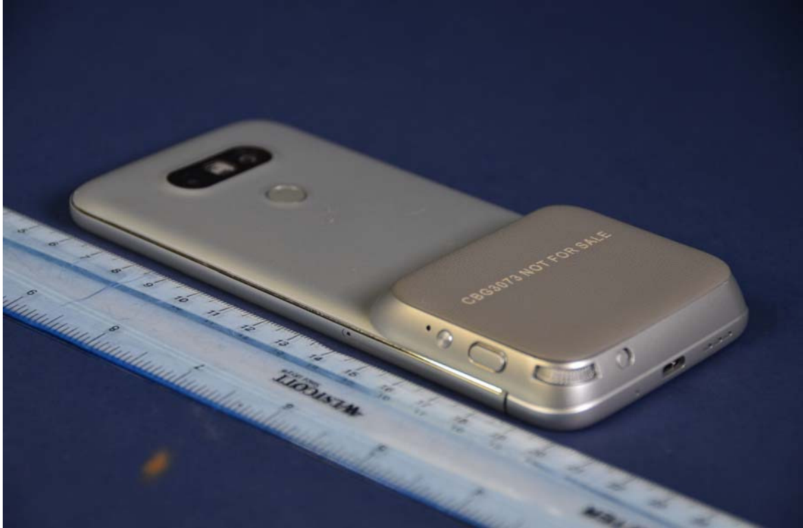
Camera Module Installed
