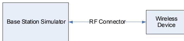
Figure 9-2 Power Measurement Setup
