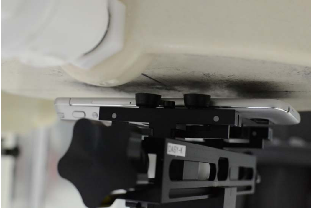
SAR Test Setup Photo 13: Front at 1.0 cm Camera Module Accessory
