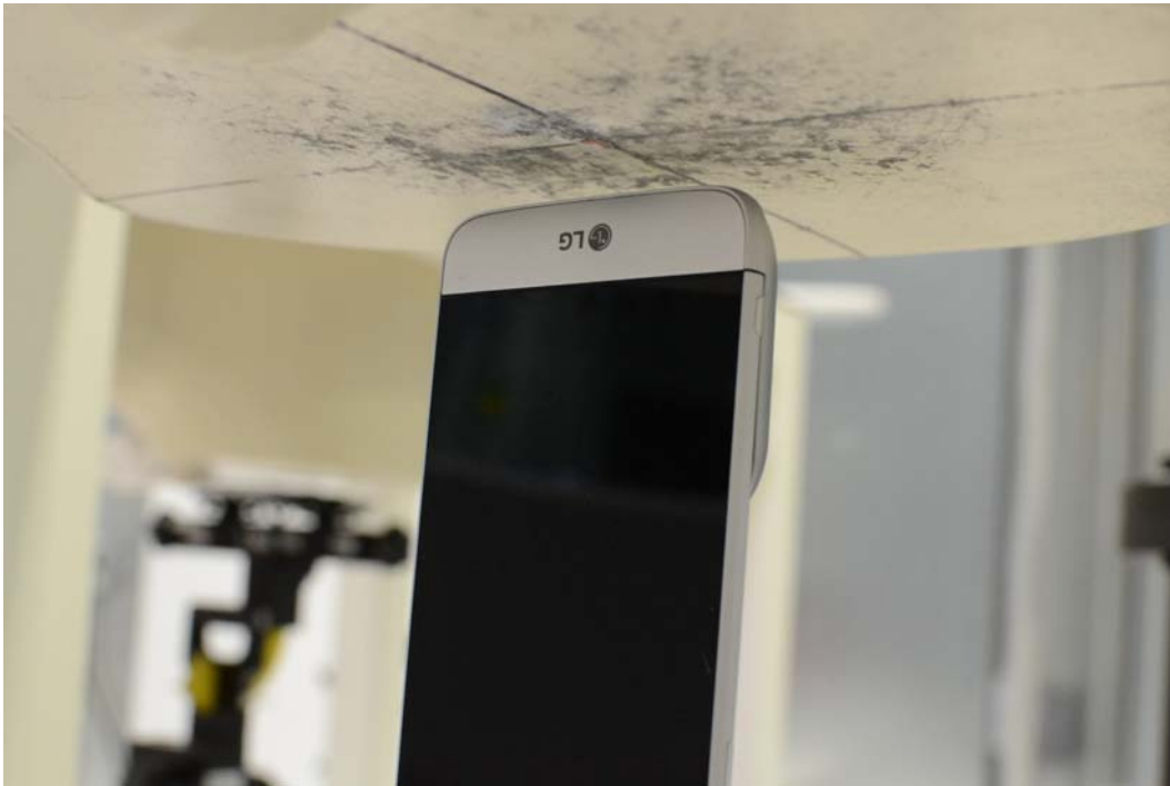
SAR Test Setup Photo 16: Bottom at 1.0 cm Camera Module Accessory
