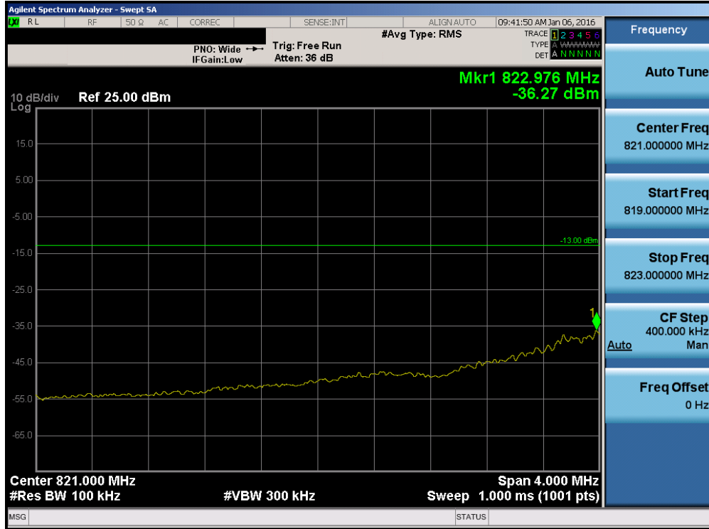
Plot 7-124. Lower Extended Band Edge Plot (Band 5 – 1.4MHz QPSK – RB Size 6)
