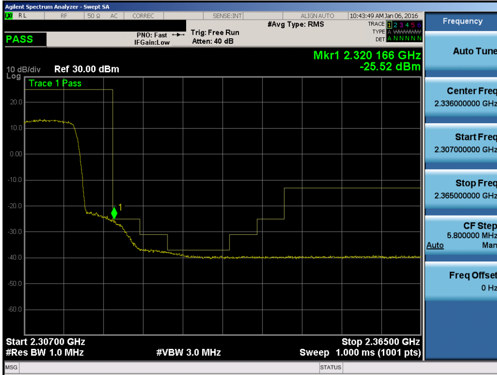
Plot 7-192. Upper Extended Band Edge Plot (Band 30 – 10.0MHz QPSK – RB Size 50)
