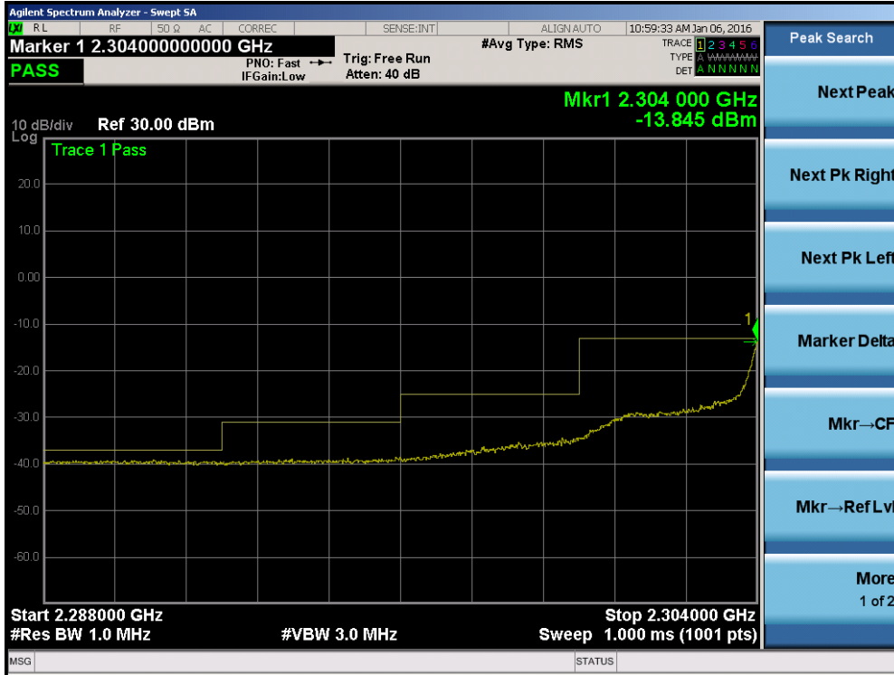
Plot 7-186. Lower Extended Band Edge Plot (Band 30 – 5.0MHz QPSK – RB Size 25)
