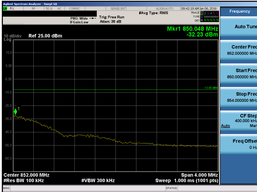
Plot 7-126. Upper Extended Band Edge Plot (Band 5 – 1.4MHz QPSK – RB Size 6)
