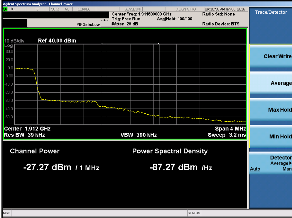
Plot 7-164. Upper Extended Band Edge Plot (Band 2 – 1.4MHz QPSK – RB Size 6)
