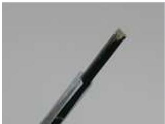
Figure 6. EX3DV4 E-field Probe
