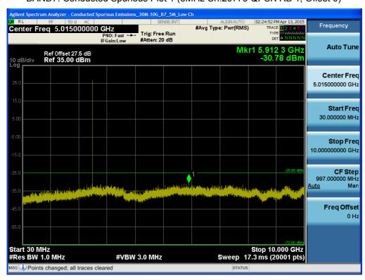
BAND7. Conducted Spurious Plot 2 (5MHz Ch.20775 QPSK RB 1, Offset 0)
