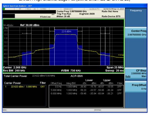
BAND7. Low Channel Edge Plot (10MHz Ch.20800 QPSK RB 50)
