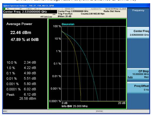
BAND7. Peak to Average Ratio Plot (15MHz Ch.21100 16-QAM RB 75)
