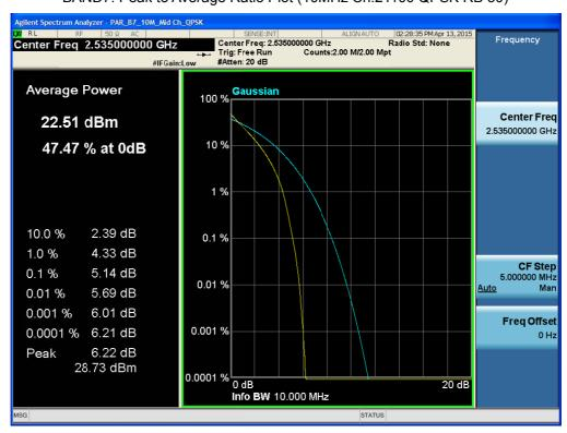
BAND7. Peak to Average Ratio Plot (10MHz Ch.21100 16-QAM RB 50)
