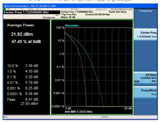
BAND 4. PAR Plot (5M BW\_Ch.20175\_16QAM\_RB25\_0)
