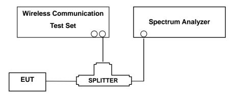
(Configuration of conducted Emission measurement)
