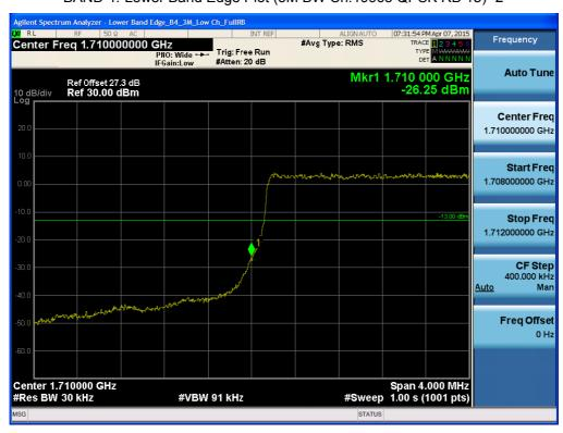
BAND 4. Lower Extended Band Edge Plot (3M BW Ch.19965 QPSK\_RB15\_0) -3
