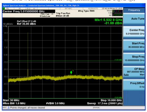
BAND 4. Conducted Spurious Plot\_2 (20325ch\_15MHz\_QPSK\_ RB 1\_0)
