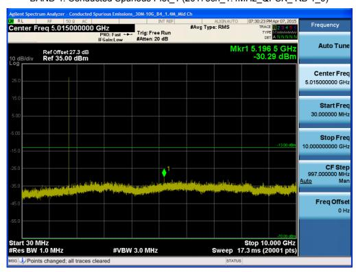
BAND 4. Conducted Spurious Plot\_2 (20175ch\_1.4MHz\_QPSK\_RB 1\_0)
