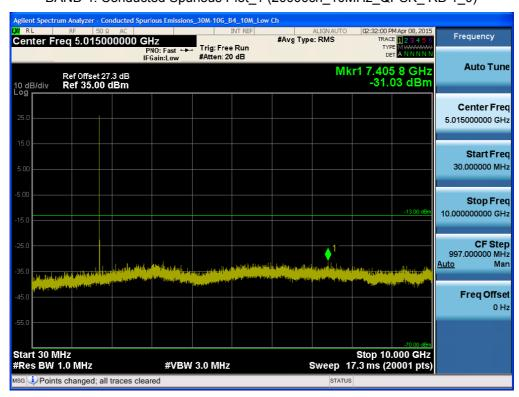
BAND 4. Conducted Spurious Plot\_2 (20000ch\_10MHz\_QPSK\_ RB 1\_0)
