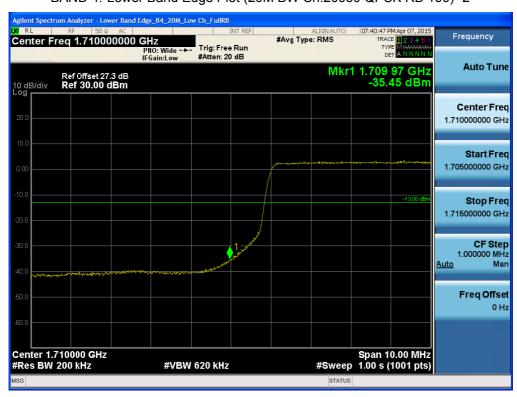
BAND 4. Lower Extended Band Edge Plot (20M BW Ch.20050 QPSK\_RB100\_0) -3
