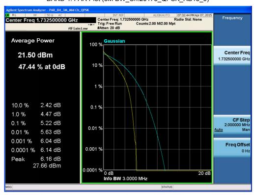
BAND 4. PAR Plot (3M BW\_Ch.20175\_16QAM\_RB15\_0)
