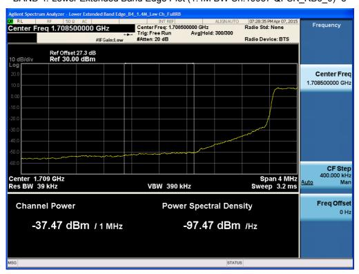
BAND 4. Lower Band Edge Plot (3M BW Ch.19965 QPSK RB 1, Offset 0) -1
