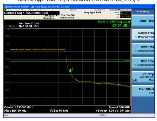
BAND 4. Upper Extended Band Edge Plot (3M BW Ch.20385 QPSK\_RB15\_0) -3
