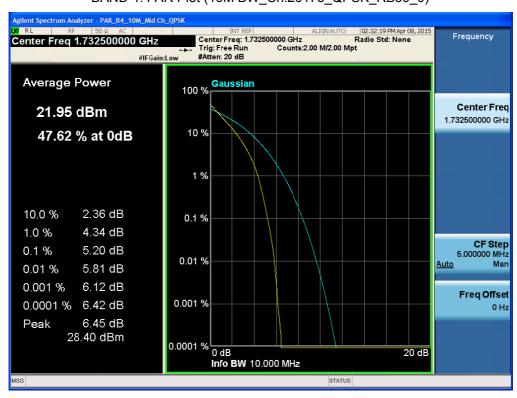
BAND 4. PAR Plot (10M BW\_Ch.20175\_16QAM\_RB50\_0)
