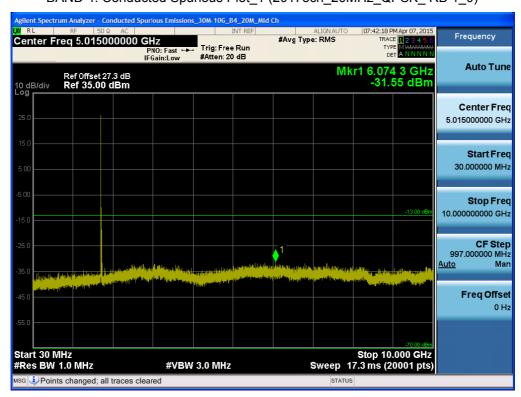
BAND 4. Conducted Spurious Plot\_2 (20175ch\_20MHz\_QPSK\_ RB 1\_0)
