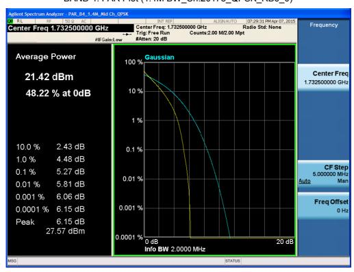
BAND 4. PAR Plot (1.4M BW\_Ch.20175\_16QAM\_RB6\_0)
