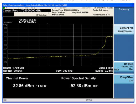
BAND 4. Lower Band Edge Plot (10M BW Ch.20000 QPSK RB 1, Offset 0) -1
