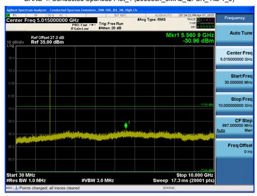
BAND 4. Conducted Spurious Plot\_2 (20385ch\_3MHz\_QPSK\_ RB 1\_0)
