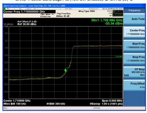
BAND 4. Lower Extended Band Edge Plot (10M BW Ch.20000 QPSK\_RB50\_0) -3
