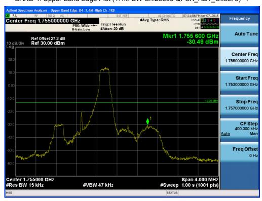
BAND 4. Upper Band Edge Plot (1.4M BW Ch.20393 QPSK\_RB6) -2
