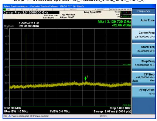
BAND 17. Conducted Spurious Plot\_2 (23825ch\_5MHz\_QPSK\_ RB 1\_0)
