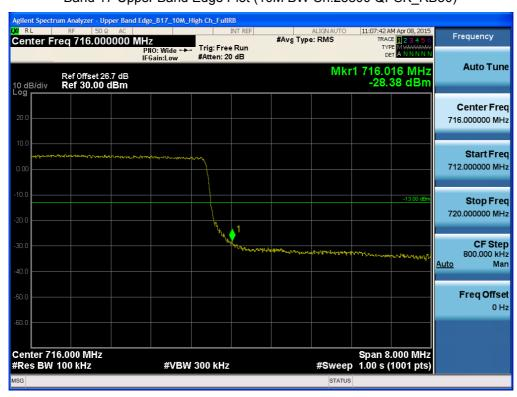
Band 17 Upper Extended Band Edge Plot (10M BW Ch.23800 QPSK\_RB50\_0)
