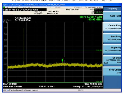
BAND 4. Conducted Spurious Plot\_2 (20175ch\_5MHz\_QPSK\_ RB 1\_0)
