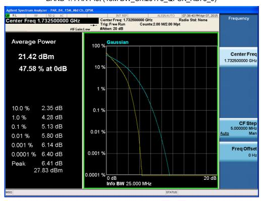
BAND 4. PAR Plot (15M BW\_Ch.20175\_16QAM\_RB75\_0)
