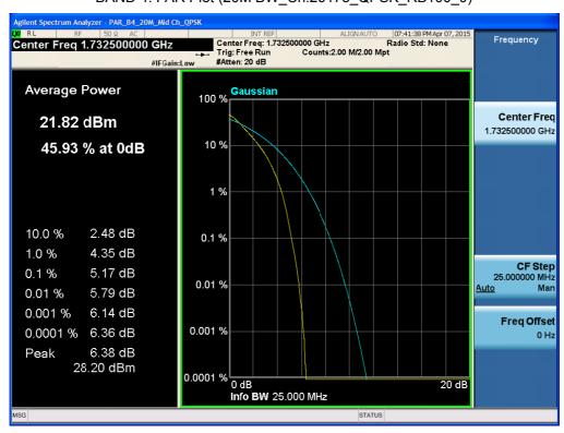
BAND 4. PAR Plot (20M BW\_Ch.20175\_16QAM\_RB100\_0)
