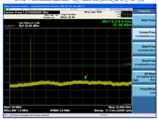
BAND 4. Conducted Spurious Plot\_2 (20375ch\_5MHz\_QPSK\_ RB 1\_0)
