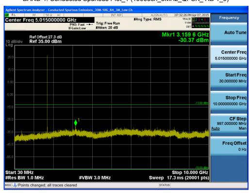
BAND 4. Conducted Spurious Plot\_2 (19965ch\_3MHz\_QPSK\_ RB 1\_0)
