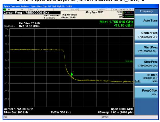
BAND 4. Upper Extended Band Edge Plot (10M BW Ch.20350 QPSK\_RB50) -3
