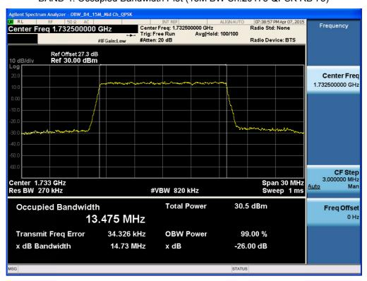
BAND 4. Occupied Bandwidth Plot (15M BW Ch.20175 16QAM RB 75)
