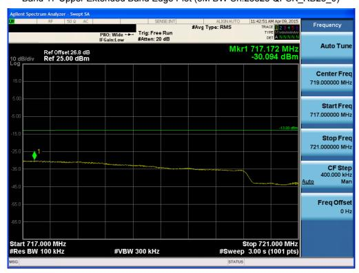
Band 17 Upper Band Edge Plot (10M BW Ch.23800 QPSK\_RB1\_Offset 49)
