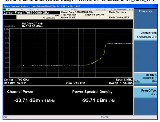
BAND 4. Lower Band Edge Plot (20M BW Ch.20050 QPSK RB 1, Offset 0) -1
