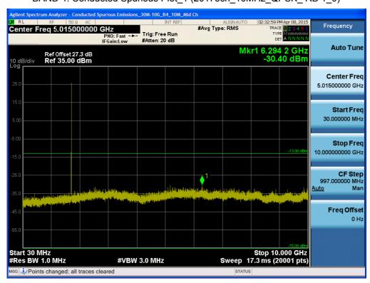
BAND 4. Conducted Spurious Plot\_2 (20175ch\_10MHz\_QPSK\_ RB 1\_0)
