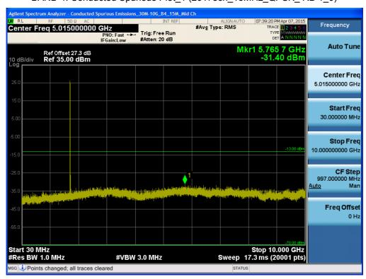
BAND 4. Conducted Spurious Plot\_2 (20175ch\_15MHz\_QPSK\_ RB 1\_0)
