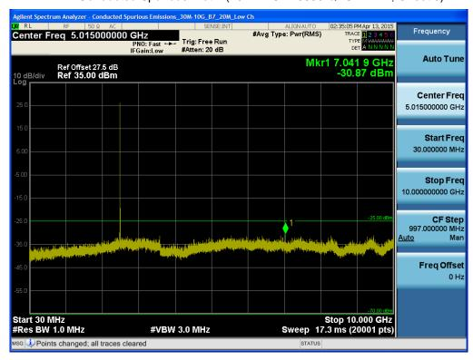
BAND7. Conducted Spurious Plot 2 (20MHz Ch.20850 QPSK RB 1, Offset 0)
