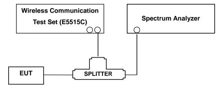
(Configuration of conducted Emission measurement)
