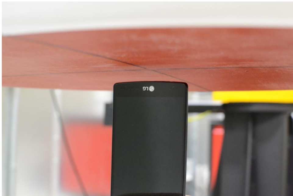
SAR Test Setup Photo 22: Bottom Edge, Standard Cover at 10 mm
