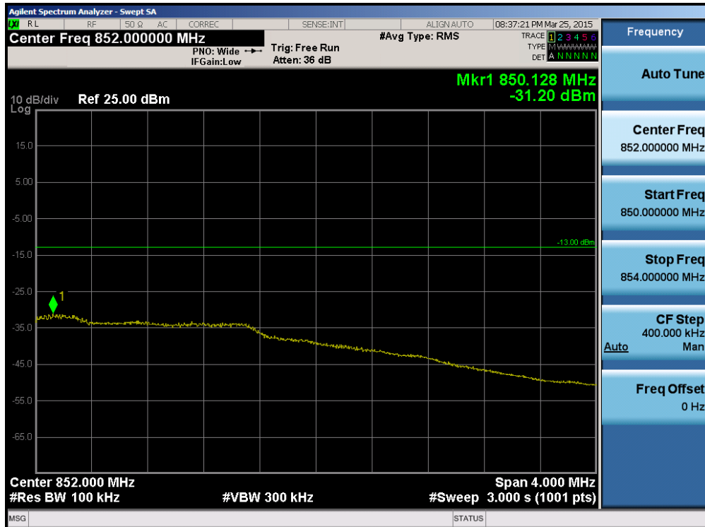
Plot 6-116. Upper Extended Band Edge Plot (Band 5 – Band 5 – 3.0MHz QPSK – RB Size 15)
