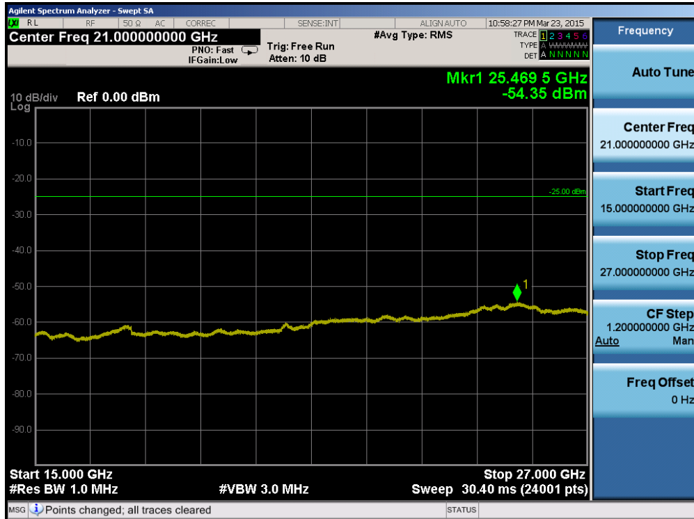
Plot 6-91. Conducted Spurious Plot (Band 7 – 20.0MHz QPSK – RB Size 1, RB Offset 0 – Mid Channel)
