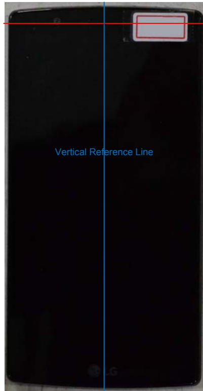
SAR Test Setup Photo 28: Horizontal and Vertical Reference Lines
