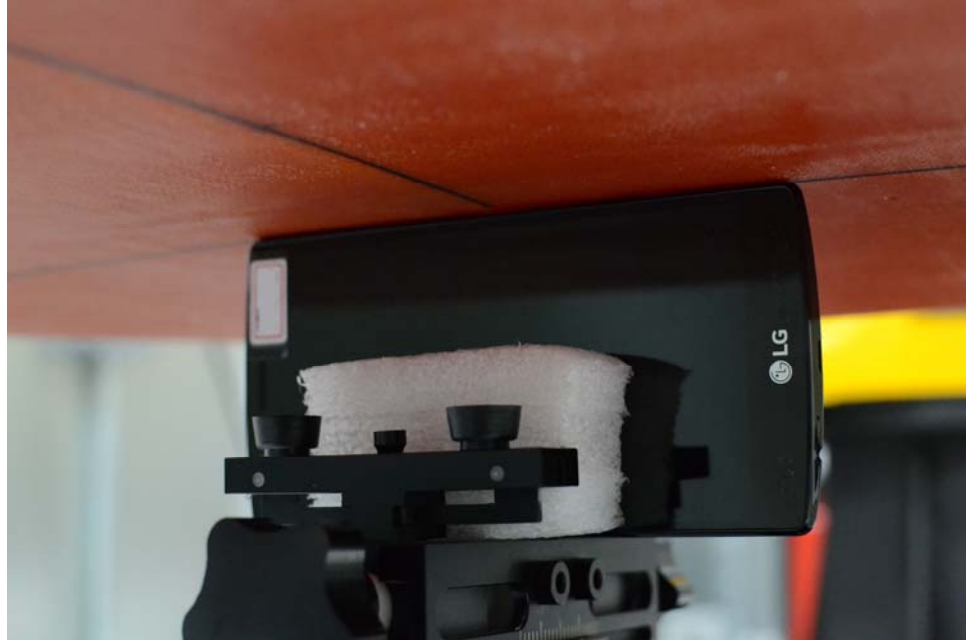
SAR Test Setup Photo 25: Right Edge, Standard Cover at 0 mm
