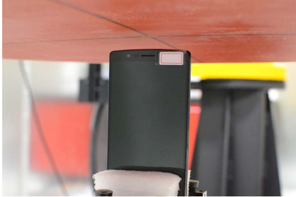
SAR Test Setup Photo 19: Top Edge, Standard Cover at 10 mm
