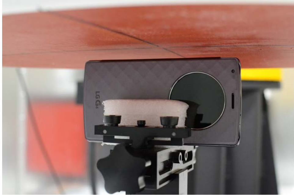
SAR Test Setup Photo 27: Left Edge, Quick Cover (Closed) at 10 mm
