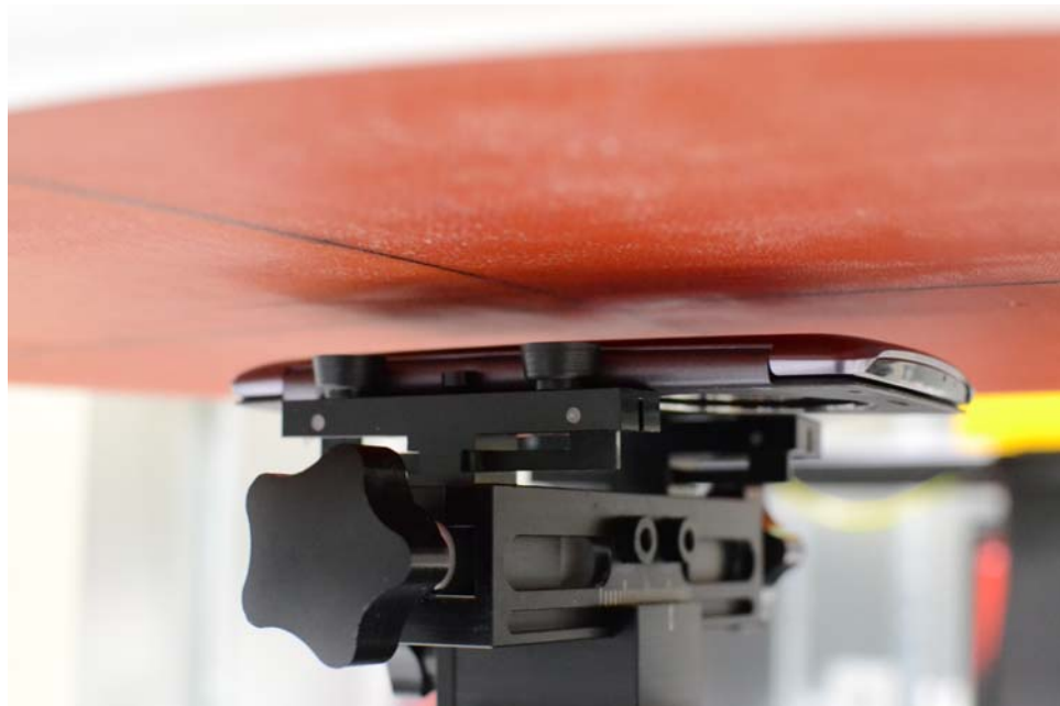
SAR Test Setup Photo 12: Back Side, Quick Cover (Closed) at 10 mm
