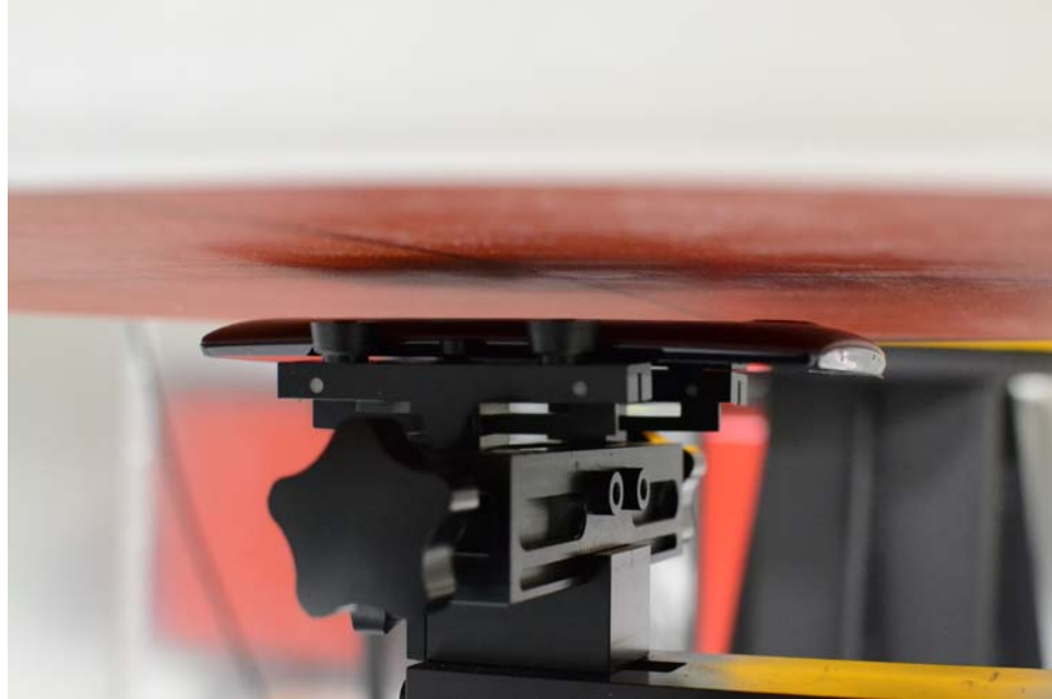
SAR Test Setup Photo 11: Back Side, Standard Cover at 10 mm
