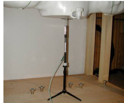
Figure 10-2 System Verification Setup Photo
