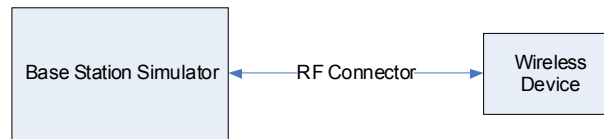
Figure 9-2 Power Measurement Setup
