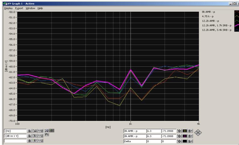
Figure 5-1 UMTS Audio Band Magnetic Noise
