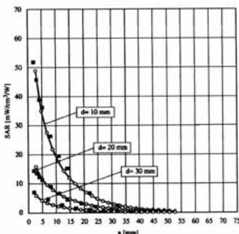
Figure 8. E-Field and temperature measurements at 1.8 GHz
