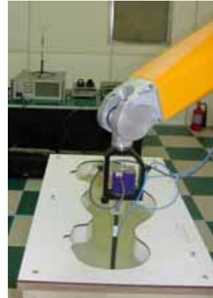
Figure 5. Photograph of the probe and the Phantom
