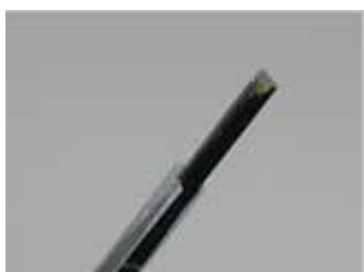
Figure 6. EX3DV4 E-field Probe
