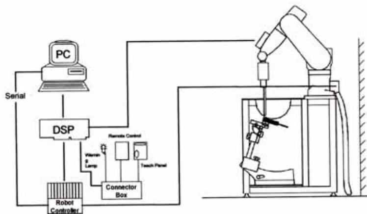
Figure 2. HCT SAR Lab. Test Measurement Set-up
