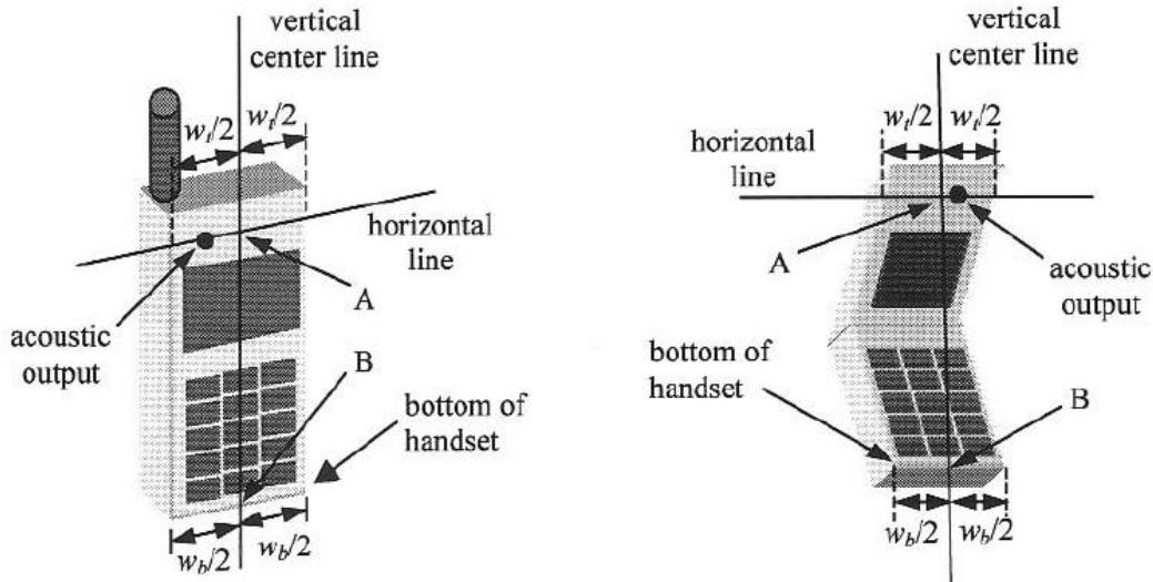
Figure 14. Handset vertical and horizontal reference lines
