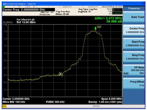
Test Plots without hopping ( $\pi$ /4DQPSK) Band Edges (High-CH)
