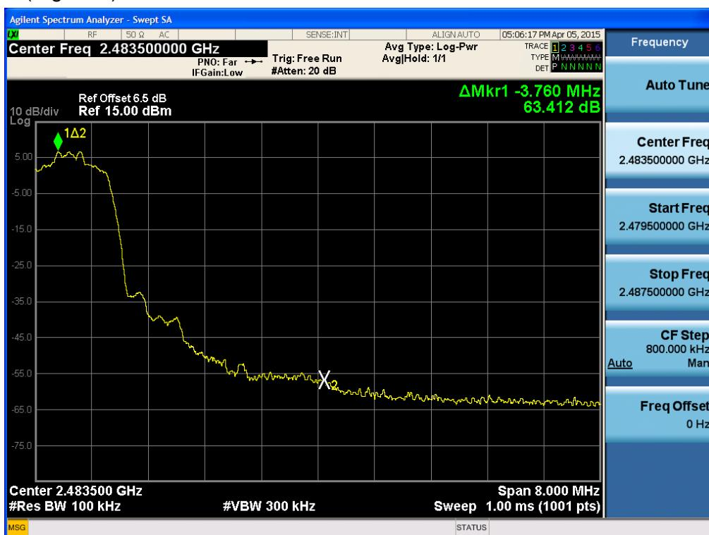
Test Plots with hopping (GFSK)
